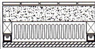
*Floor construction type: Timber: 19mm thick chipboard floor sheeting with timber joist, furring channel, insulation and two layers plaster ceiling*
