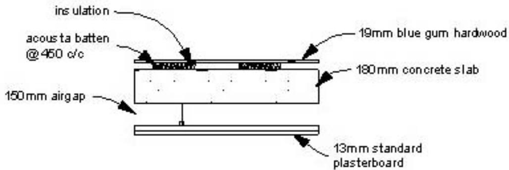
**FIGURE 29 – FLOOR DETAIL - TYPE D SYSTEM**
