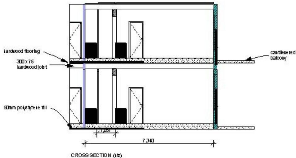
**FIGURE 22 - CROSS SECTION THROUGH STRUCTURE**
