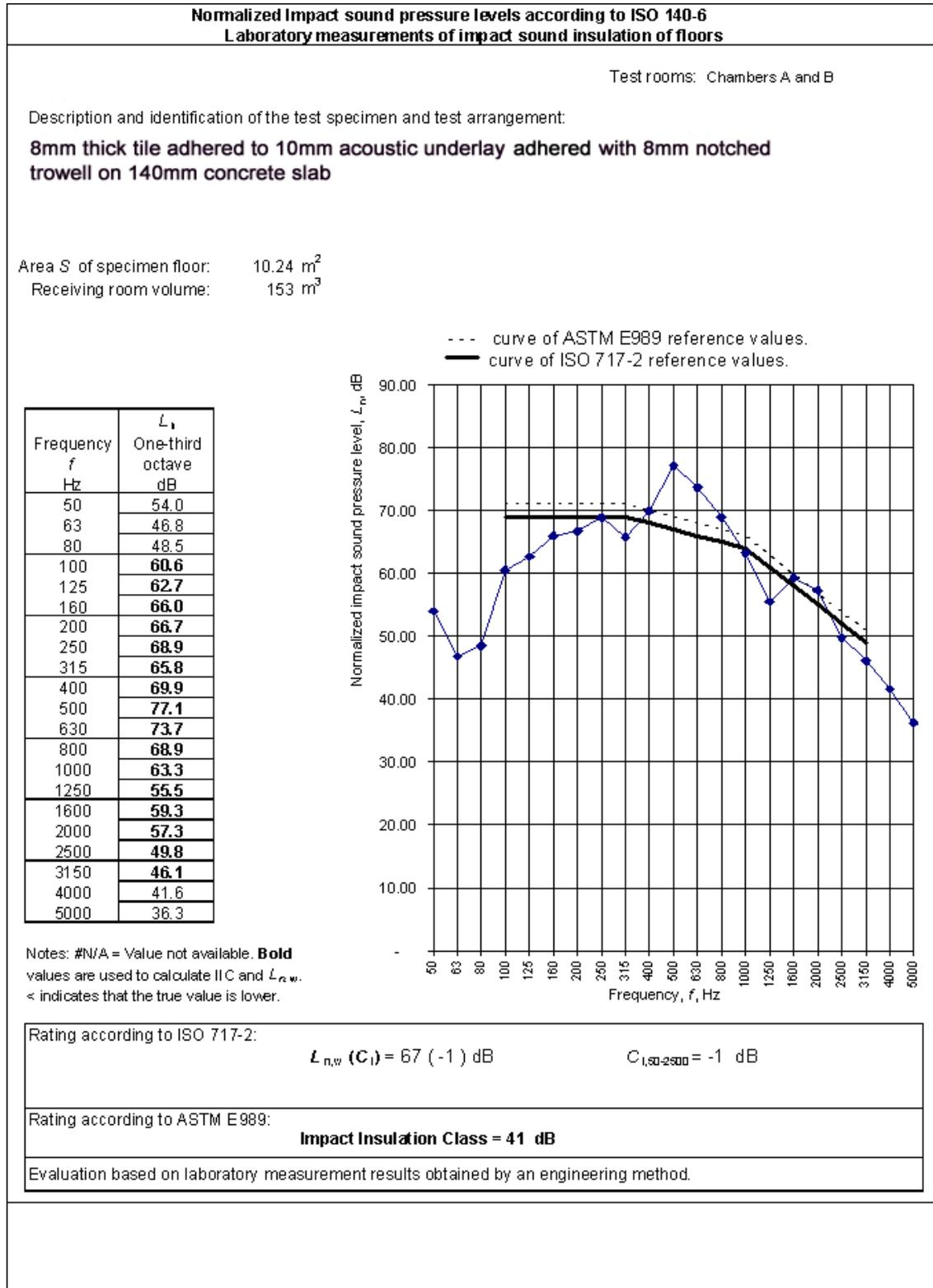
The example given for the laboratory measurements of impact sound insulation of floors, for the 8mm thick tile to 10mm acoustic underlay adhered with 8mm notched trowel on 140mm concrete slab, indicates the test results recorded in one-third octaves. The specimen floor area is identified and the volume of the receiving room recorded. The results are graphed in relation to the reference values and the rating is given in accordance with ISO 717-2.
