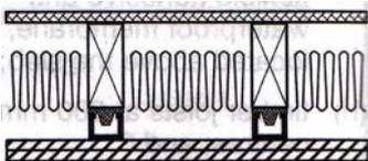
*Floor construction type: Timber: 19mm thick tongued and grooved boards, timber joist, two layers insulation and single plaster ceiling*
