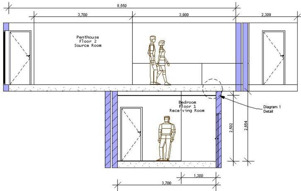
**FIGURE 13 – CROSS SECTION THROUGH FLOORS 1 & 2**
