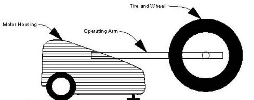
**FIGURE 8 - SKETCH OF THE RION BANG MACHINE** (not to scale)
