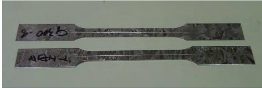
(b) Tension test coupons
