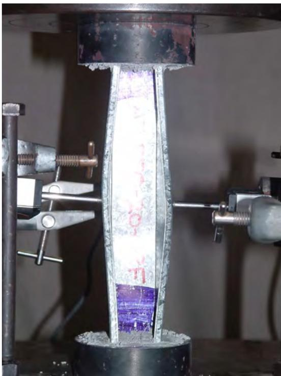
(a) Distortional buckling failure of Type A specimen
