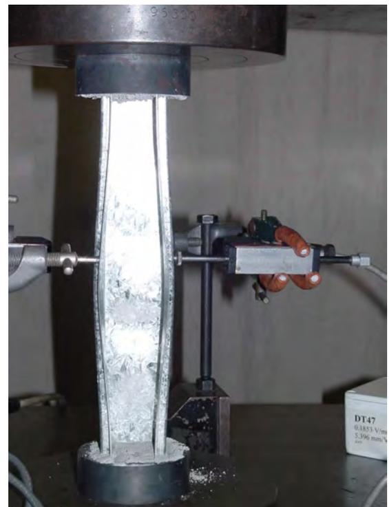
(b) Distortional buckling failure of Type B specimen
