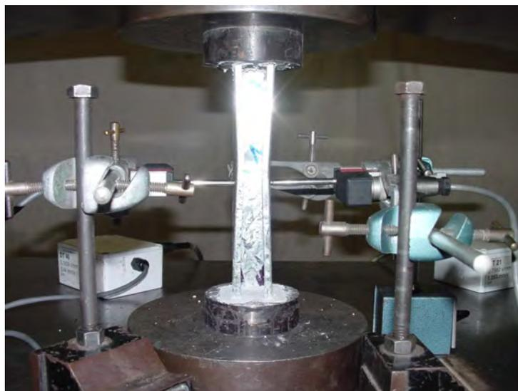
**Figure 4.9 Distortional Buckling Failure Mode Observed
