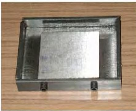
(a) End plate before inserting the specimen
