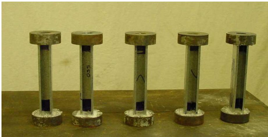
**Figure 4.11** Test Specimens with End Plates
