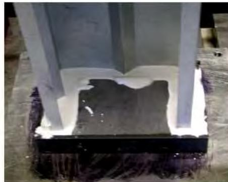
(b) Specimen on end plate filled with pattern-stone
