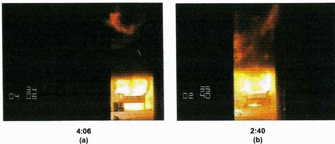
Figure 9.3– Burning armchair in ISO room at flashover: (a) plasterboard walls and ceiling; and (b) Lauan plywood walls and plasterboard ceiling
