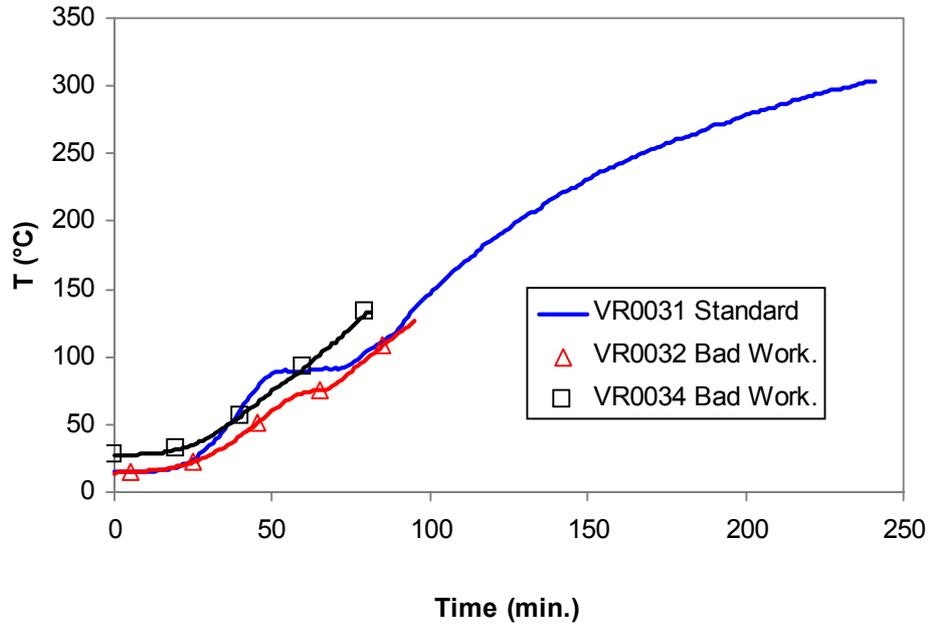
**Figure 5-3.** Average temperature on unexposed faces of masonry test walls. Standard furnace test.
