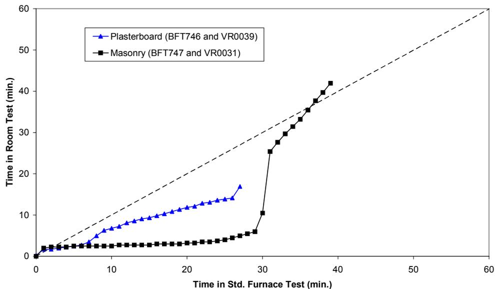
**Figure 7-4.** Time to reach the same change in unexposed-face temperature in standard furnace test and room test (using thermocouples  $U1-U5$ ).
