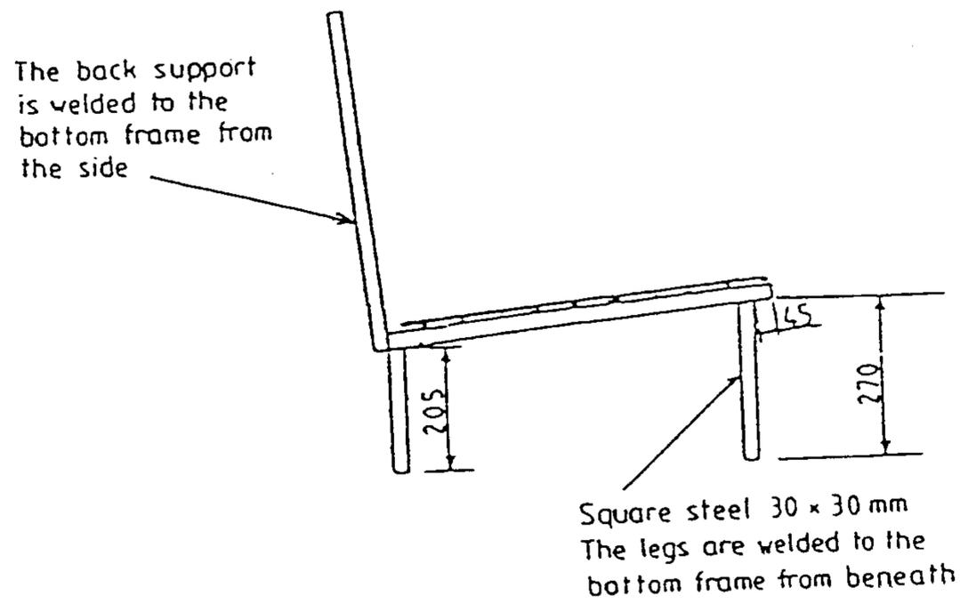
c) Side view of assembled seat frame.
