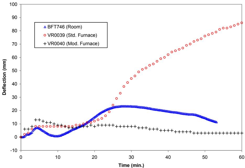
**Figure 6-6.** Modified furnace test on plasterboard wall: Comparison of deflection at mid-point of wall obtained during the furnace and room tests.
