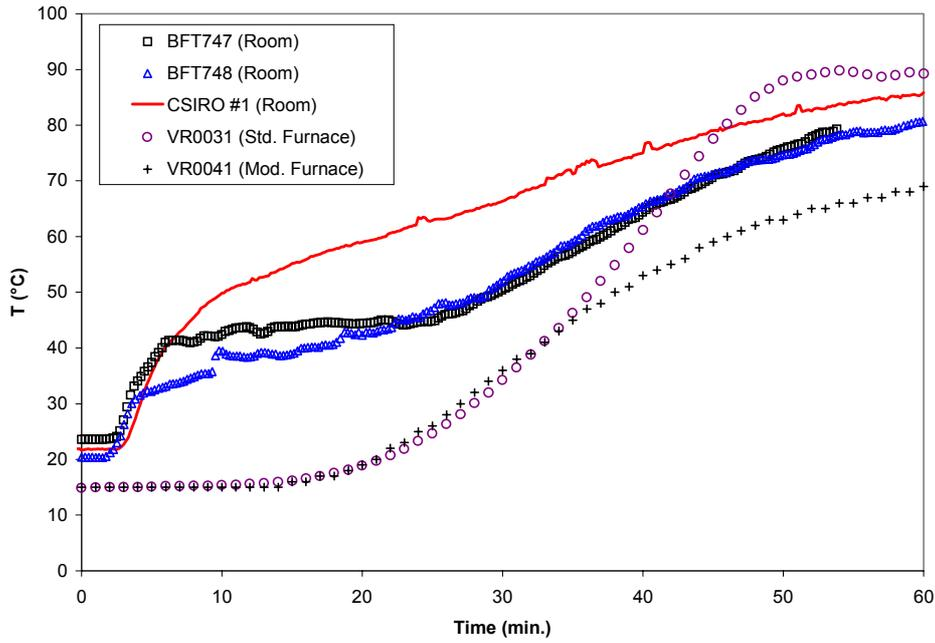
**Figure 6-2.** Modified furnace test on masonry wall: Comparison of average unexposed-face wall temperatures (thermocouples *U1-U5*) obtained during the furnace and room tests.
