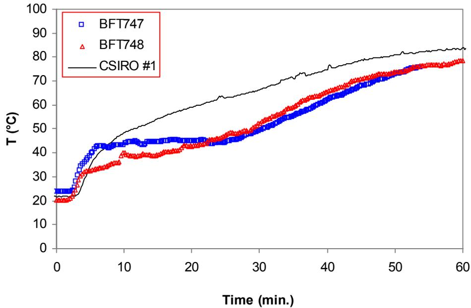
**Figure 4-10.** Masonry test walls: Unexposed-face average temperatures (thermocouples *UI-U7*) recorded during room tests.
