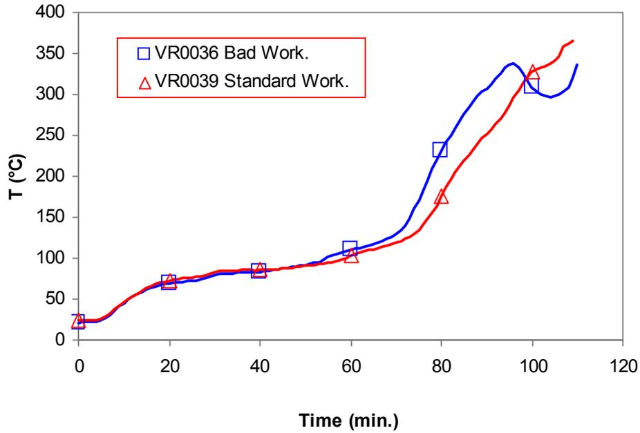
**Figure 5-7.** Average temperature on unexposed faces of plasterboard walls. Standard furnace test.
