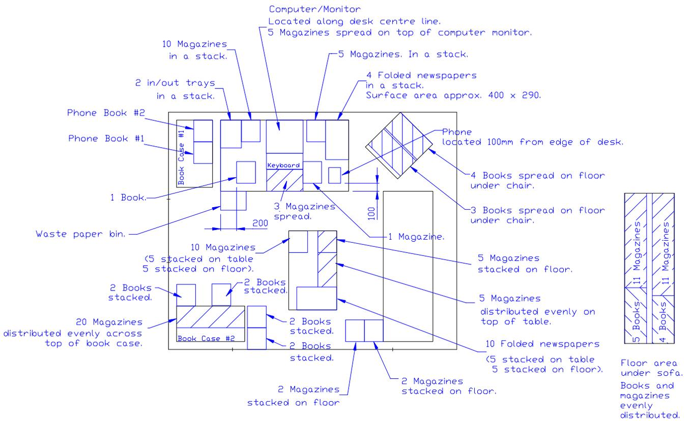
**Figure 12 Additional fire load layout.**
