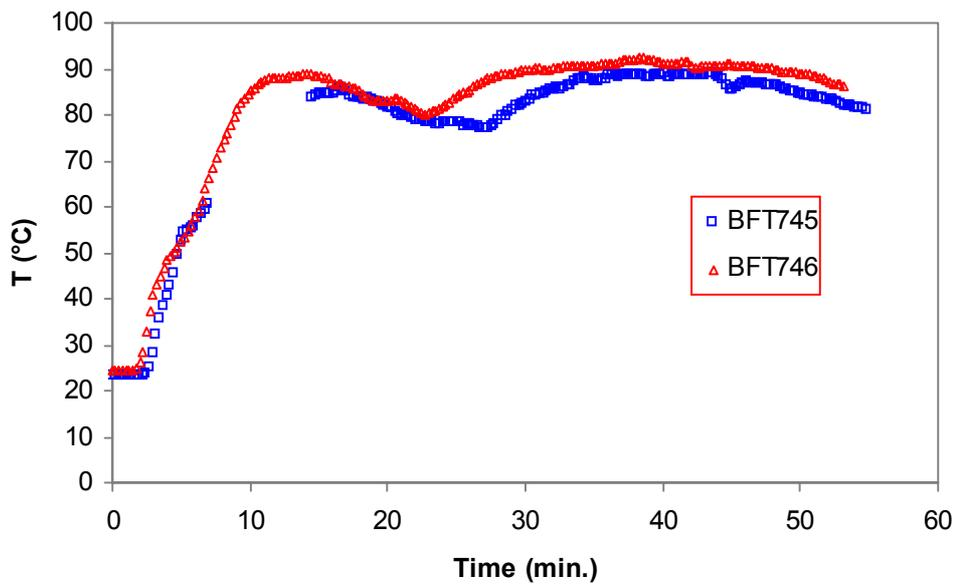
**Figure 4-14.** Plasterboard test walls: Unexposed-face maximum temperatures recorded during room tests.
