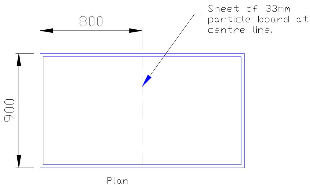
The top, one long side (1600 x 700), and one narrow side (900 x 700) located furthest from Bookcase #1, are to be lined with 33mm particle board. A 900mm x 700mm sheet of 33mm particle board is also to be fitted vertically at the centre line of the desk.
