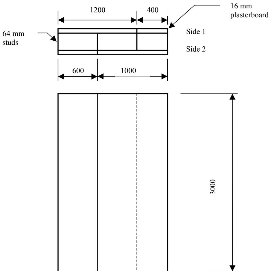
**Figure 9 Standard-workmanship plasterboard test wall for BHP furnace tests.**
