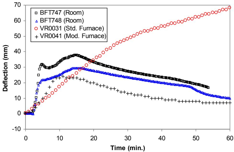
**Figure 6-3.** Modified furnace test on masonry wall: Comparison of deflection at mid-point of wall obtained during the furnace and room tests.
