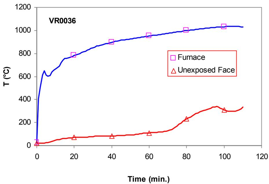
**Figure 5-6.** Average temperature versus time for bad-workmanship plasterboard wall. Standard furnace test.
