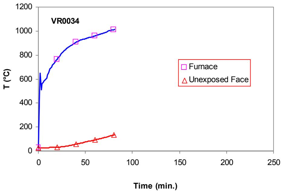
**Figure 5-2.** Average temperature versus time for *bad-workmanship* masonry wall. Standard furnace test.
