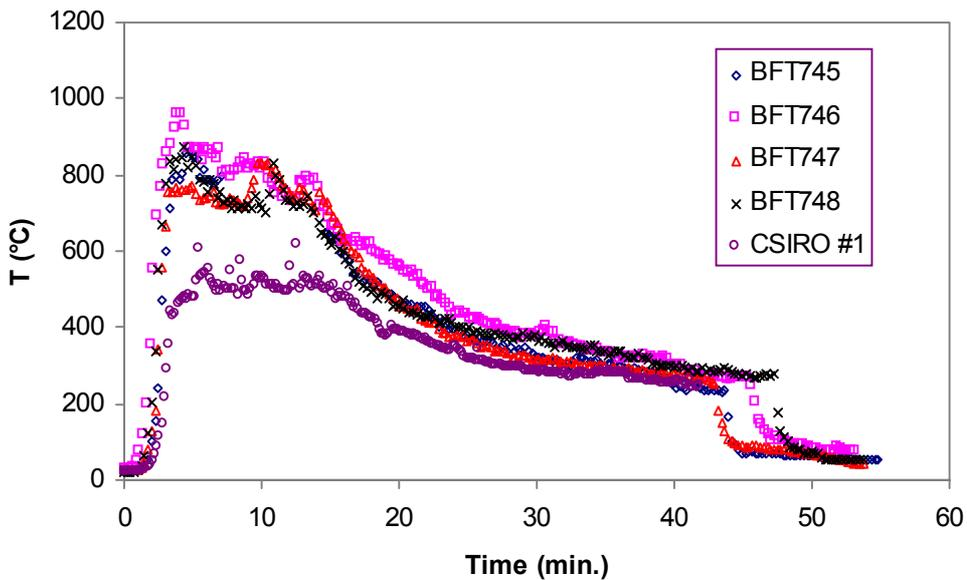
**Figure 4-9.** Room air temperatures (average of thermocouples  $A1-A20$ ): A comparison of five room tests.
