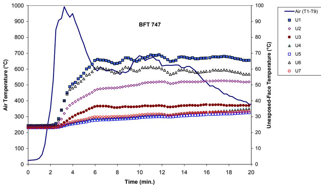
**Figure 8-1.** Temperatures recorded during room test on masonry wall.
