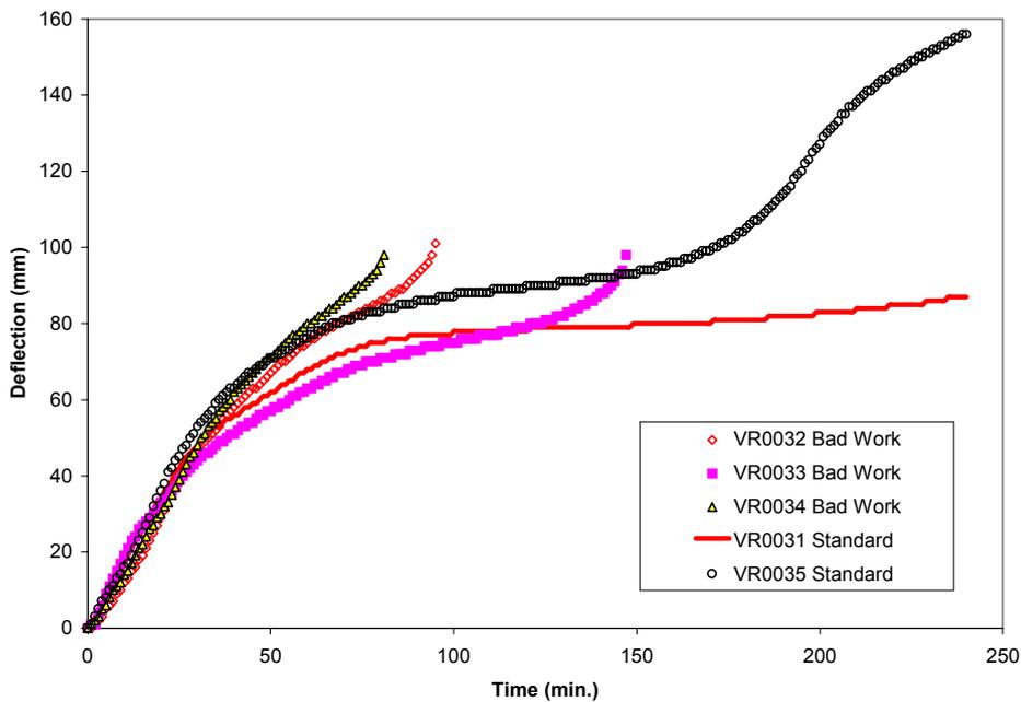
**Figure 5-4.** Deflection measured at midpoint of standard and bad-workmanship masonry walls. Standard furnace test.
