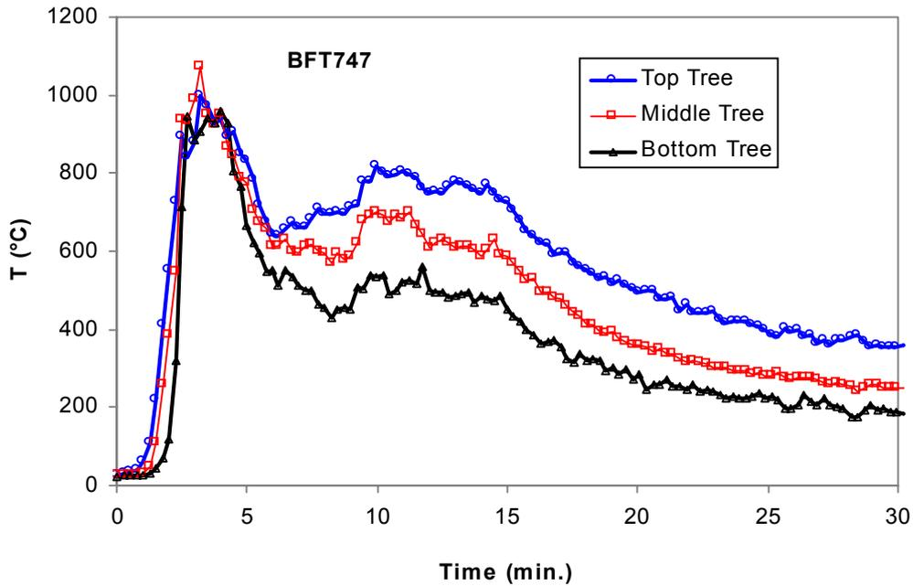
**Figure 4-2.** Air-temperature variations on exposed face *BFT 747*.
