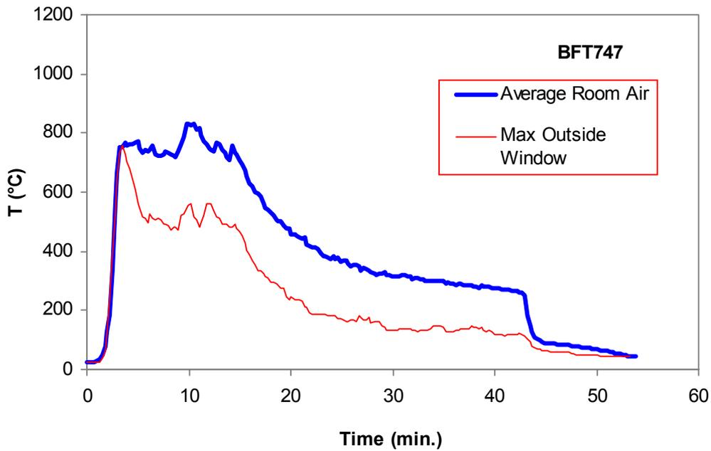
Figure 4-6. Air temperature in room compared to temperature outside window.
