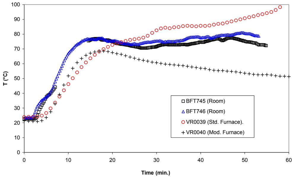
**Figure 6-5.** Modified furnace test on plasterboard wall: Comparison of average unexposed-face wall temperatures (thermocouples *U1-U5*) obtained during the furnace and room tests.
