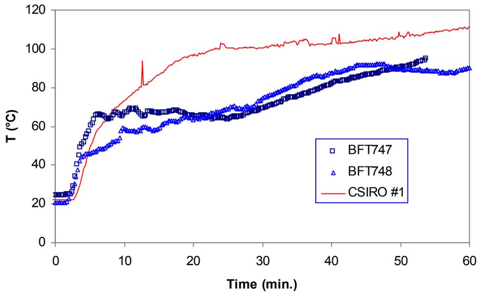
**Figure 4-11.** Masonry test walls: Unexposed-face maximum temperatures (thermocouples *UI-U7*) recorded during room tests.
