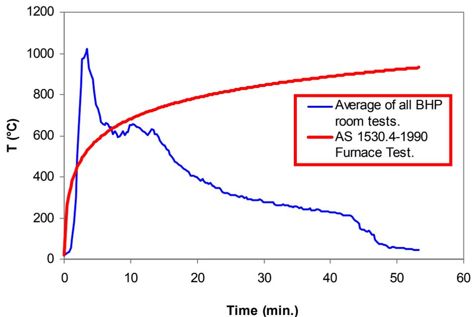
**Figure 7-1.** Exposed-face air temperatures measured during BHP room tests compared with the standard furnace test from AS1530.4-1990.
