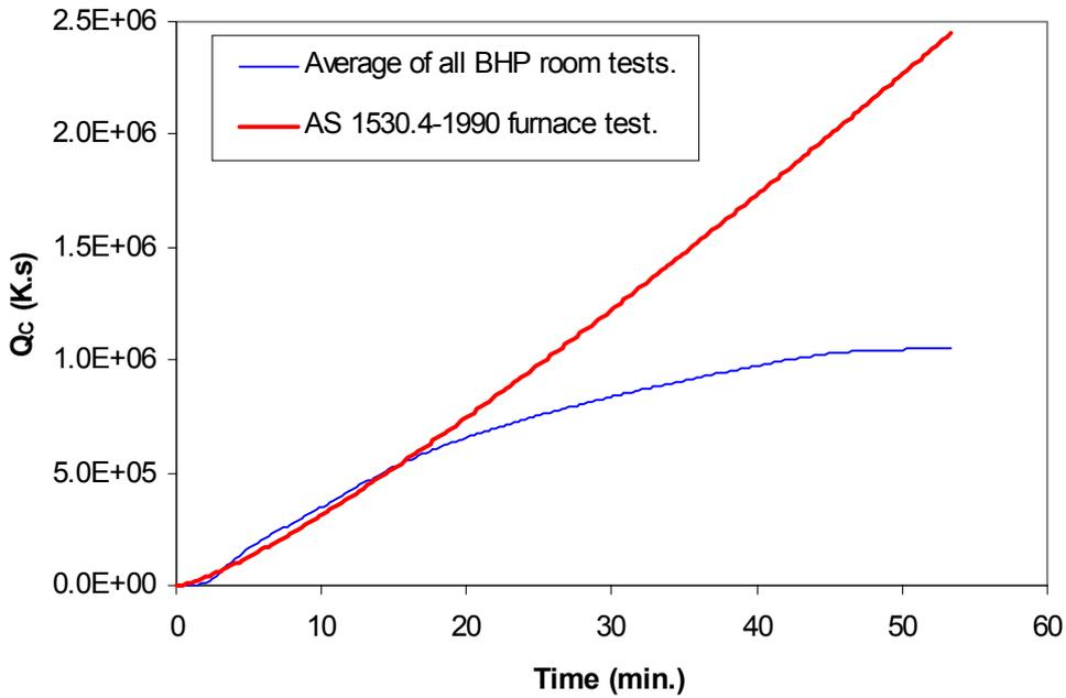
**Figure 7-3.** Integrated values of the time-temperature curves recorded near the exposed faces of the test walls.
