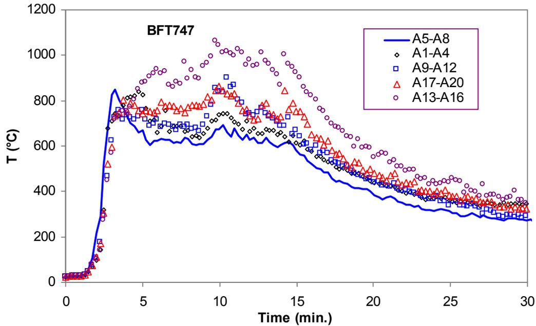
**Figure 4-7.** Room-air temperatures in different corners of room.
