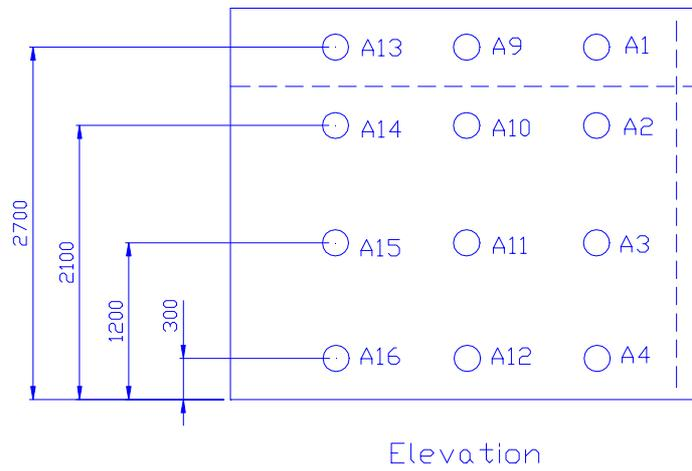
**Figure 3-3.** Location of air-temperature thermocouples.
