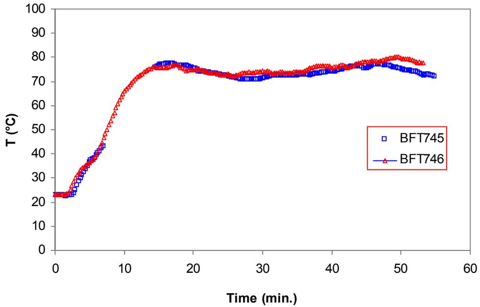
**Figure 4-13.** Plasterboard test walls: Unexposed-face average temperatures (thermocouples *U1-U7*) recorded during room tests.
