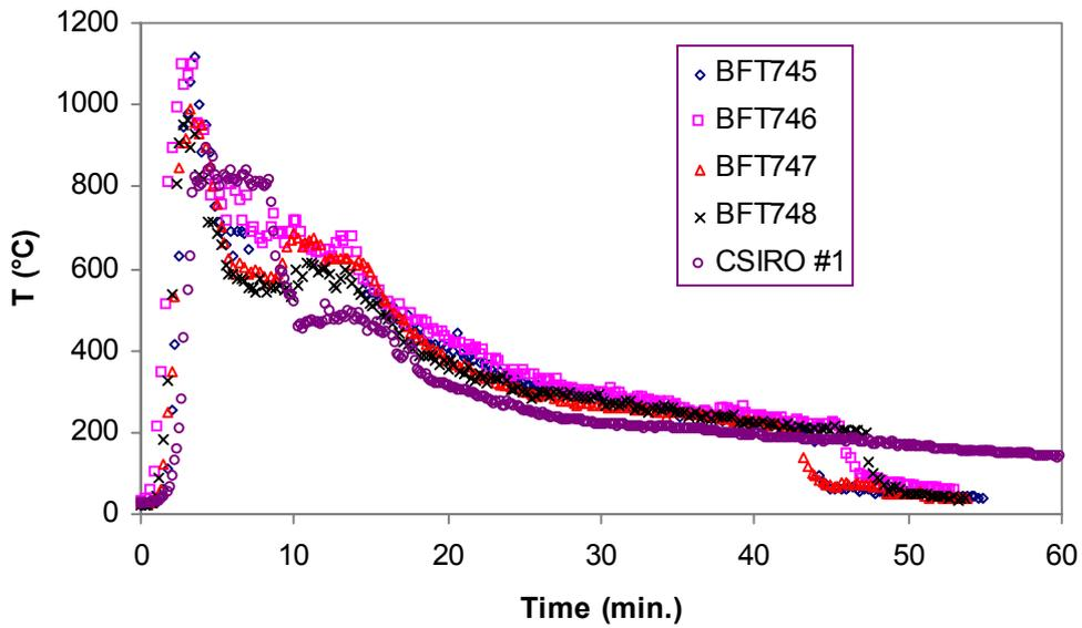
**Figure 4-8.** Exposed-wall air temperatures (average of thermocouples  $T1-T9$ ): A comparison of five room tests.
