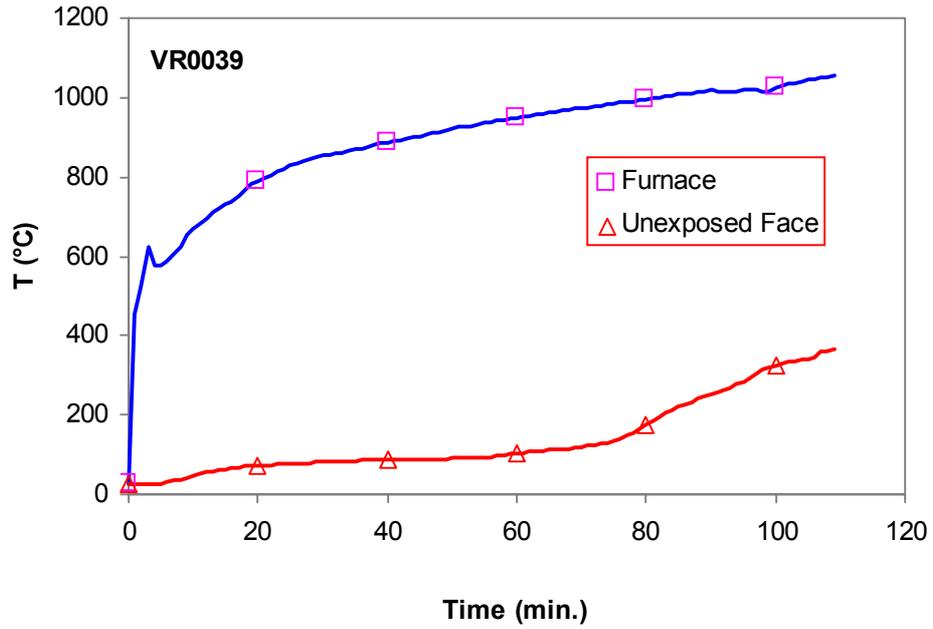
**Figure 5-5.** Average temperature versus time for standard-workmanship plasterboard wall. Standard furnace test.
