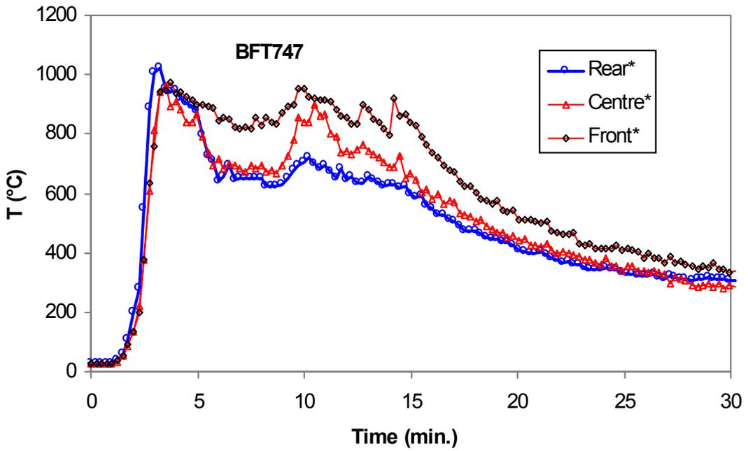
Figure 4-5. Adjusted temperature variations between the front and rear of room.
