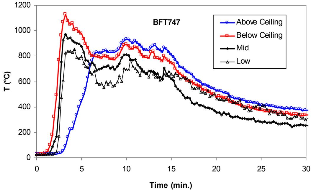
**Figure 4-4.** Room air temperatures at different levels.
