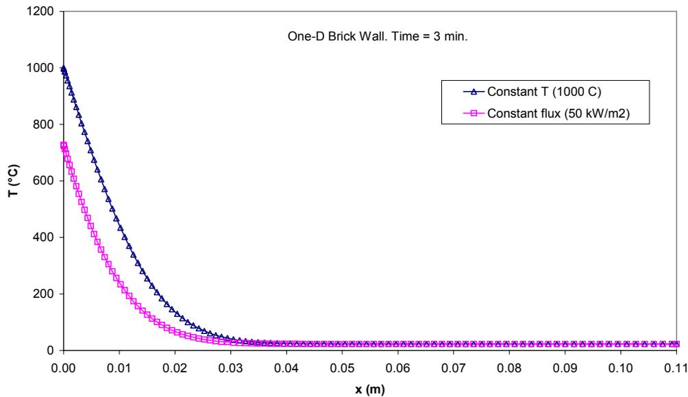
**Figure 8-2.** Theoretical temperature profile through thickness of brick wall at time 3 minutes.
