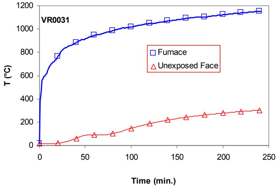
**Figure 5-1.** Average temperature versus time for *standard-workmanship* masonry wall. Standard furnace test.
