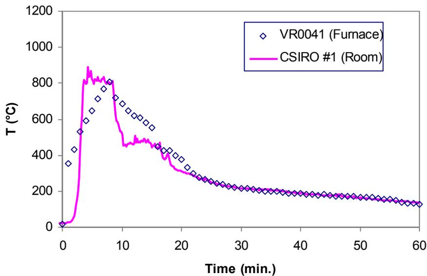
**Figure 6-1.** Modified furnace test on masonry wall: Comparison of average furnace temperatures with average room-test air temperatures.
