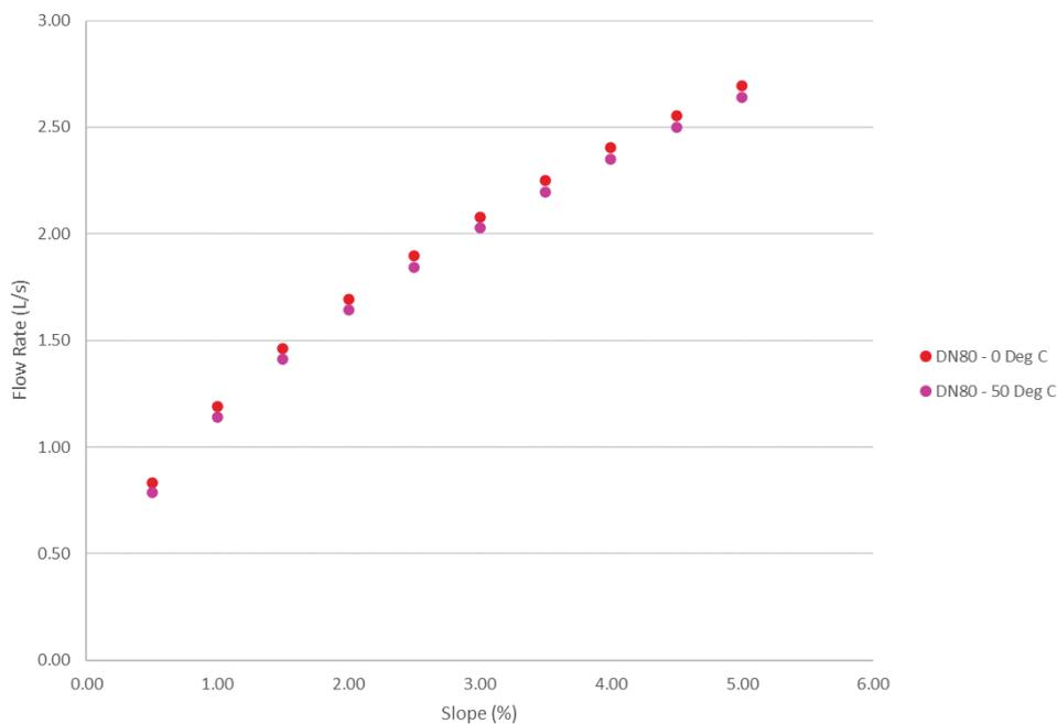
Figure 42: Effect of viscosity on flow rate for h/D=0.5 and Australian PVC-U internal pipe diameters
