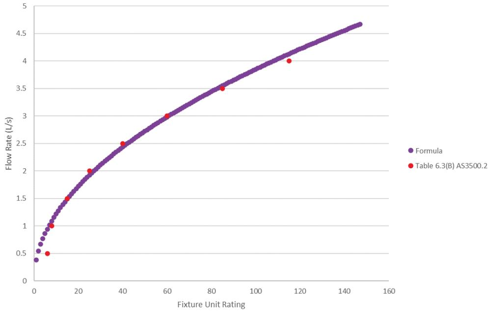
**Figure 46: Plot of fixture unit rating versus flow rate**
