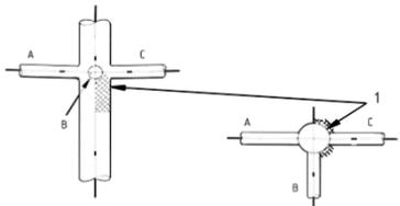
d) Other branches may be fitted at the same level as A, as shown at B and C. Each branch creates its own no connection zone. Only that of branch A is shown in this diagram.
