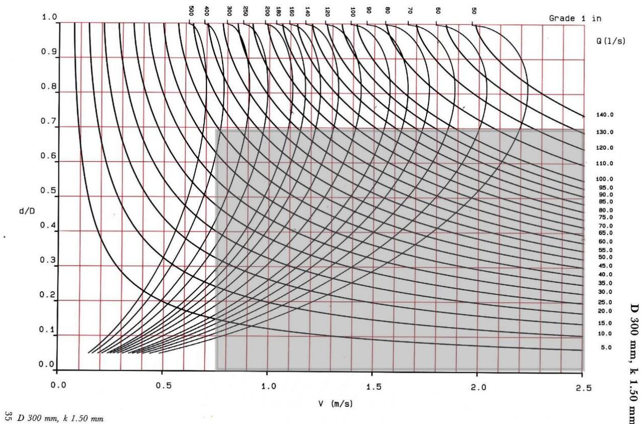
**Figure 8: A design chart for a pipe size of 300mm with a roughness coefficient of 1.5mm (Butler & Pinkerton, 1987)**
