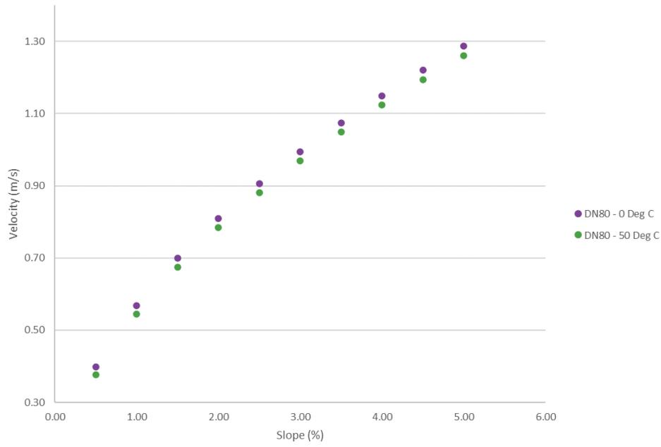
**Figure 43: Effect of viscosity on velocity for h/D=0.5 and Australian PVC-U internal pipe diameters**
