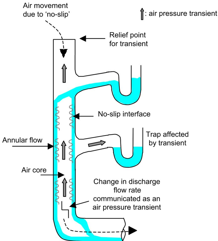
**Figure 23: Annular flow within stacks and effects of flow rate changes on pressure transients (Jack & Swaffield, 2009)**
