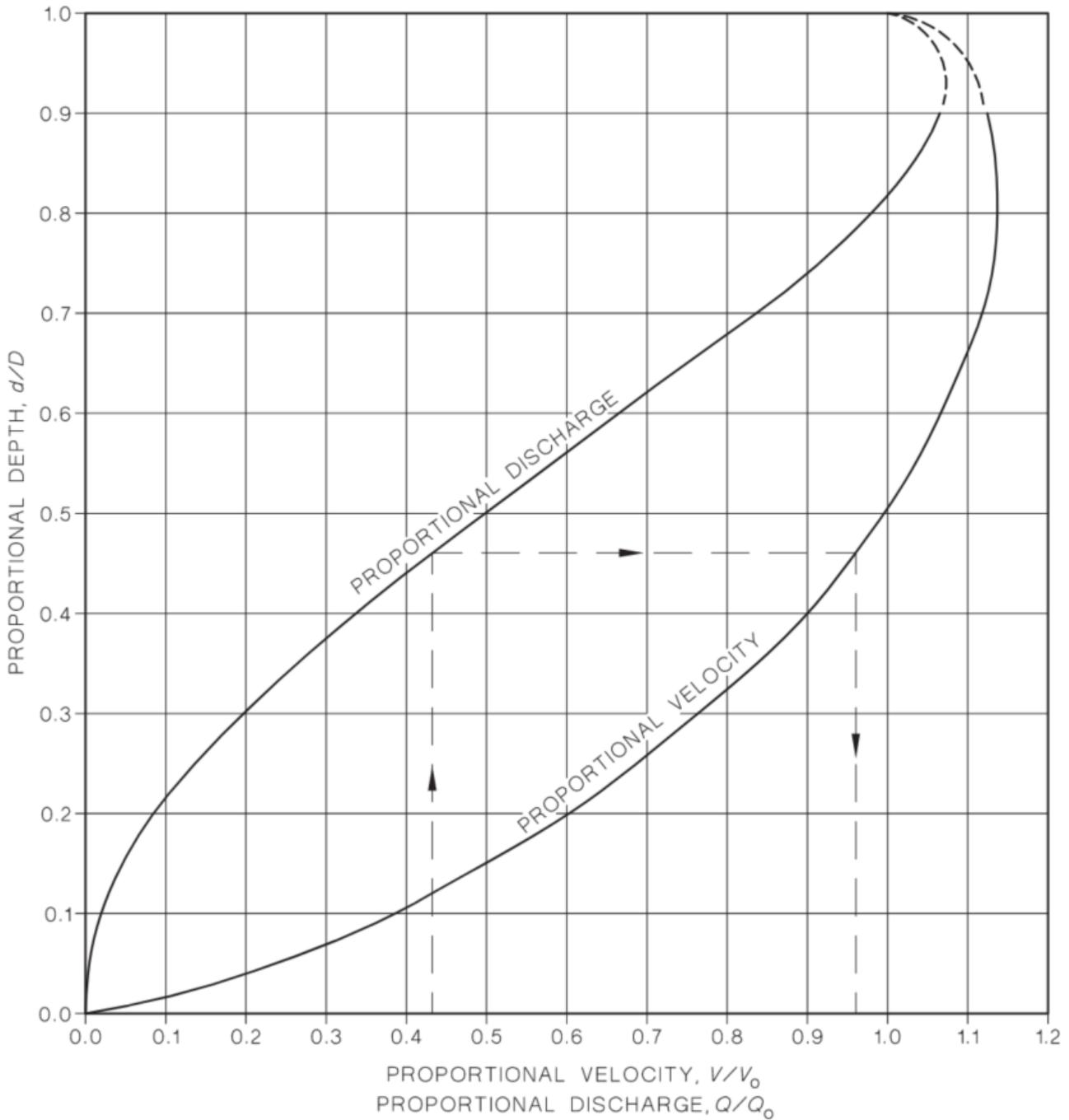
Figure 10: Chart provided in AS 2200-2006 to calculate non-full-bore flows (Standards Australia, 2006)
