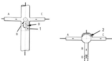
e) A branch may also be fitted at D, or elsewhere on the same vertical centre line. Although this would be on the boundaries of the no connection zones of branches A and C, its centre line would not be inside either of them. But as branch B has no connection zone on the far side of the stack, it would not be possible to fit a branch opposite branch D.
