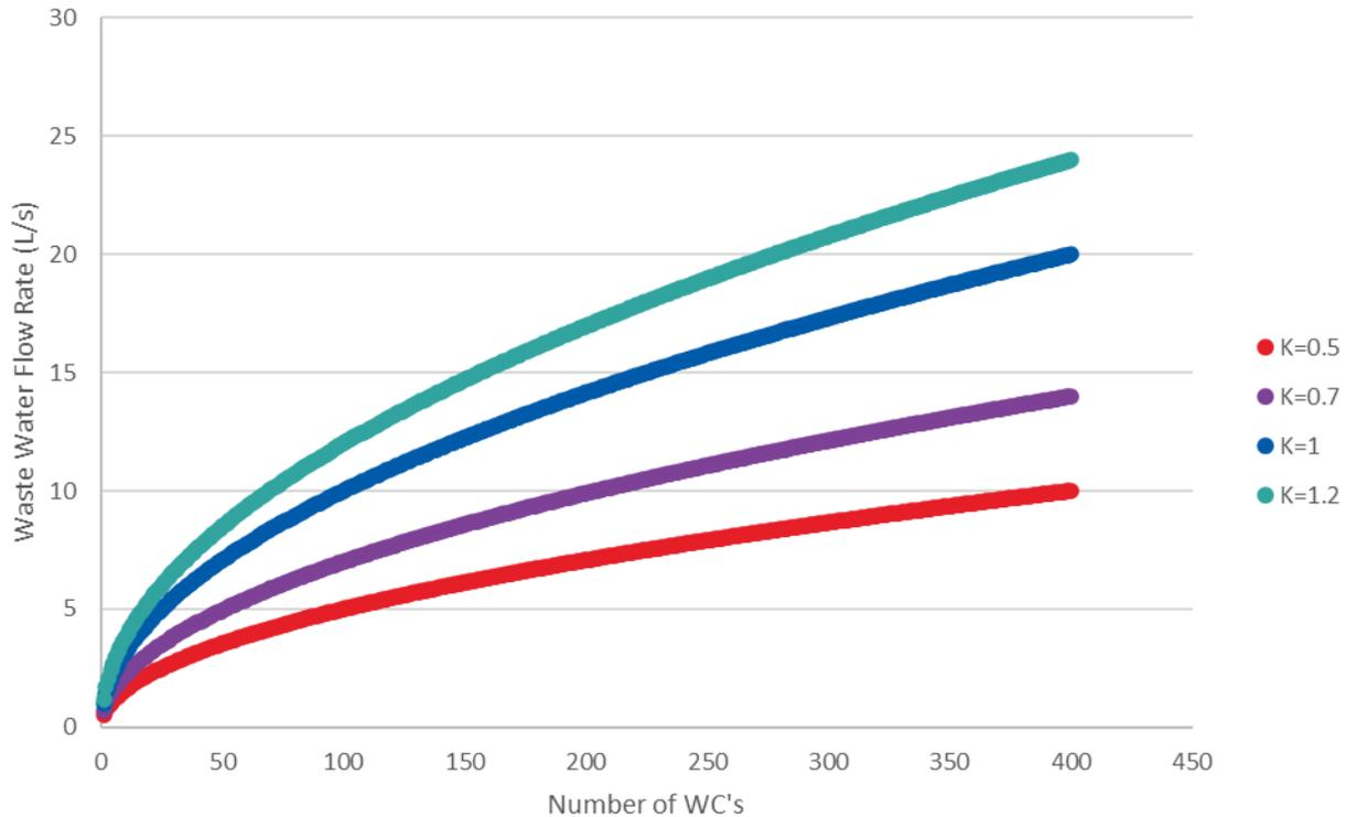
**Figure 44: Discharge units versus flow rate for the four frequency factors**
