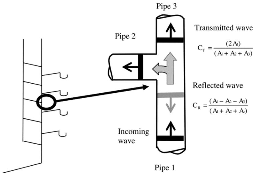
Figure 2.8 Typical three-pipe junction in a building drainage and vent system vertical stack; assume transient arrives from below along pipe 1, possibly due to a change in flow conditions further down the building
