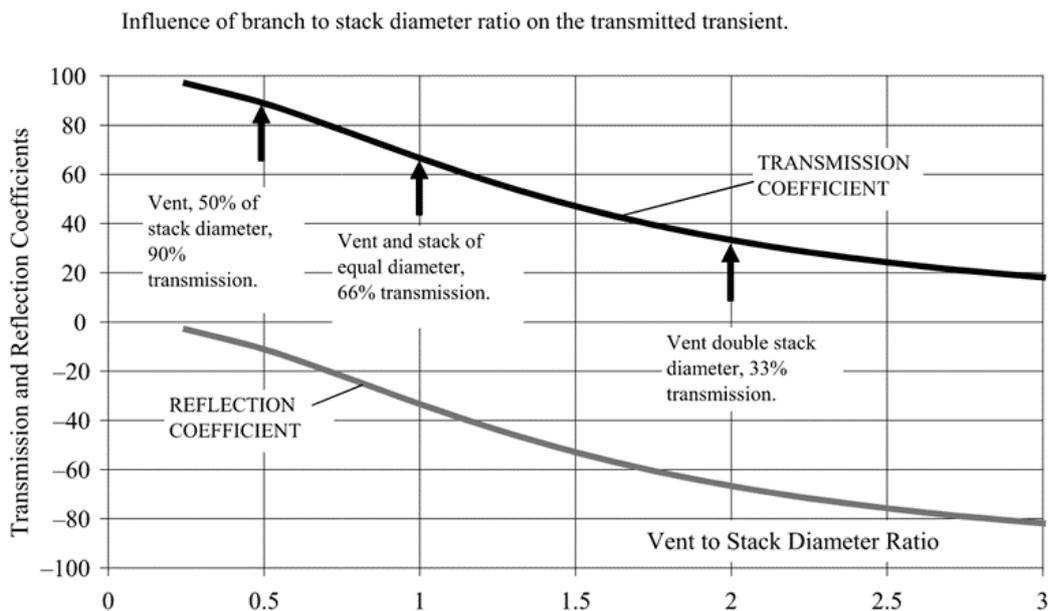
Figure 2.9 Reflection and transmission at a three-pipe junction expressed as % of the incoming wave, taken here as a positive low amplitude air pressure transient
