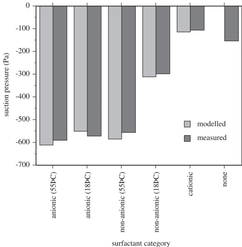
**Figure 25: Summary of simulated versus measured air pressures for various detergent classes at set temperatures in 100mm x 5.8m tall glass stack with closed entry to simulate temporary blockage (Campbell, 2007)**
