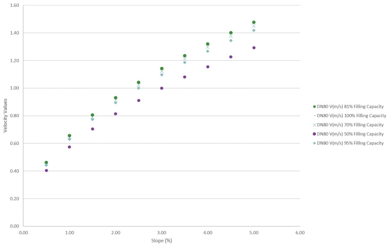
Figure 39: Velocities for varying filling capacities for DN80 pipe (Australian Internal diameter)
