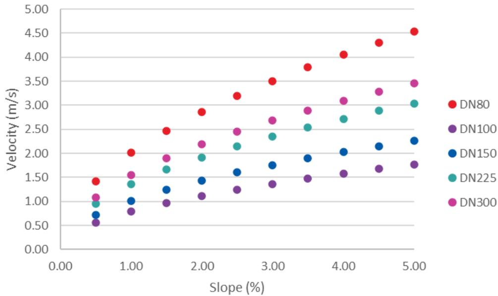
Figure 41: Effect of diameter on velocity for h/D=0.7 and Australian PVC-U internal pipe diameters
