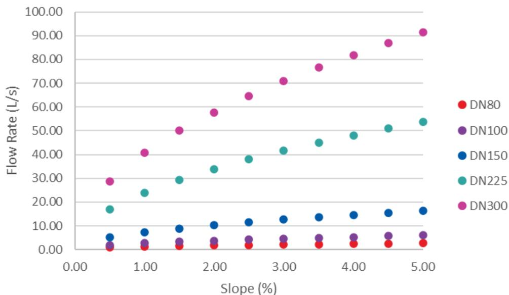
**Figure 40: Effect of diameter on flow rate for h/D=0.7 and Australian PVC-U internal pipe diameters**
