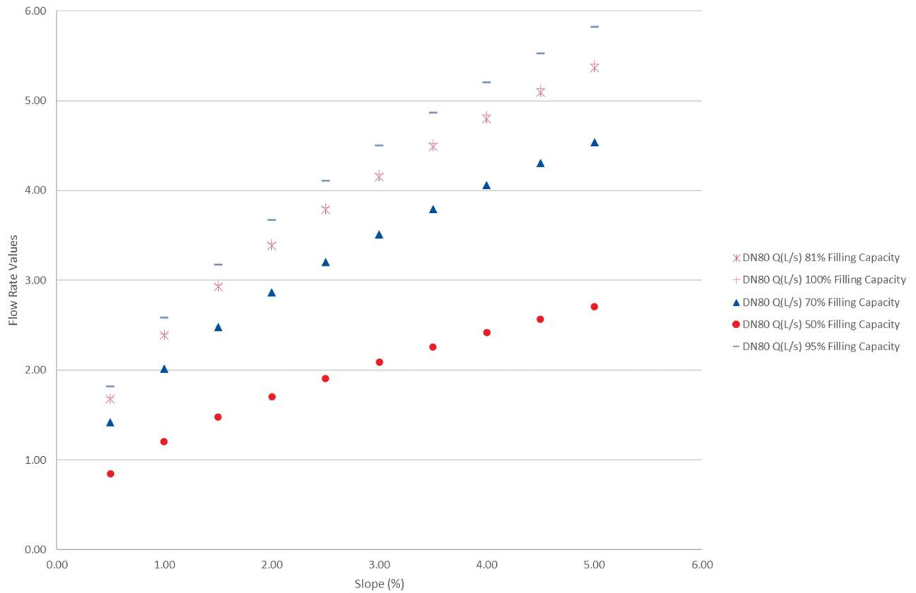
Figure 38: Flow rates for varying filling capacities for DN80 pipe (Australian internal diameter)
