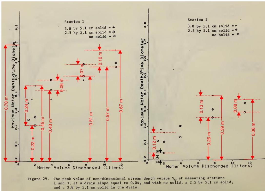
Figure 49: Annotated Results of Flow depth versus water volume discharged at Station 1 and 3 (Mahajan, 1981)
