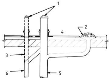
b) For stack vents also collecting rainwater from roofs
