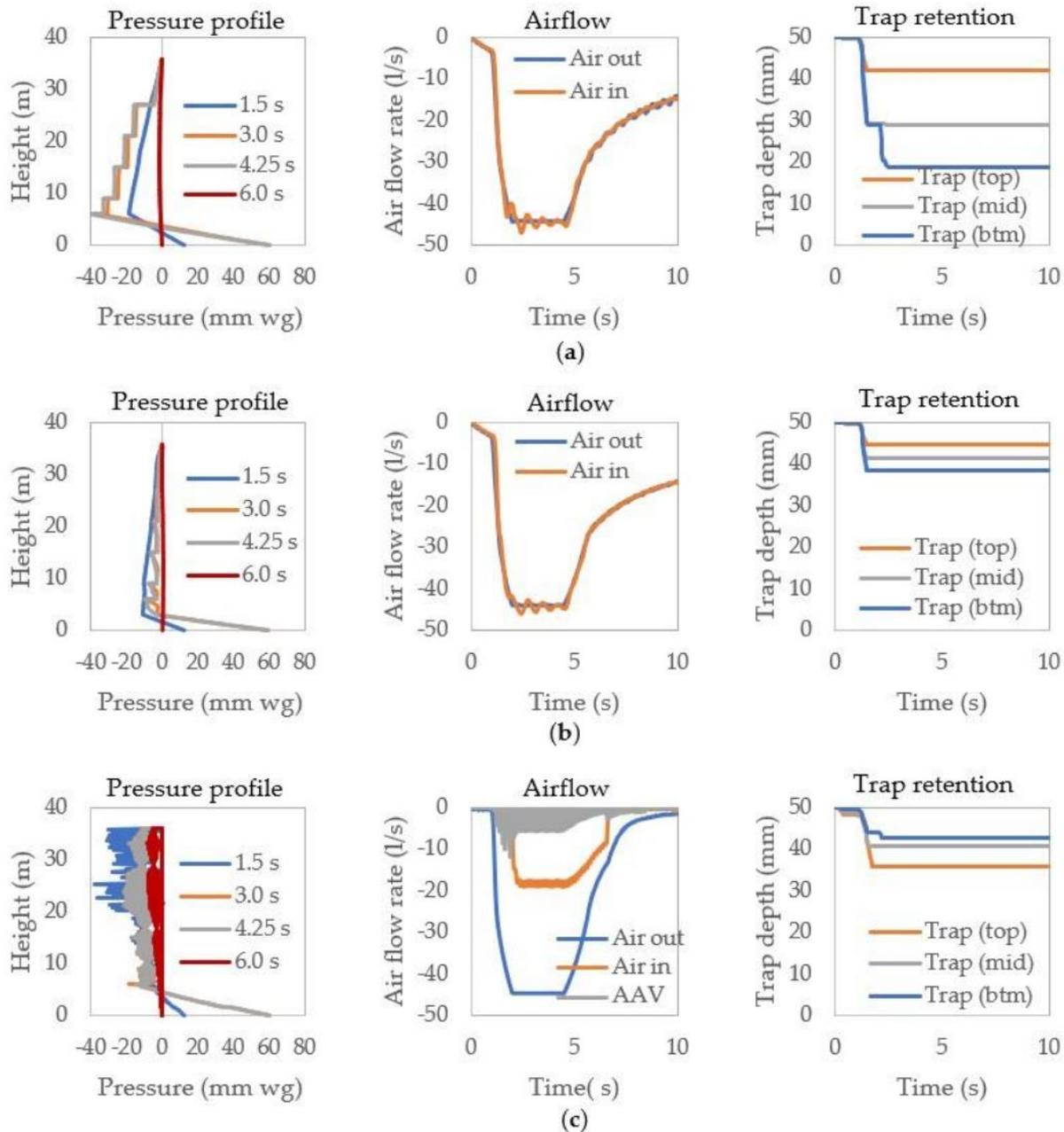
**Figure 24: Simulated elements of operational performance for 10 story building with 100 mm dia. stack in system configurations: (a) single-stack; (b) fully-vented; and (c) single-stack with AAVs (Gormley, et al., 2021)**
