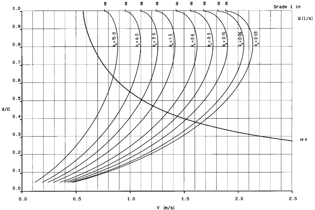
Figure 7: Sensitivity of flow rate and velocity to roughness (Butler & Pinkerton, 1987)
