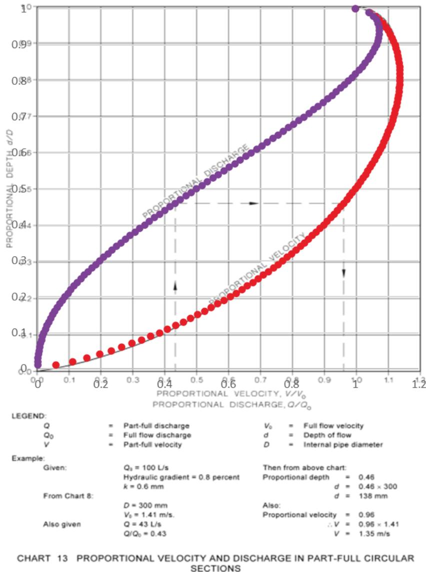
**Figure 36: Proportional velocity and flowrate for various filling ratios for 143mm internal diameter pipe at 5% slope (Standards Australia, 2006)**
