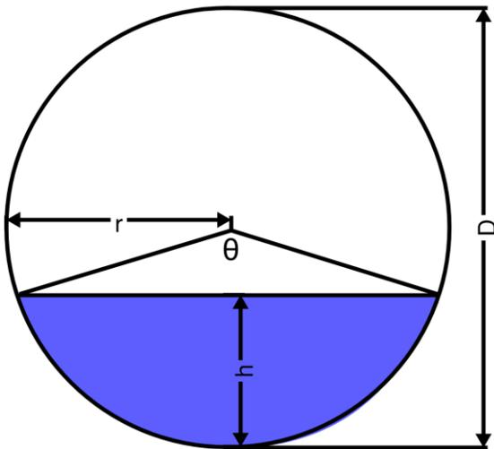
**Figure 1: Radius ( $r$ ), central angle ( $\theta$ ) and depth of water ( $h$ ) of a partly filled pipe**
