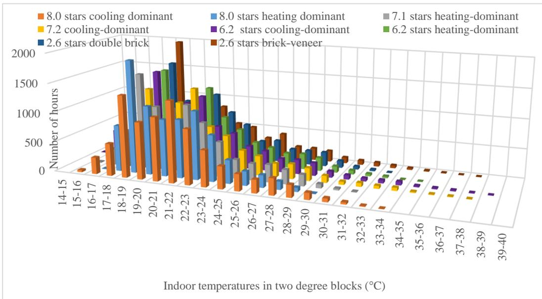
Figure 10 Overheating analysis of a north-facing bedroom for the whole year in Adelaide
