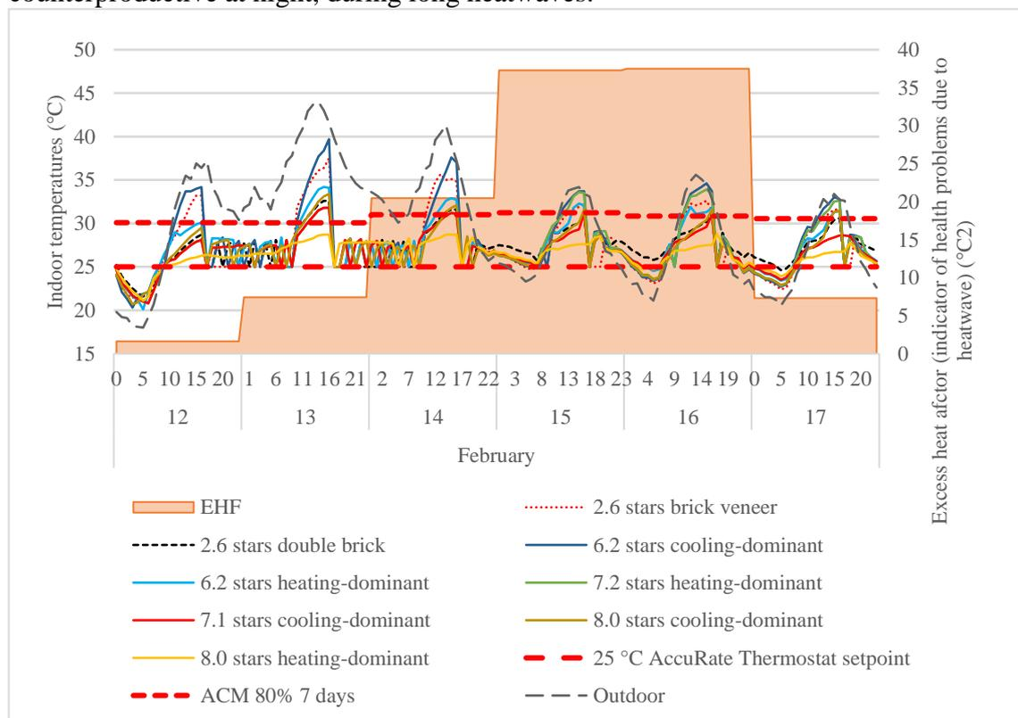
Figure 12 Overheating analysis of a north-facing bedroom during a medium heatwave period in Adelaide
