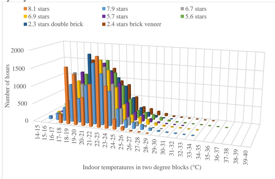
Figure 11 Overheating analysis of a north-facing bedroom for the whole year in Sydney
