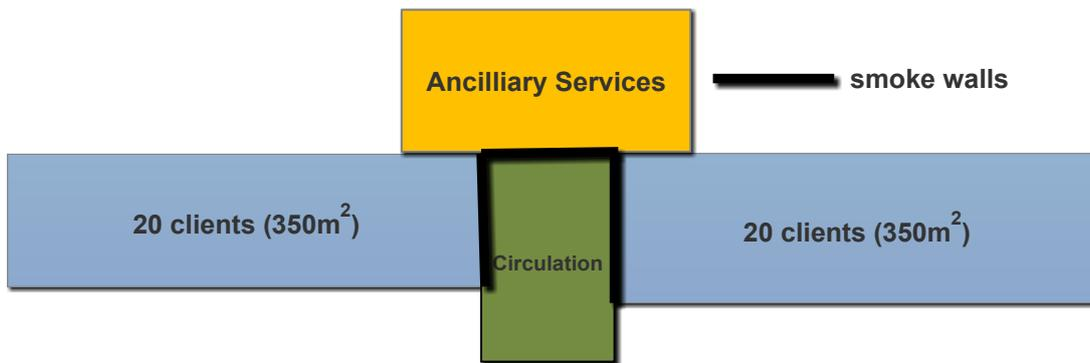
**Figure 10 Schematic Layout of Class 9c single storey building**
