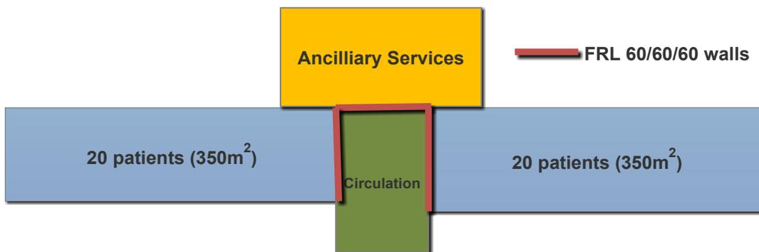
**Figure 11 Schematic Layout of Class 9a single storey building**
