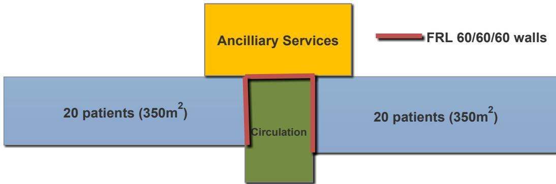
**Figure 20 Schematic Layout of Class 9a single storey building**
