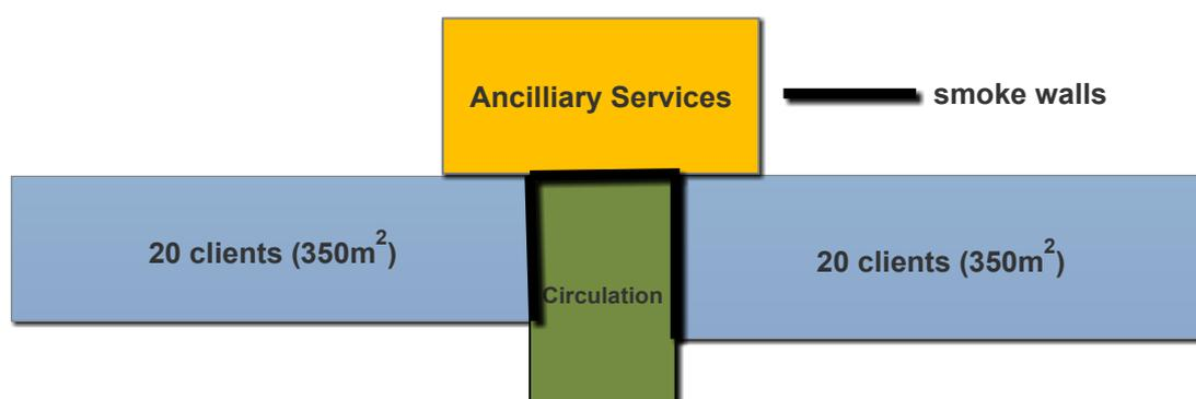
**Figure 19 Schematic Layout of Class 9c single storey building**
