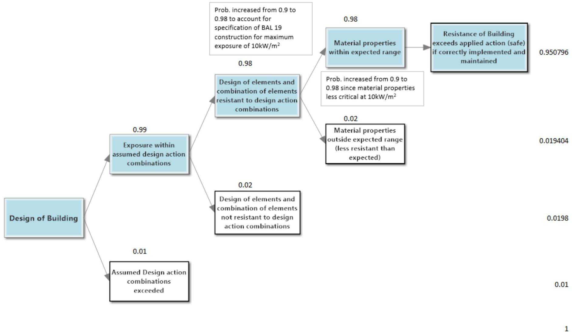
Figure 29 Event Tree for Design Process for Class 9 Buildings with explanation of change from values for Class 2 Buildings
