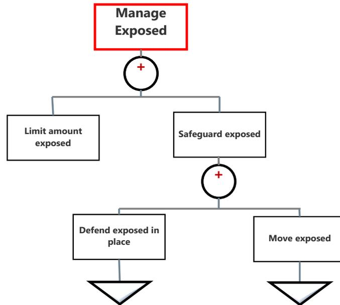
Figure 16 Manage Exposed Branch of the Fire Safety Concepts Tree
