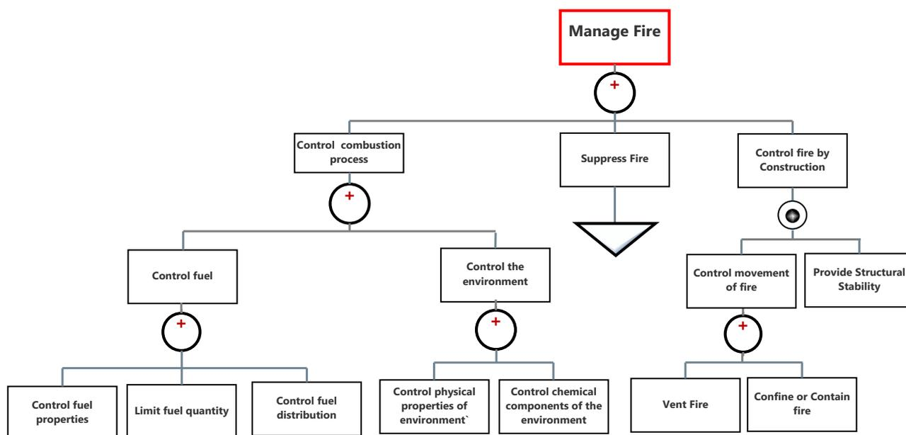
Figure 14 Expanded Manage Fire Branch
