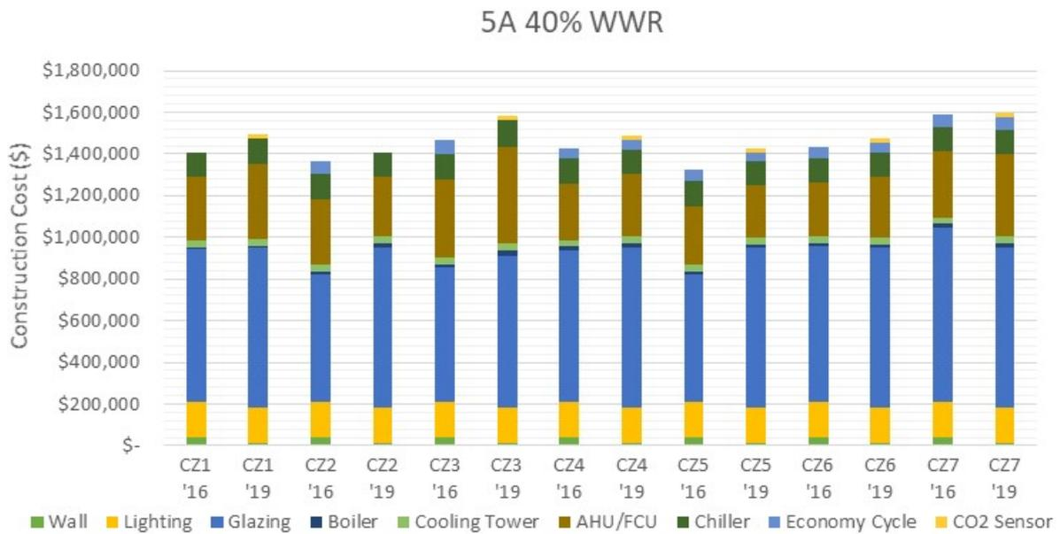
Figure 33: Comparison of initial construction cost for model 5A (40% WWR).
