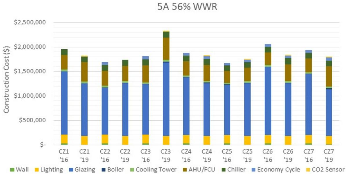
Figure 32: Comparison of initial construction cost for model 5A (56% WWR).
