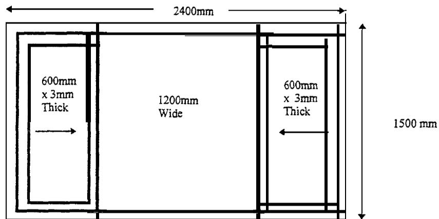
**Figure 3-7 Window W102 Construction Details**
