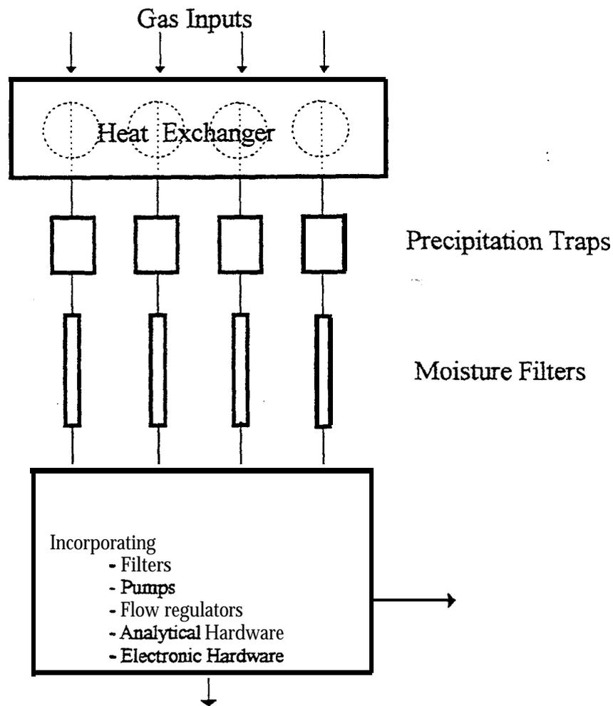
**Figure A.11** Chemical analysis flow diagram
