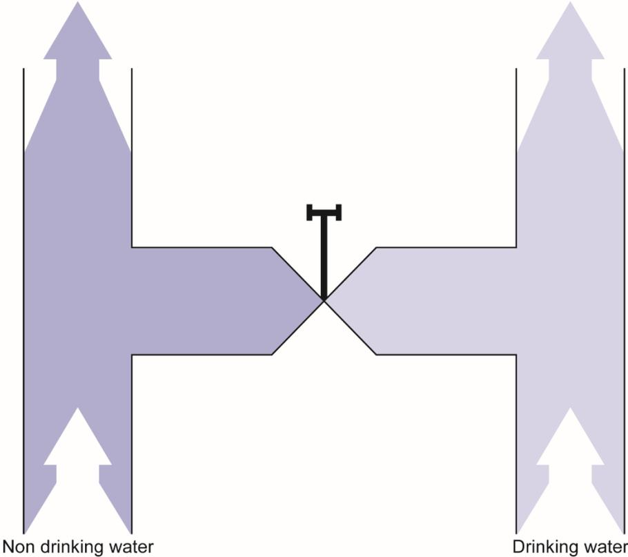
Figure 3.11 Valved connection between water supply and sanitary drainage system
