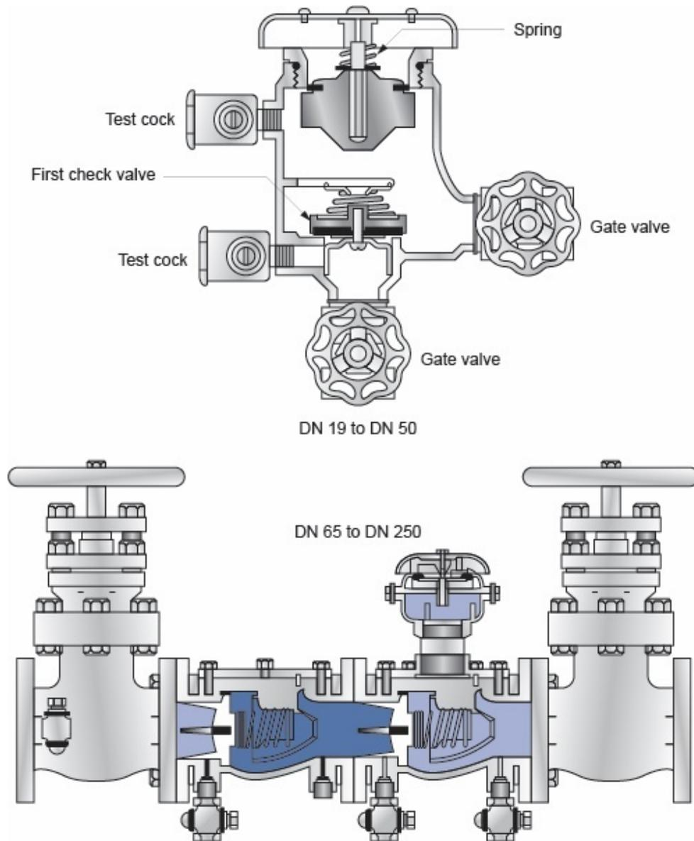
Figure 6.8 Pressure vacuum breaker - typical installation
