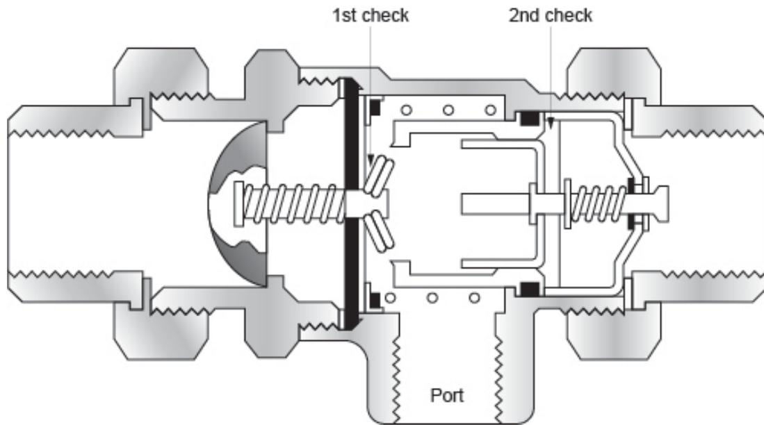
Line pressure keeps the vent port closed, but zero supply pressure or backsiphonage will open the inner chamber to atmosphere. With this device, extra protection is gained through the atmospheric venting capability.
