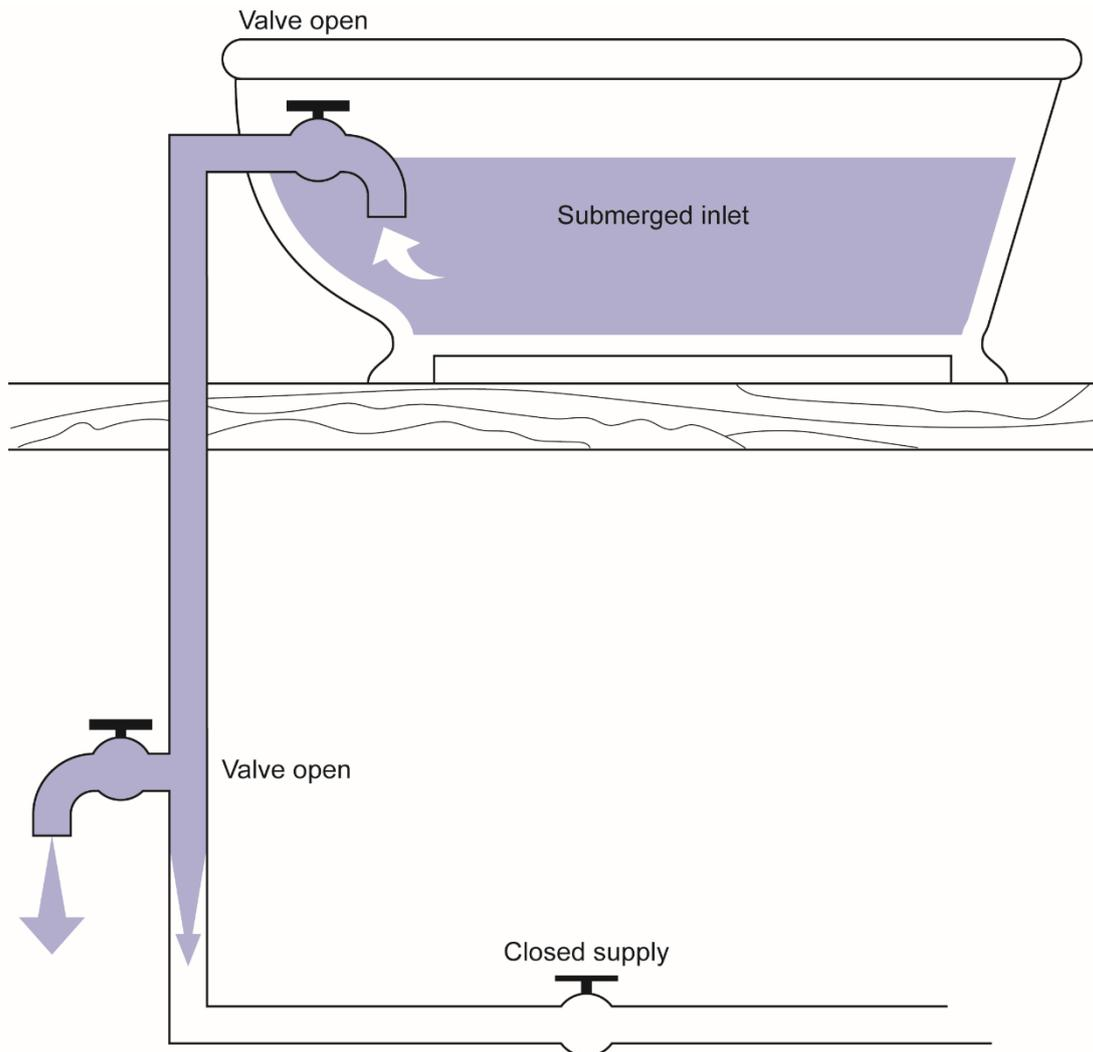
The siphon actions cited have been produced by reduced pressures resulting from a difference in the water levels at two separated points within a continuous fluid system.
