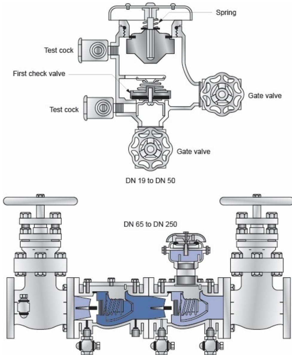
Figure 6.7 Pressure vacuum breaker (PVB)
