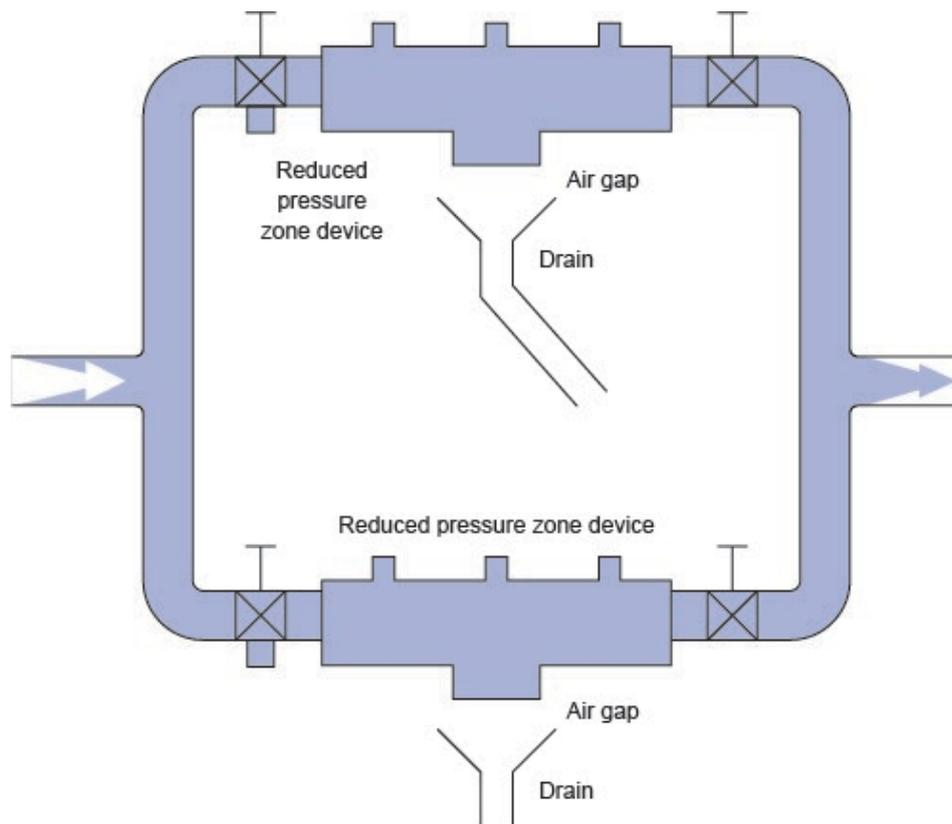
Note: although Figure 7.1 depicts a protected bypass using reduced pressure zone devices, other devices can also be installed, provided that an isolation valve is installed at the end of each device to enable it to be isolated from the water supply, and removed if found to be defective.
