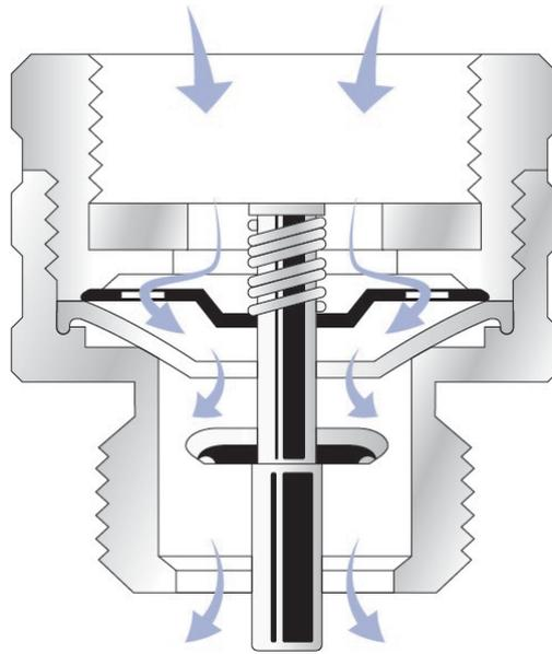
When the water supply is turned off, the device vents to atmosphere, thus protecting against backsiphonage conditions. Typical installation is shown in Figure 6.6.
