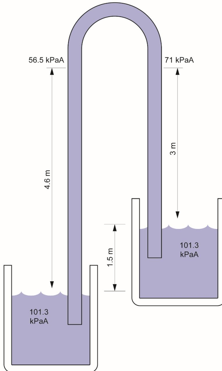
Figure 3.7 shows how this siphon principle can be hazardous in a plumbing system. If the supply valve is closed, the pressure in the line supplying the tap is less than the pressure in the supply line to the bathtub. Therefore flow will occur through siphonage, from the bathtub to the open tap.
