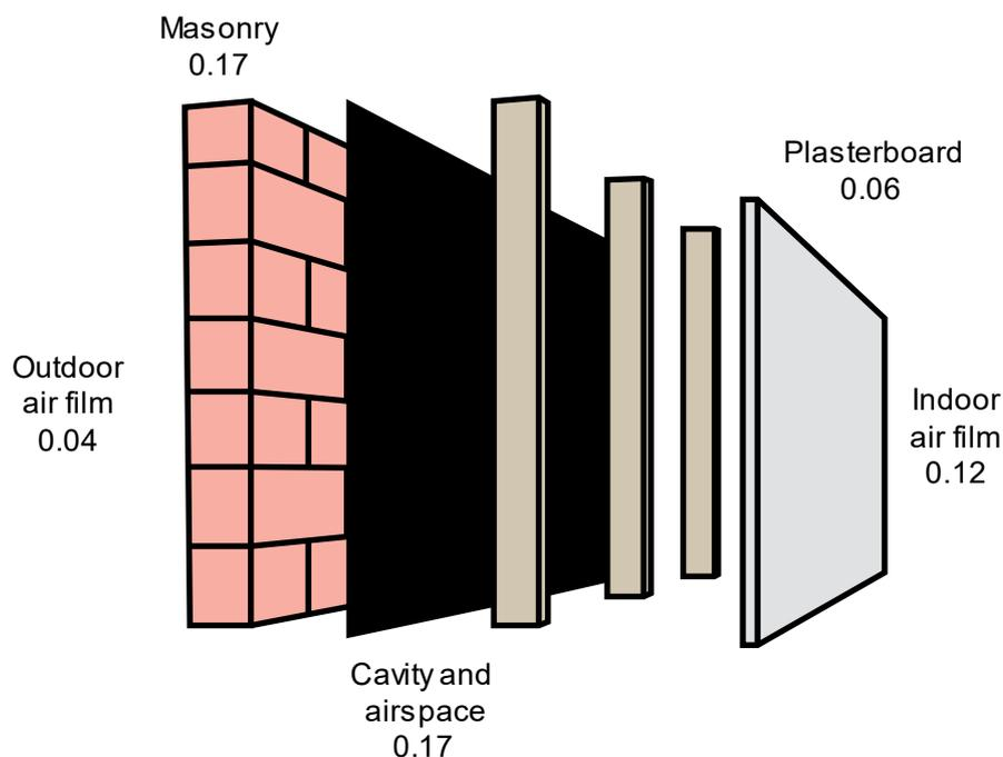
The figures below provide more detailed examples of typical insulation locations in various types of wall construction. The *Total R-Value* required is achieved by adding
