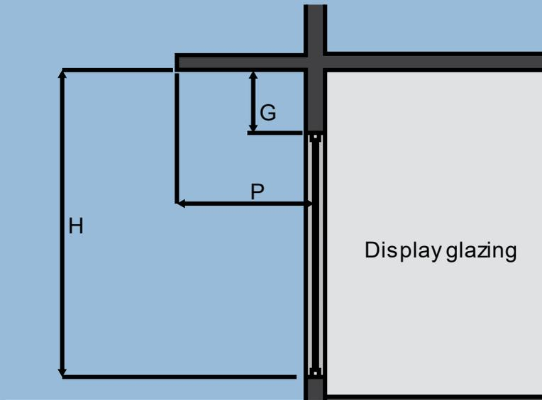
To determine the shading multiplier,  $G/H$  and  $P/H$  must first be calculated.
