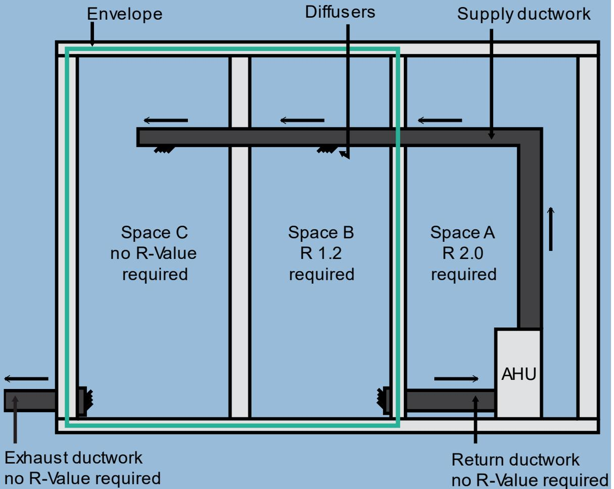
The building is in *climate zone 5* and the ductwork is greater than 3 m in length.
