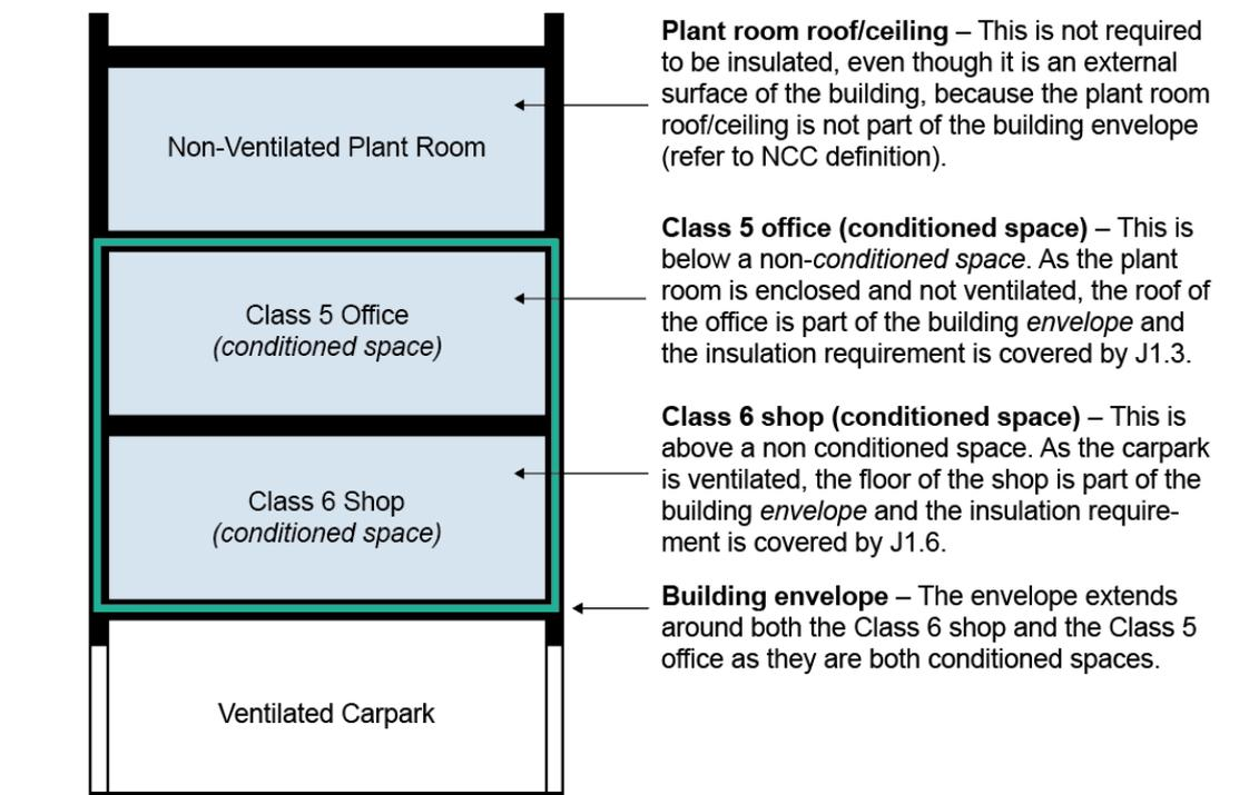
In practice, occupied spaces are likely to be conditioned at some time over the life of the building and their external elements will form the building *envelope*. The *envelope* can extend through multiple floors of a building encompassing any number of *conditioned spaces* that are located side by side or one above the other. However, the floor or wall between two *conditioned spaces* is not part of the *envelope* by definition because very little energy transfer is expected to occur.
