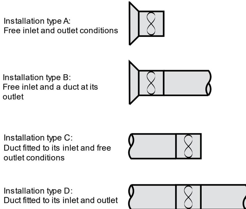
Installation types A and C require a minimum required system static efficiency, while installation types B and D require a minimum required system total efficiency.
