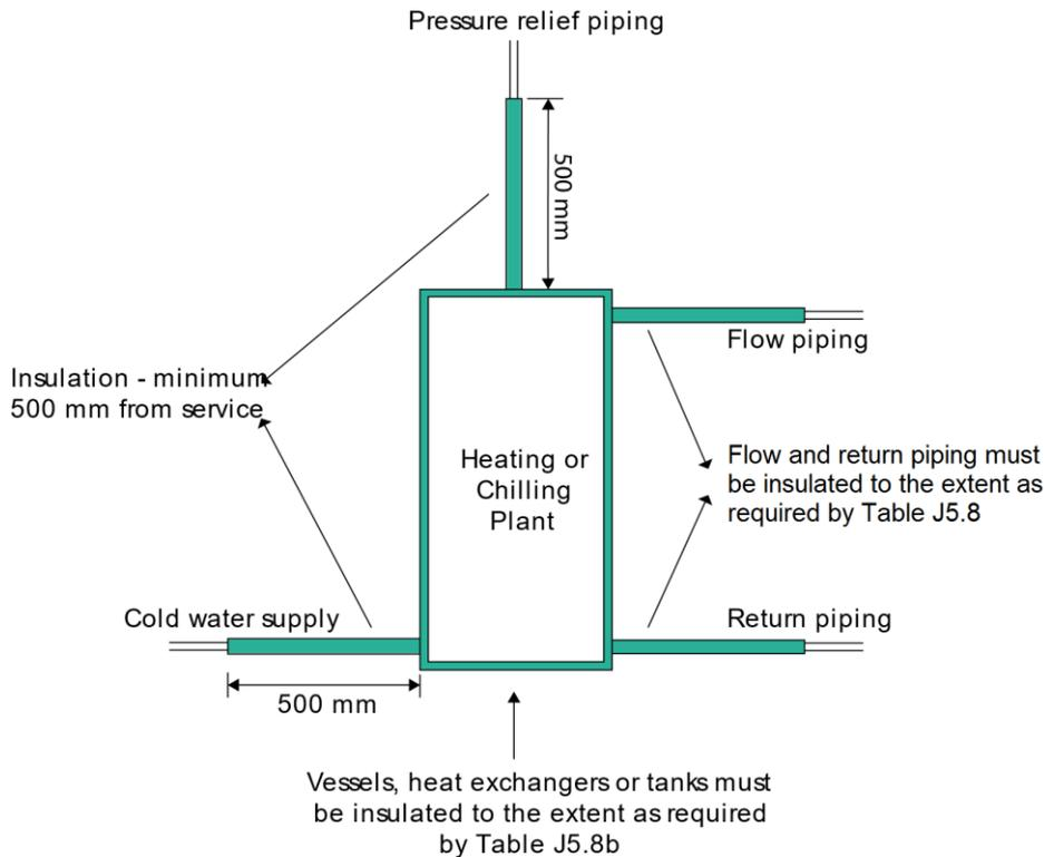
As an example, pressure relief piping is connected to a 40 mm diameter pipe carrying low temperature chilled water  $\leq 2$  °C. The pipe requires a minimum insulation *R-Value* of 1.3 and therefore the pressure relief piping, to 500 mm from the connection also requires insulation with *R-Value* of 1.3.
