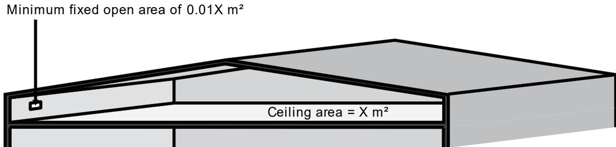
Subclause (d)(ii) specifies that a ventilated roof space could also be a roof space with at least 2 wind-driven roof ventilators with a total opening area of at least 0.14 m<sup>2</sup>. This requirement must be accompanied by vents with a total fixed open area of at least 0.2% of the ceiling area.
