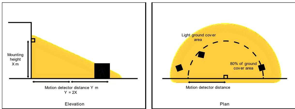
When outside a building, the motion detector must control less than or equal to 5 lights to avoid wasteful energy. The motion detector must use time switches to ensure the lighting does not operate during the day. Additionally, the motion detector must be configured so that the lights turn off after 15 minutes of the space being unoccupied and be *capable* of being overridden by a manual switch which is reset after a period of less than 4 hours.
