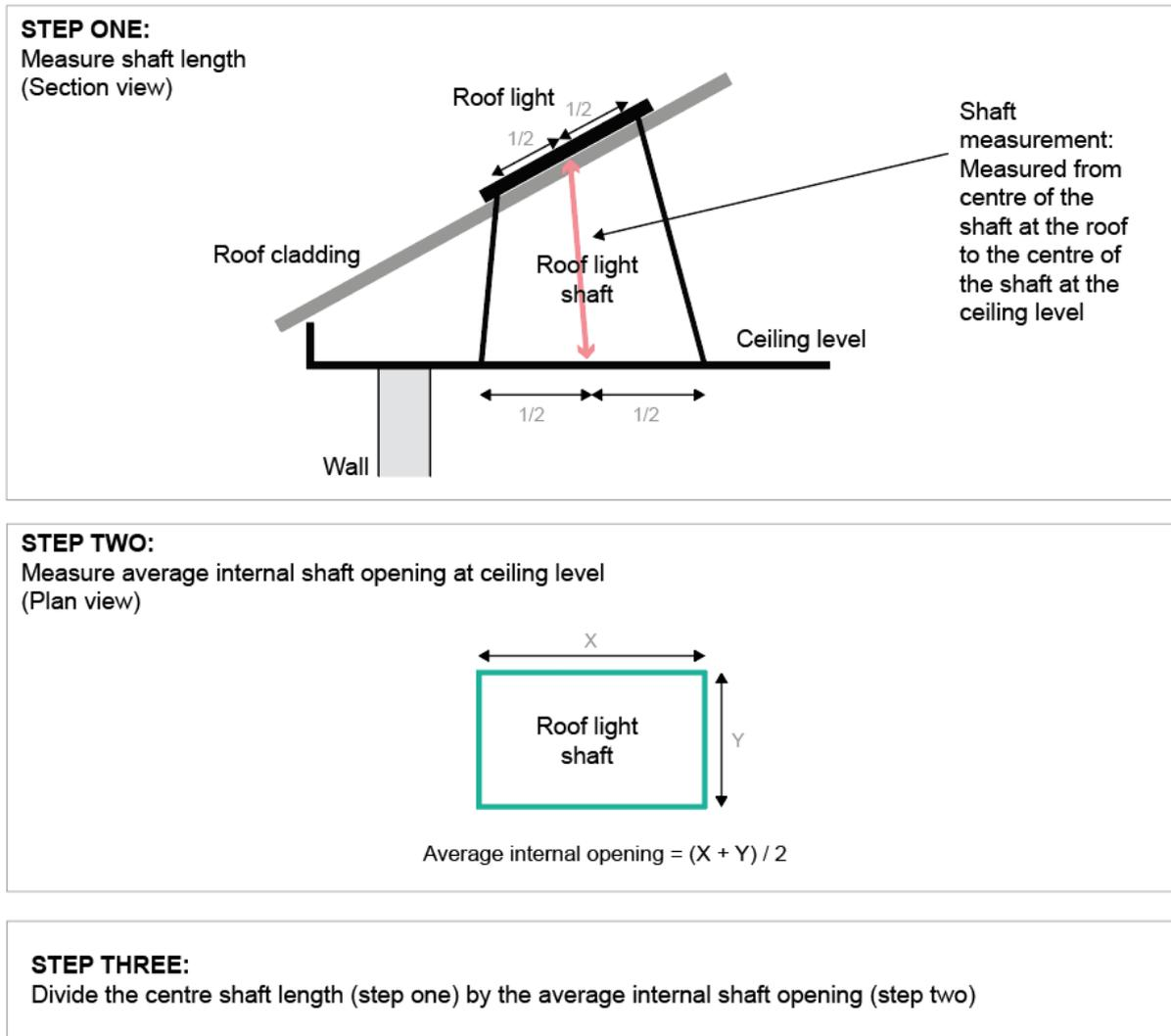
Note 2 to Table J1.4 specifies that the area of a *roof light* is equal to the area of the opening in the roof that allows light into the building. Combining the values of individual *roof lights* gives the total area of *roof lights* serving a room or space.
