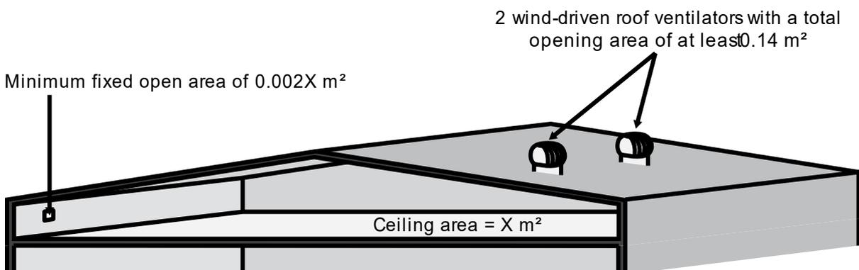
Subclause (d)(iii) specifies that a ventilated roof space can also be a roof space that is tiled and has no sarking-type material at roof level.
