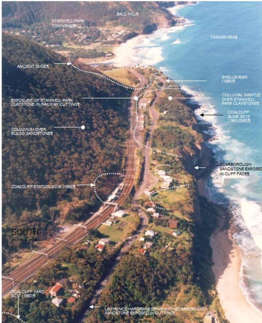
Figure 8 illustrates a generic landslide mechanism on a relatively flat platform area within steep terrain. This type of landslide is described as an earth slide with a 'stick-slip' mode, which is repeated when ground-water levels rise near the railway track. The ocean-side track "rode" upon the landslide whilst the other remained in place. The main cause of instability was high water pressure at the failure surface.
