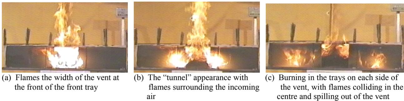
**Figure 10 Front Views of Fire in Enclosure 1500 mm Wide, 600 mm Deep and 300 mm High Vent 300 mm wide by 275 mm High**
