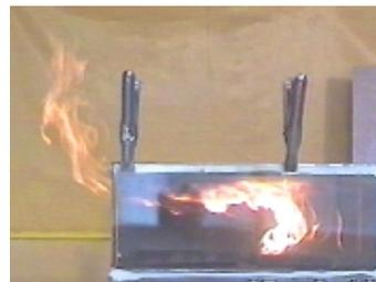
(b) Flames from front of **rear tray** after fuel in front tray exhausted - flames largely from front edge of tray, curve upward then towards vent (note obscuration of flames near vent due soot deposited on glass)
