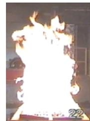
Double Row of Five Trays Per Row - arranged as for 1500 mm by 600 mm enclosure
