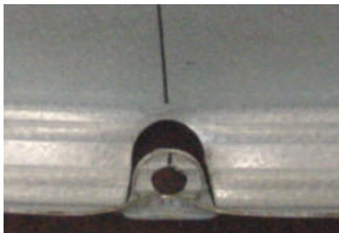
Figure 4.7 Stramit Batten failure mode
