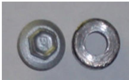
Figure 3.5 Batten screw (12 gauge) and washer used in laboratory experiments
