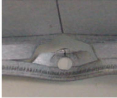
Figure 4.3 BHP batten static failure mode at the unsymmetric wider turned over edge
