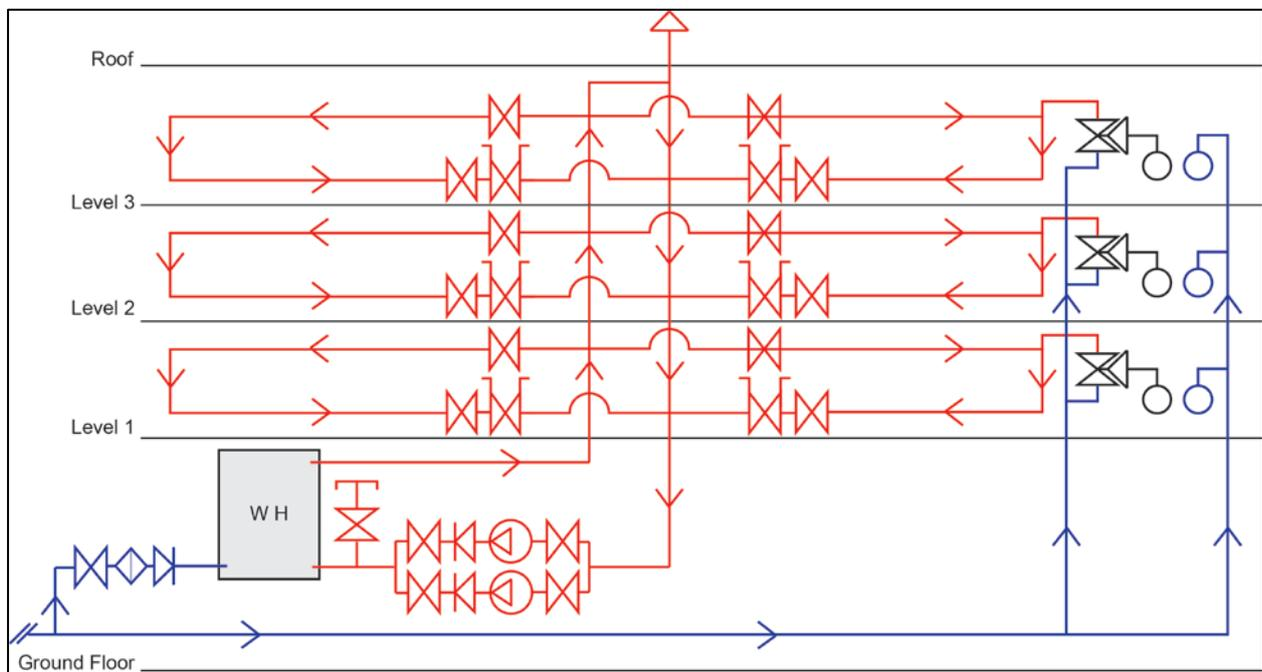
Figure 16: Typical example of a two pipe – Reverse return system.
