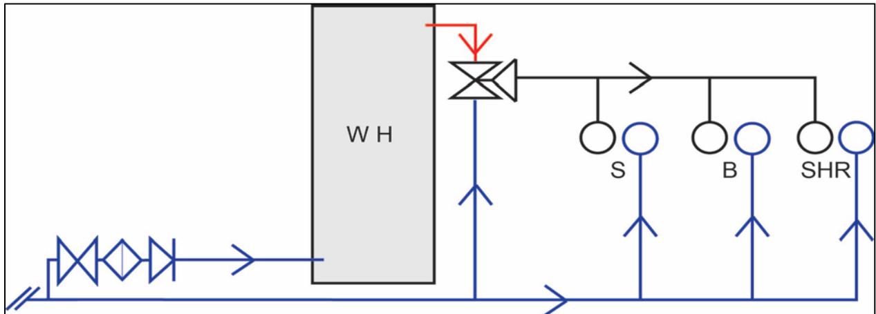
**Figure 1: Typical example of a fully tempered reticulated warm water system.**
