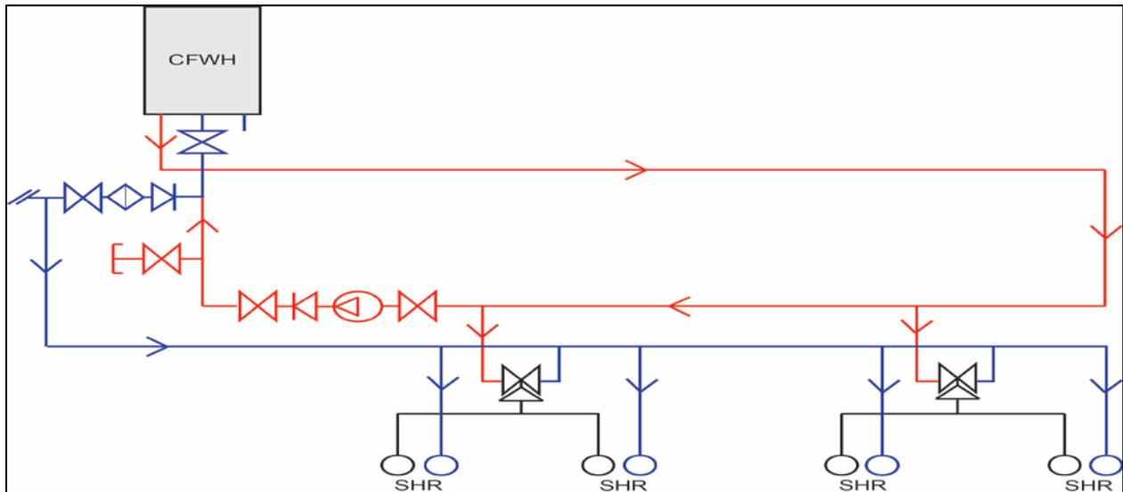
**Figure 5: Typical example of a circulating warm water system controlled by a continuous flow water heater.**
