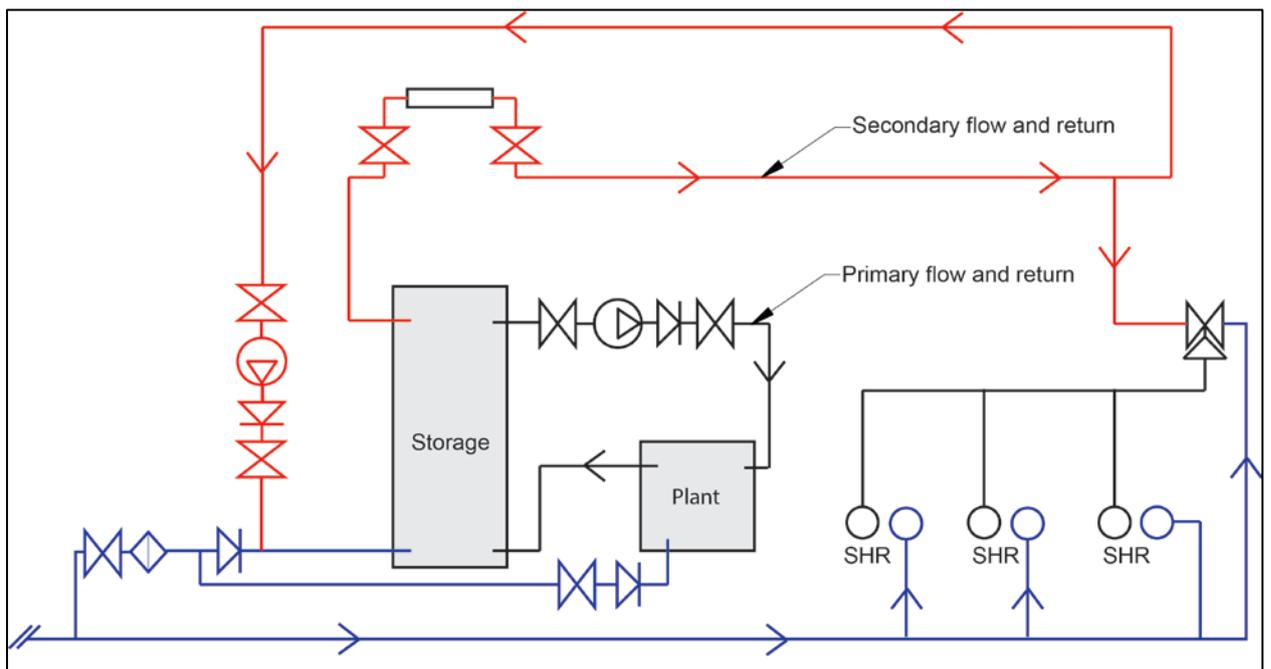
**Figure 11: Typical example of a primary flow and return system through a boiler.**
