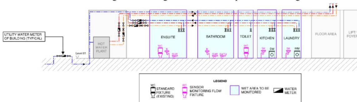
Figure 4 Single user amenities building schematic for Scenario 3 – Existing Configuration Suitable for Monitoring
