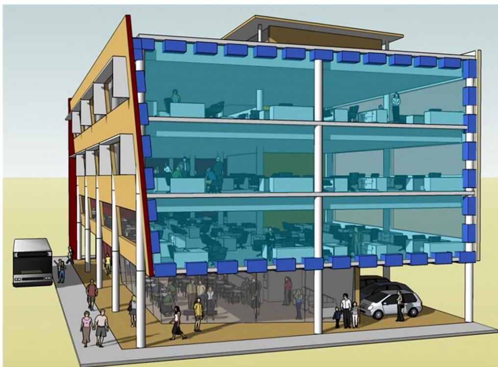
In Figure 4.2, a blue dotted line highlights the boundaries of an envelope which protects air-conditioned office interiors from warm, humid conditions outside. The differences in temperature, air pressure and water vapour dew points across the building envelope drive
