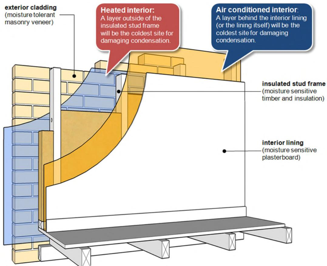
In Figure 6.6, the timber framing will be at risk of mould and decay if accumulating condensate drives up its moisture content and the insulation will lose much of its thermal resistance if it becomes waterlogged. Water in the stud frame space will easily find its way into the occupied interior of the building, damaging wall linings, trims and finishes.
