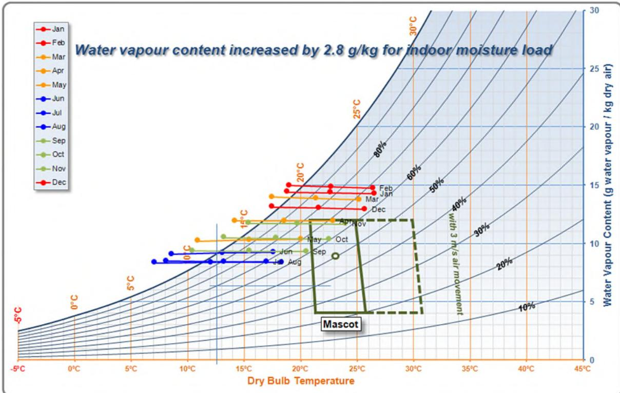
Figure D.10 Water vapour content values adjusted for indoor load – Moorabbin, Melbourne (Vic)
