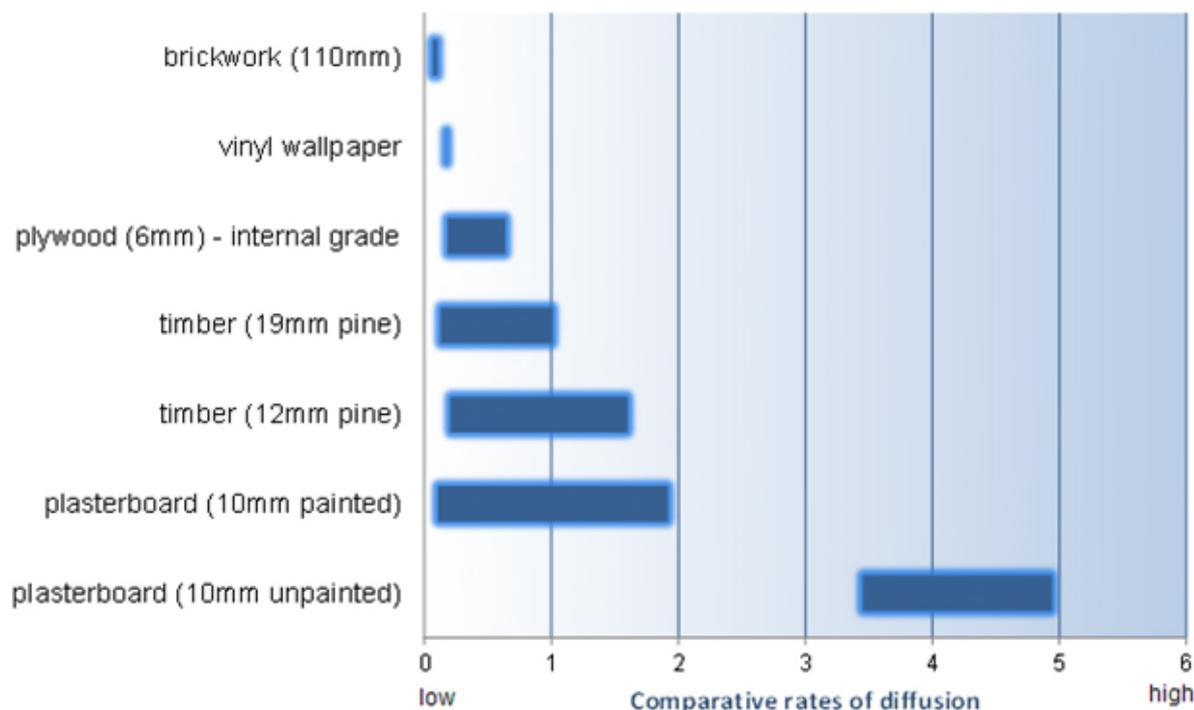
The driving force for adsorption is a difference in vapour pressure across a material or between spaces.
