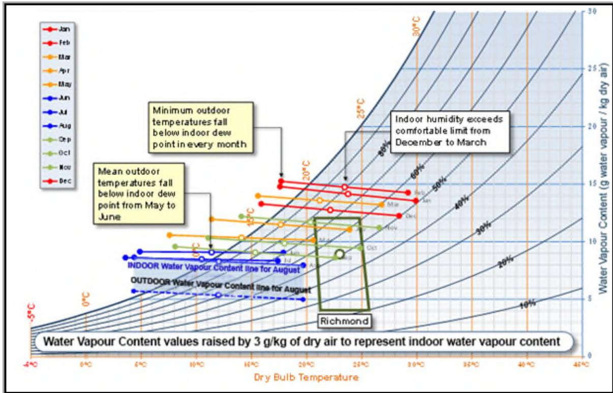
In the adjusted version of the climate analysis chart, all water vapour content values have been increased by a uniform 3 g/kg (on the vertical axis) to represent the approximate impact of the indoor water vapour load. The outdoor temperatures retain their positions on the horizontal axis.
