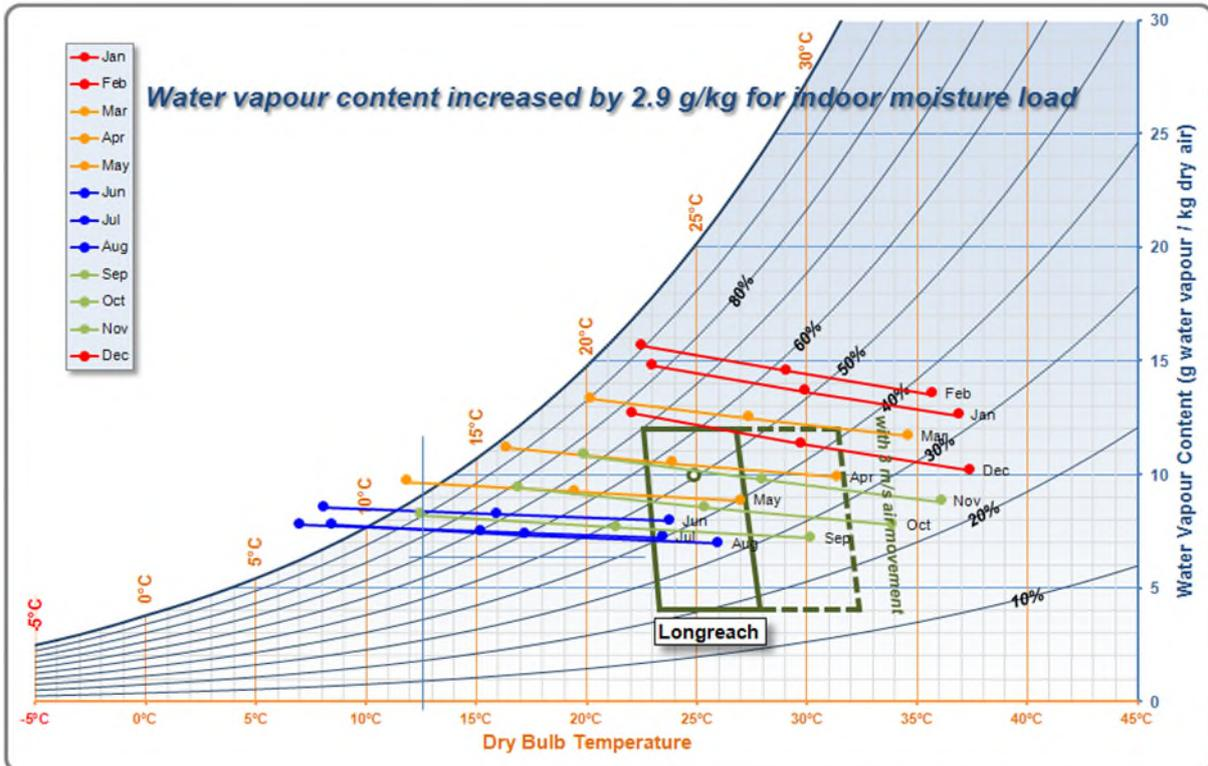
**Figure D.6 Water vapour content values adjusted for indoor load – Mildura (Vic)**
