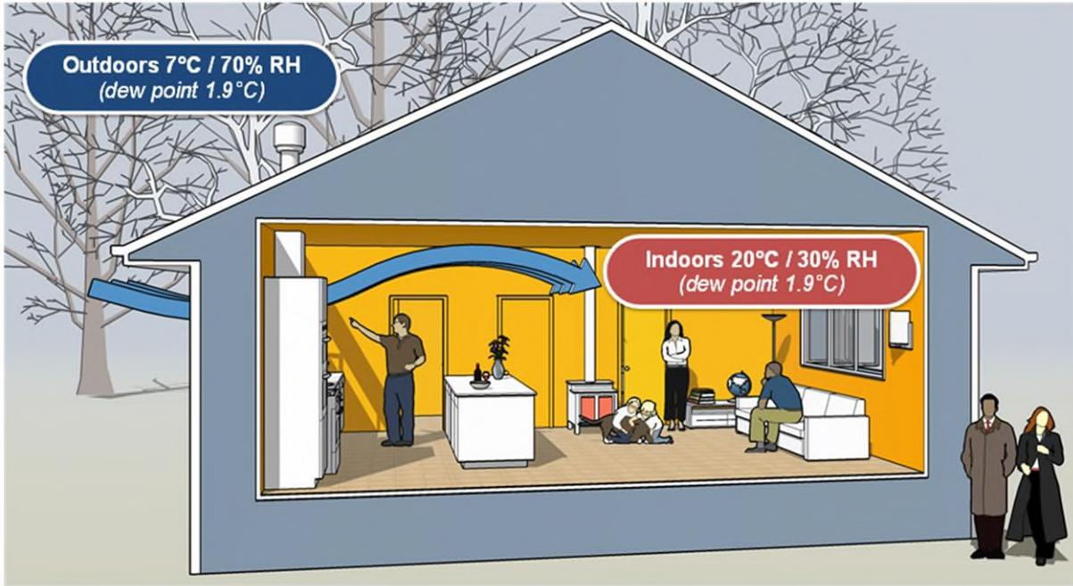
In reality, outdoor air is not the only source of water vapour that will influence the RH indoors. All occupied buildings have their own internal sources of water vapour due, in part, to the breathing of the occupants and housekeeping. How much of the added water vapour accumulates inside the building will depend also on the rate of ventilation and or extraction systems.
