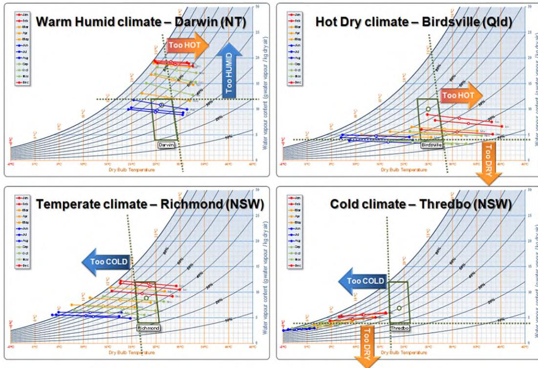
Distinct differences between the four climate types are quickly evident in Figure 3.29, where the placement, spacing, length and slope of the monthly lines are all significant. In considering what the charts suggest about the nature of the climate, and possible responses by building occupants seeking to remain comfortable, the key characteristics to look for are the:
