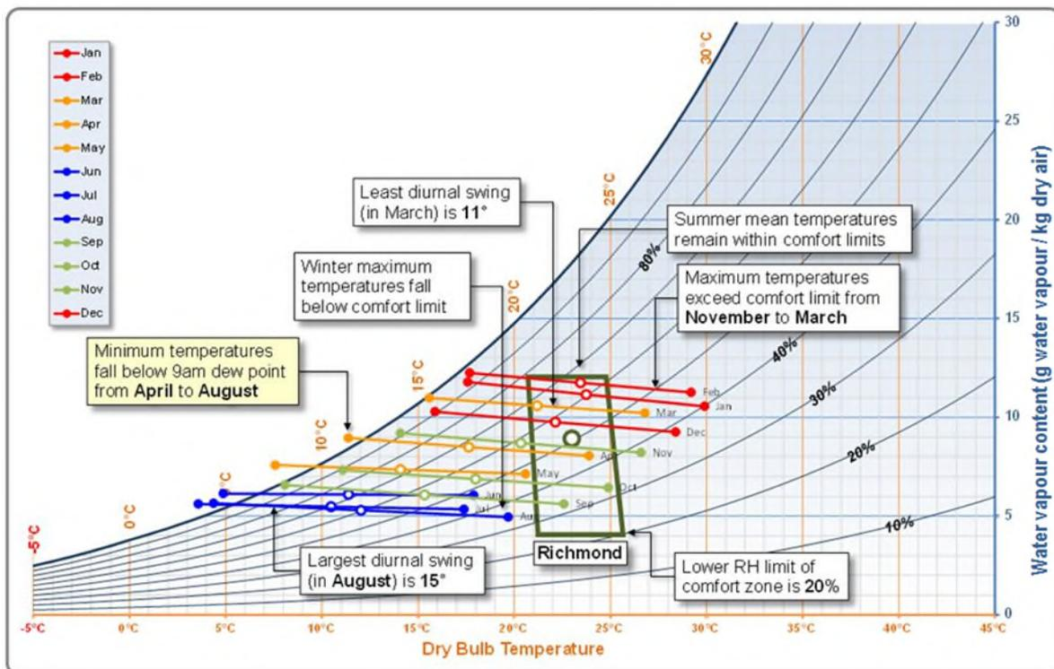
This graphical approach has the advantage of assembling information about average outdoor conditions in all 12 months in a compact format. The same approach is extended in Section 3.3.6 to address the likely impact of water vapour levels in the indoor climate.
