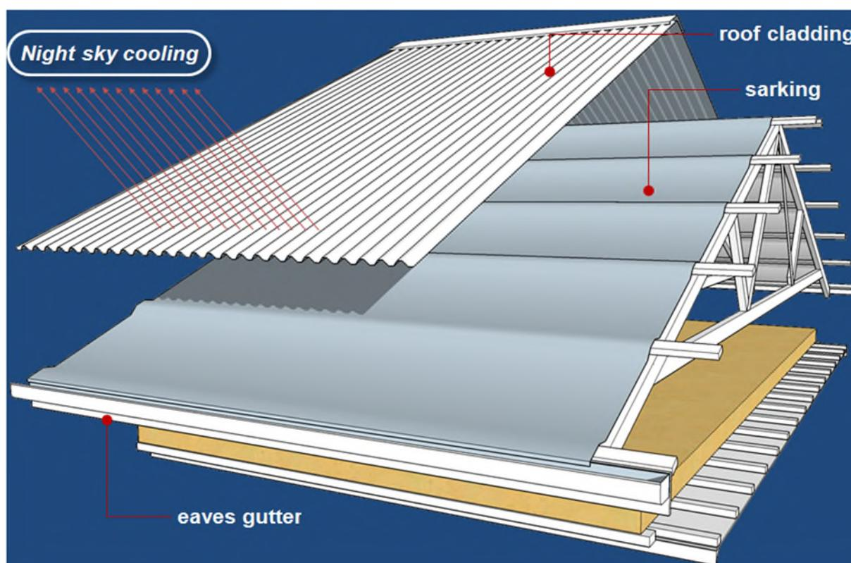
The condensation is caused by outdoor air circulating through roofing corrugations and may cool to several degrees below the outdoor air temperature. The risks depend almost entirely on the outdoor climate since only outdoor air is circulating above the sarking.
