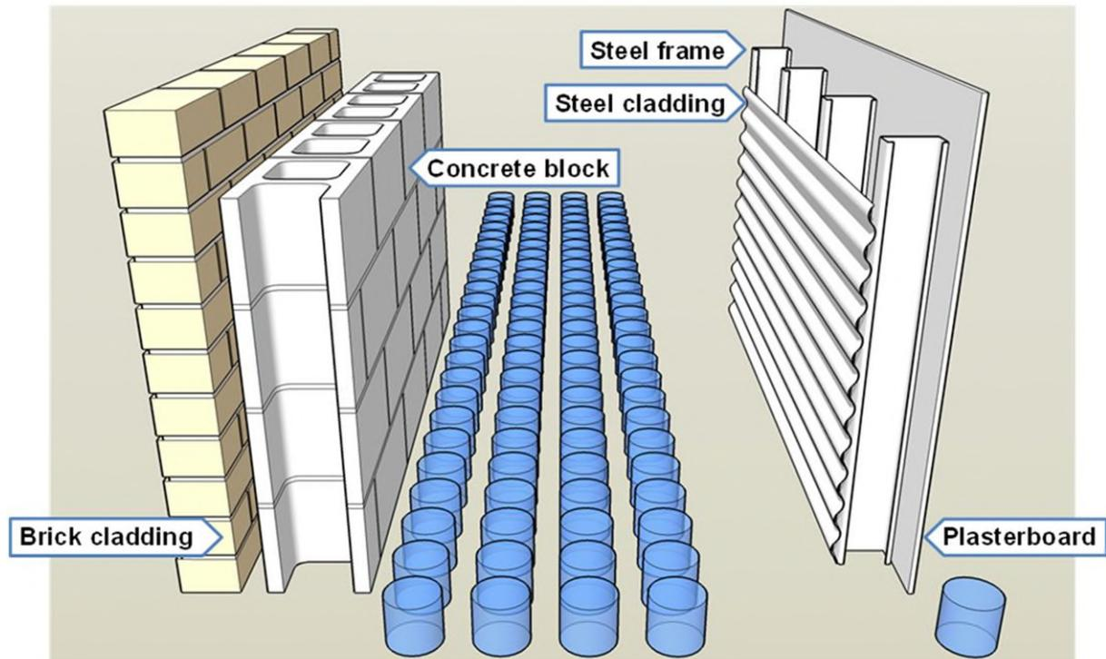
Relying on the hygric capacity of the building envelope construction is not a panacea for avoiding problems with water vapour. Some of the capacity will be needed to deal with periodic wetting by rain, surface water or rising groundwater, and some for construction moisture in the building fabric itself (e.g. water in concrete slabs or steam cured concrete blocks).
