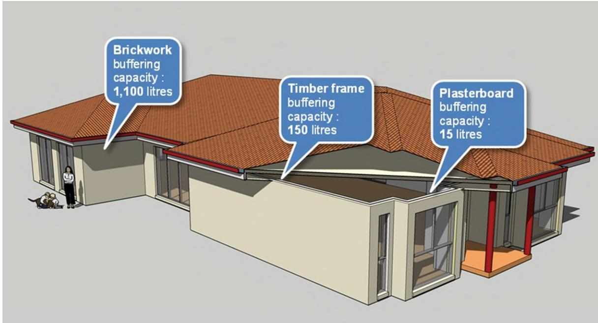
The interior plasterboard lining, in first contact with this airborne water vapour, can take up some of it by adsorption and help to stabilise RH at less problematic levels. The timber frame would increase the buffering capacity of the wall assembly more than ten times. Brick veneer for the external cladding increases it by more than 80 times (Salonvarra et al. 2007).
