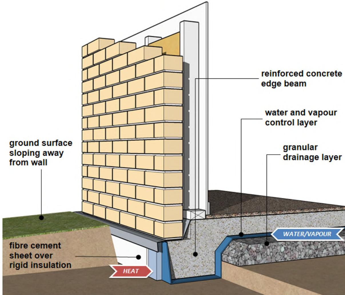
To minimise water and vapour pressure under the slab and to create a capillary break, a 100 mm granular drainage bed should be formed using coarse aggregate. The bed should discharge collected water clear of the building base and be vented to the atmosphere to assist drying.
