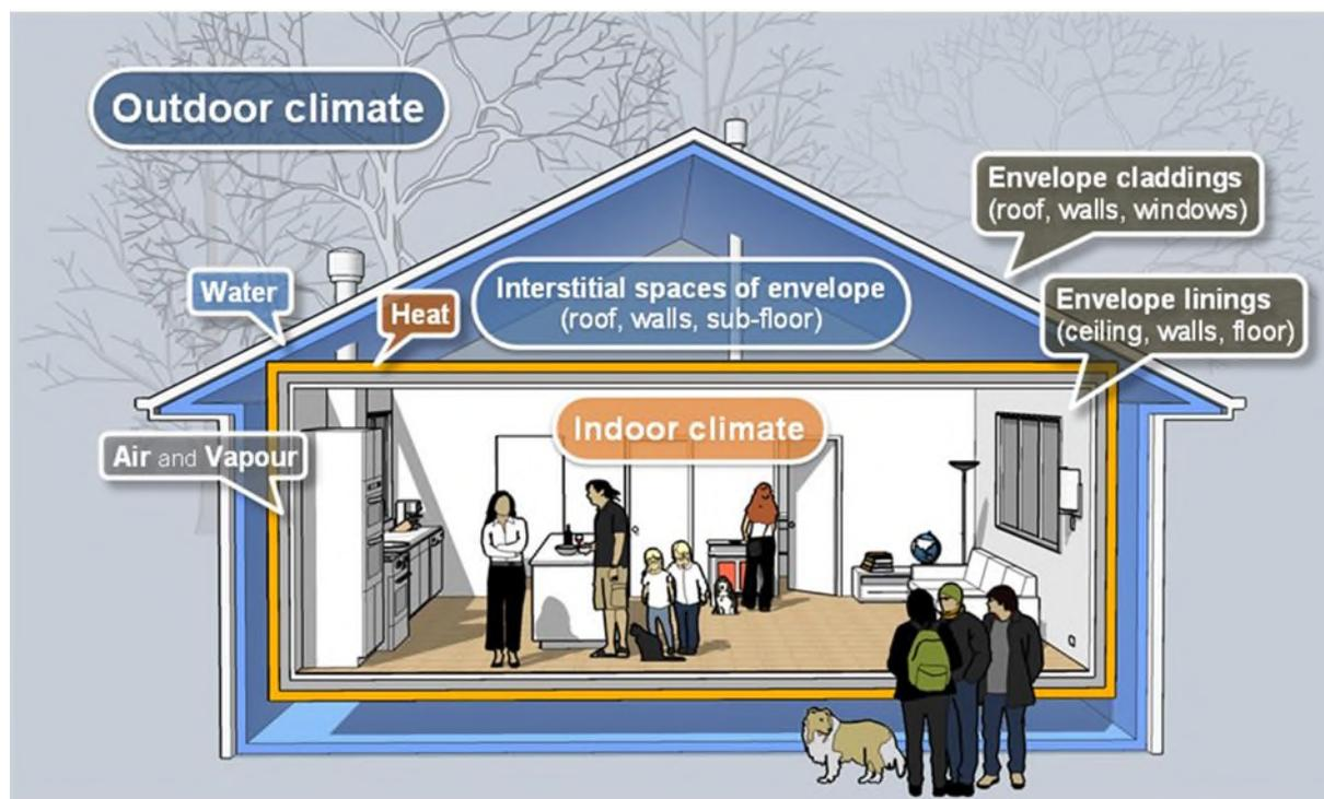
The control layers need to be continuous on all sides but the function can pass from material to material in the building fabric provided each can do the job and appropriate overlap or joining occurs at every transition.
