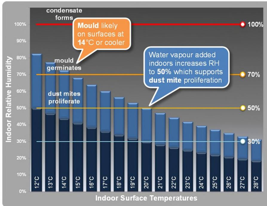
The psychrometric chart in Figure 3.10 illustrates RH falling as temperatures increase but the risks for buildings stem from the rising RH which develops as temperatures fall. The temperature fall can be due to a cold external environment or cooling in an air-conditioned interior. As suggested by Figure 3.12, unwelcome effects can emerge before RH reaches 100% and the dew point when condensation begins.
