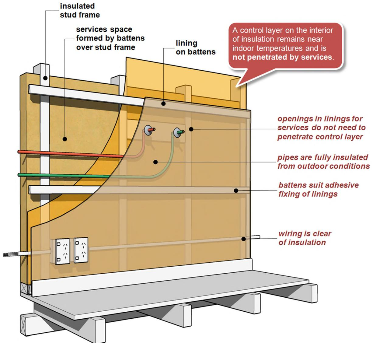
Emphasising the importance of effective air control, the British Standard BS 5250:2011+A1:2016, Annex G, advises that a dedicated space for the installation of services should be formed behind interior surface finishes or linings. This will allow an air control layer to be formed on the interior side of wall insulation without penetrations for services, as illustrated in Figure 4.12.
