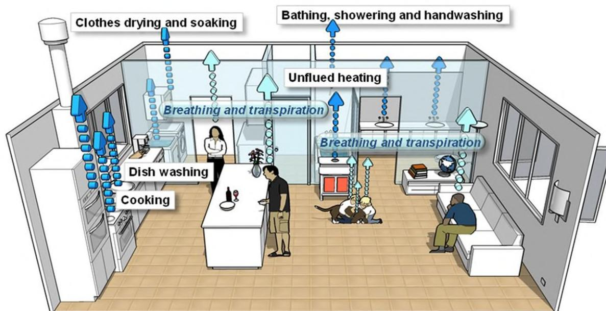
In a residential room where both temperature and humidity are closely controlled, the amount of circulating water vapour might vary from under 0.5% of the moist air mass in a cold climate up to about 1% in a warm humid climate. While this may not seem like a lot of water vapour, only a small amount of extra water vapour is needed to increase the risk of condensation related problems.
