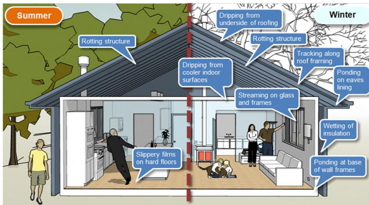
Liquid water responds to gravity to accumulate, run, drip and pond, possibly causing nuisance or damage in places away from the first point of condensation. When water appears where it is not wanted in a building, it is often taken as evidence of a leak rather than condensation, and a search for the cause begins in the wrong places. One strong indication that a phantom leak could be at work is when water emerges in the absence of significant rainfall.
