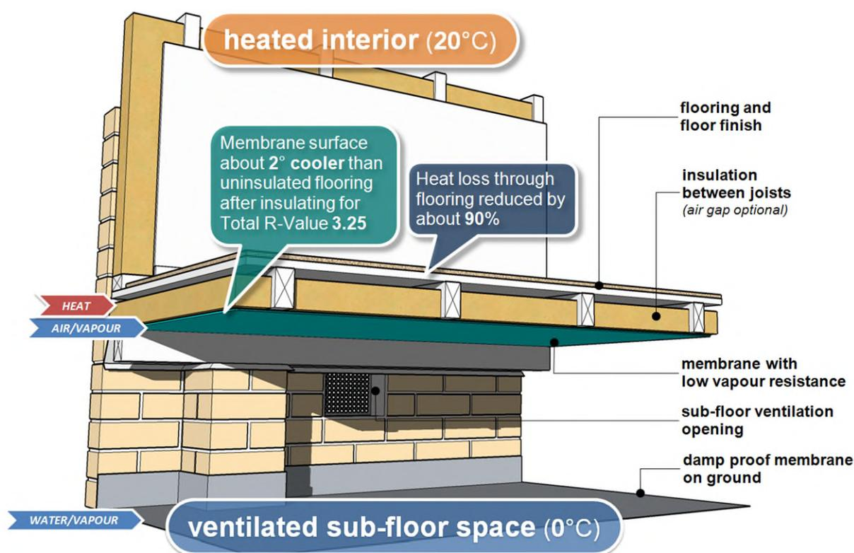
The suspended timber framed floor over a ventilated sub-floor space has insulation installed between the joists and supported on a membrane with low water vapour resistance. This arrangement follows an example in the British Standard BS 5250:2011+A1:2016 "Code of practice for control of condensation in buildings" (Figure F.6). It relies on ventilation to keep the dew point in that space low and close to the outdoor level.
