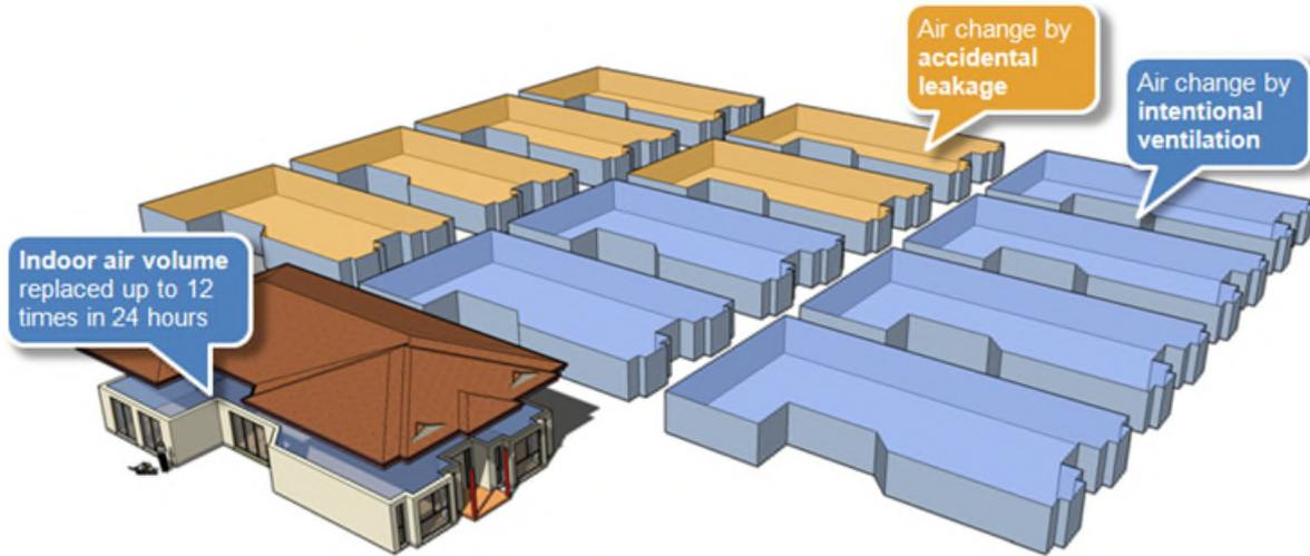
Since outdoor air supply cannot safely be reduced below an essential minimum, water vapour brought in with outdoor air will limit attempts to lower water vapour levels indoors (unless an air conditioning system with substantial dehumidifying capacity is involved). Once that lower limit is reached, RH must be managed by raising the indoor temperature, using active or passive heating. The benefits of controllable heating are illustrated in Figure 3.4.
