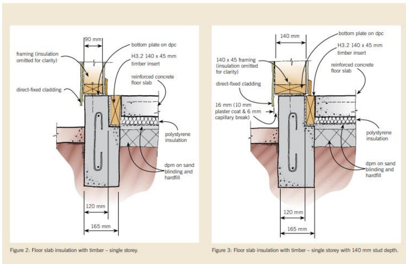
Figure 17. External wall thickness definitions as defined by Ian Cox-Smith (BRANZ) in Build Magazine (page 105, BUILD June/July 2007 – accessed: <https://www.buildmagazine.org.nz/assets/PDF/B100-103-InsulateSlab.pdf>)
