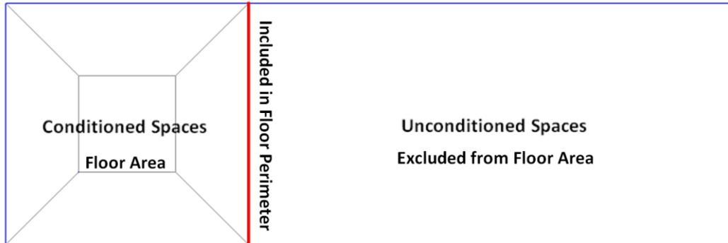
Figure 19 Floor Area and Floor Perimeter for Conditioned Spaces connected to Unconditioned Spaces
