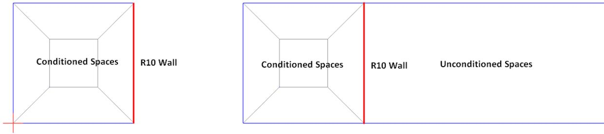
**Figure 14 Models to Test the Heat Transfer through the Floor in a Conditioned Space and an Unconditioned Space**
