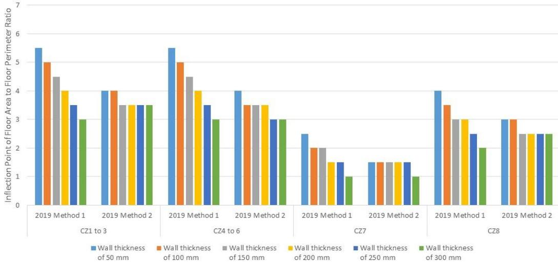
Figure 4 Inflection Points of Floor Area to Floor Perimeter Ratio (Soil Type – Clay or Silt)
