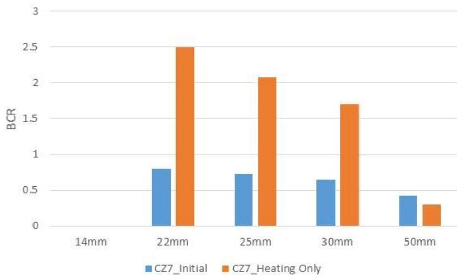
Figure 12 BCR Results for Motel Models in CZ7 (Sensitivity Analysis for Edge Insulation)
