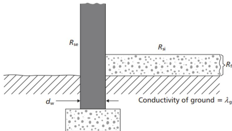
$$\text{Total equivalent thickness of floor: } d_{ef} = d_w + \lambda_g (R_{si} + R_f + R_{se})$$
