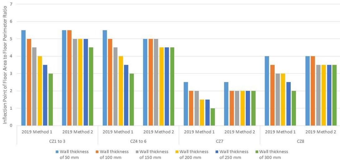
Figure 5 Inflection Points of Floor Area to Floor Perimeter Ratio (Soil Type – Sand or Gravel)
