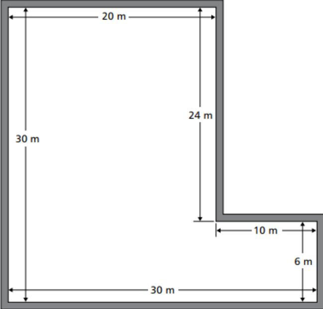
Figure 20 Example 3.4 in CIBSE Section 3.5 indicating the floor area and the floor perimeter is calculated from the interior surface of the external wall surrounding the floor
