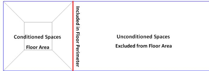
Figure 1 Floor Area and Floor Perimeter for Conditioned Spaces connected to Unconditioned Spaces
