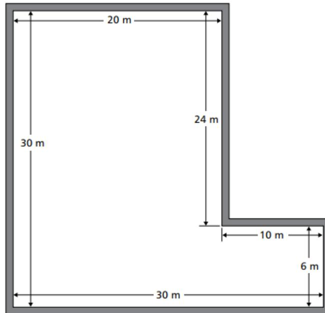
Figure 16 Example 3.4 in CIBSE Section J3.5 indicating the floor area and the floor perimeter is calculated from calculated from the interior surface of the external wall surrounding the floor
