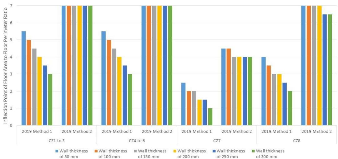
Figure 6 Inflection Points of Floor Area to Floor Perimeter Ratio (Soil Type – Homogeneous Rock)
