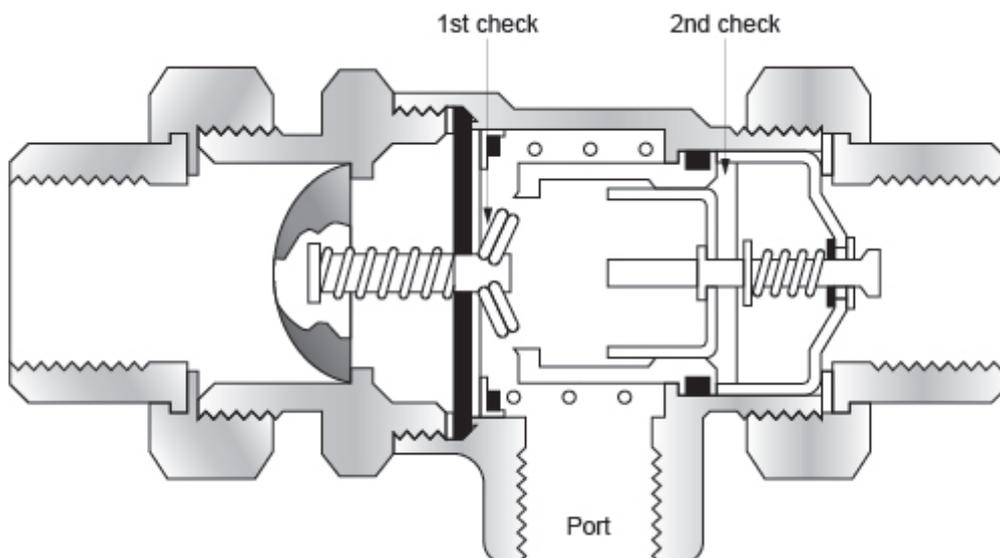
Pressure within a water service keeps the vent port closed, but zero supply pressure or backsiphonage will open the inner chamber to atmosphere. With this device, extra protection is gained through the capability of venting to atmosphere.
