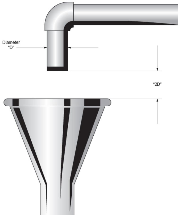
An AG can cause a corresponding loss of pressure to downstream outlets. However, they are an extremely effective backflow preventer when used to prevent backsiphonage and backpressure conditions. Consequently, AGs are primarily used at end of line services where reservoirs or storage tanks are desired.
