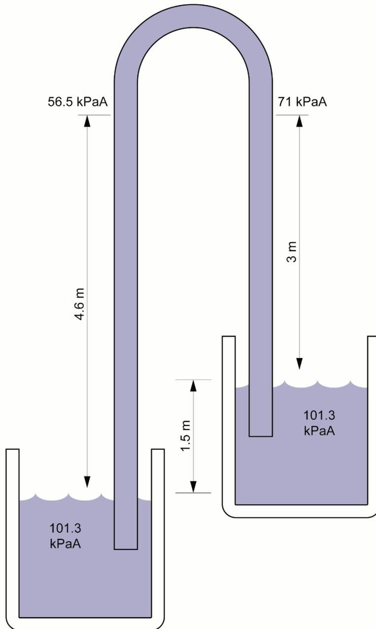
Figure C.7 shows how this siphon principle can be hazardous in a plumbing system. If the supply valve is closed, the pressure in the line supplying the tap is less than the pressure in the supply line to the bathtub. Therefore, flow will occur through siphonage, from the bathtub to the open tap.
