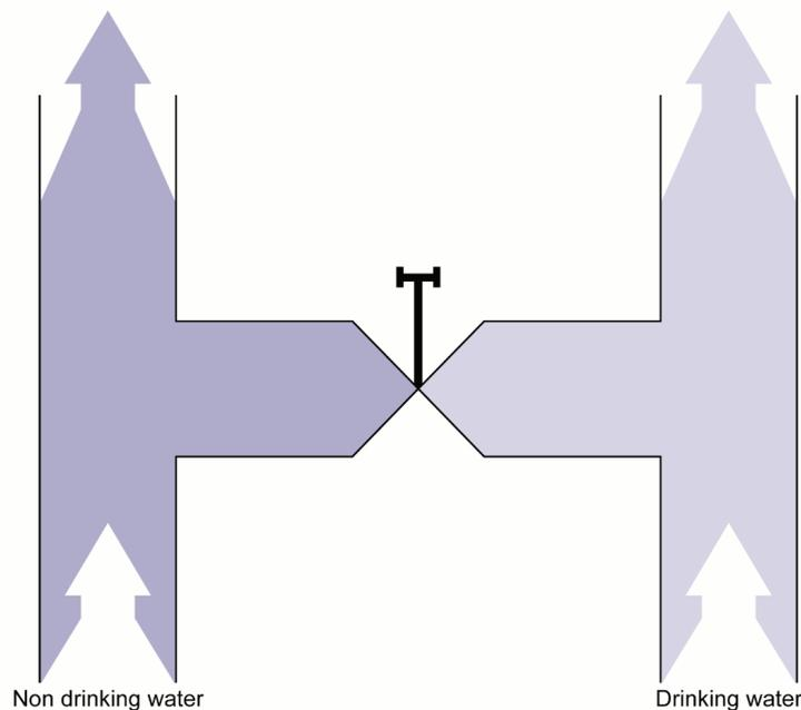
**Figure C.11 Valved connection between water supply and sanitary drainage system**
