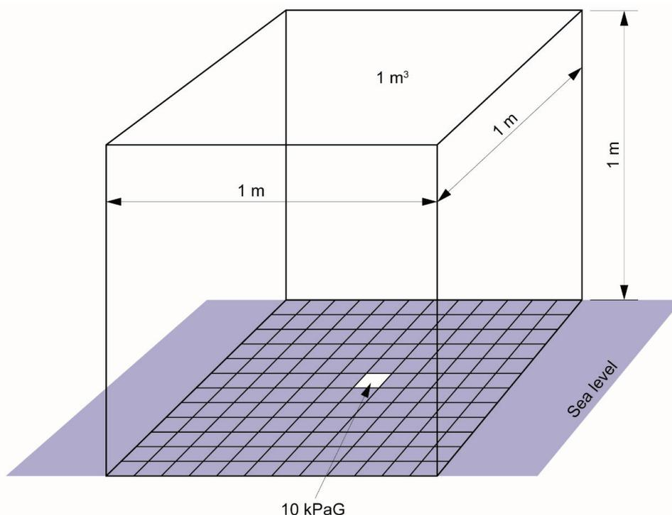
Suppose another cubic metre of water was placed directly on top of the first, see Figure C.2. The pressure on the top surface of the first cube which was originally atmospheric, or 0 kPaG, would now be 10 kPaG because of the superimposed cubic metre of water. The pressure on the base of the first cube would also be increased by the same amount to 20 kPaG, or 2 times the original pressure.
