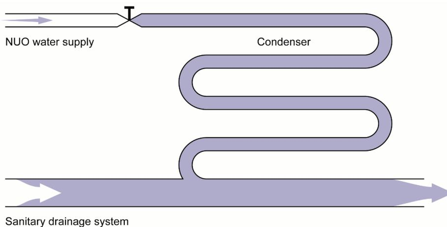
Submerged inlets are found on many common plumbing fixtures and are sometimes necessary features of the fixtures if they are to function properly. Examples of this type of design are bottom filling vats or vessels, water closets, flushing rim slop sinks, and dental cuspidors.
