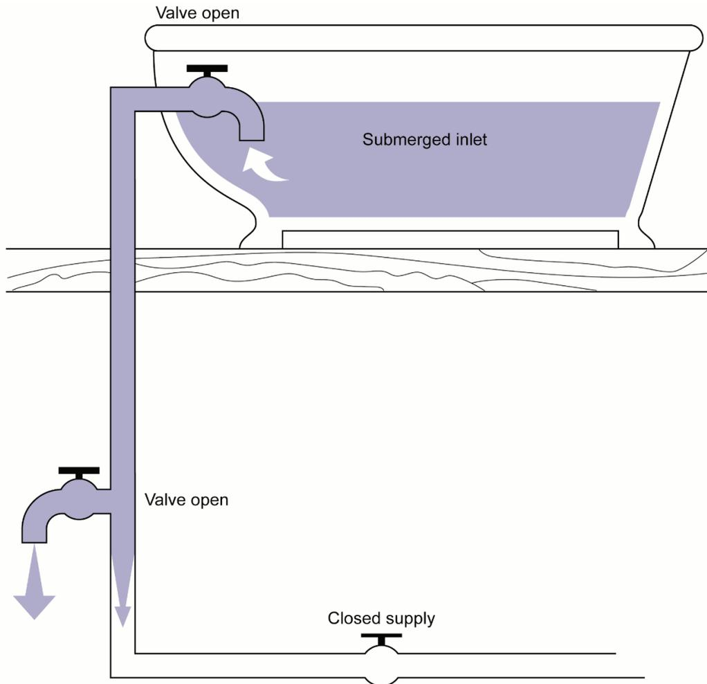
The siphon actions cited have been produced by reduced pressures due to a difference in the water levels at 2 separated points within a continuous fluid system.
