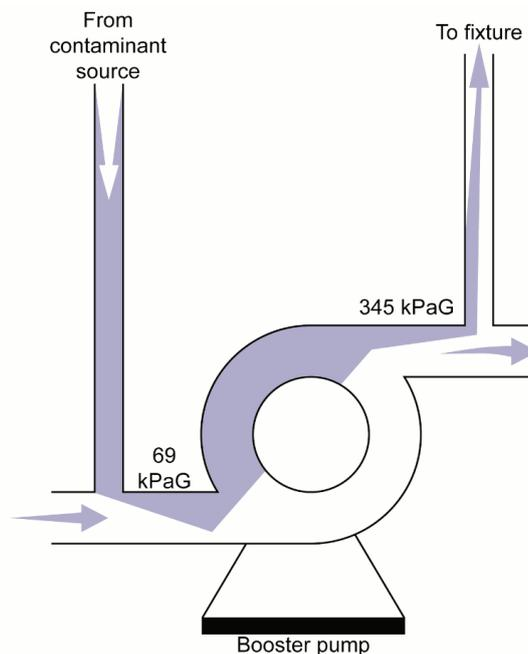
The previous discussion has described some ways negative pressures may be created and which frequently occur to produce backsiphonage. In addition to the negative pressure or reversed force necessary to cause backsiphonage and backflow, there must also be the cross-connection or connecting link between the water supply and the source of contamination. Two basic types of connections may be created in piping systems. These are the solid pipe with valve connection and the submerged inlet.
