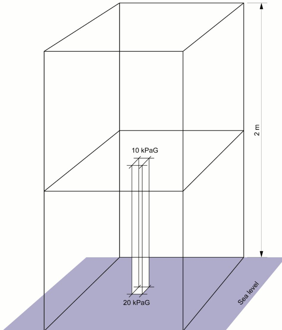
If this process was repeated with a third cubic metre of water, the pressures at the base of each cube would be 30 kPaG, 20 kPaG, and 10 kPaG, respectively. It is evident that pressure varies with depth below a free water surface. In general, each metre of elevation change within a liquid, changes the pressure by an amount equal to the weight-per-unit area of 1 metre of the liquid. The rate of increase for water is 10 kPaG per metre of depth.
