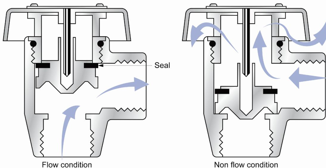
AVBs must be installed vertically and must not have any shutoffs downstream of the device. They must be installed at least 150 mm higher than the highest downstream outlet. Figure 6.4 shows the typical installation of an AVB. Note that no shutoff valve is installed downstream of the device that would otherwise keep the AVB under continuous pressure.
