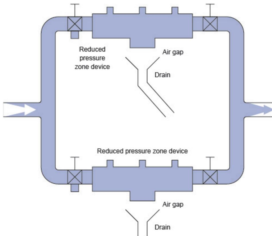
Although Figure 7.1 depicts a protected bypass using RPZDs, other devices can also be installed, provided that an isolation valve is installed at the end of each device to enable it to be isolated from the water supply and removed if found to be defective. Always ensure the 2 devices are of the same hazard protection level.
