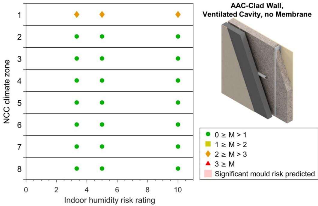
Figure 4-17: Maximum 10-year mould index ( $M$ ) simulated in walls clad with autoclaved aerated concrete (AAC), with ventilated cavities and no membrane.
