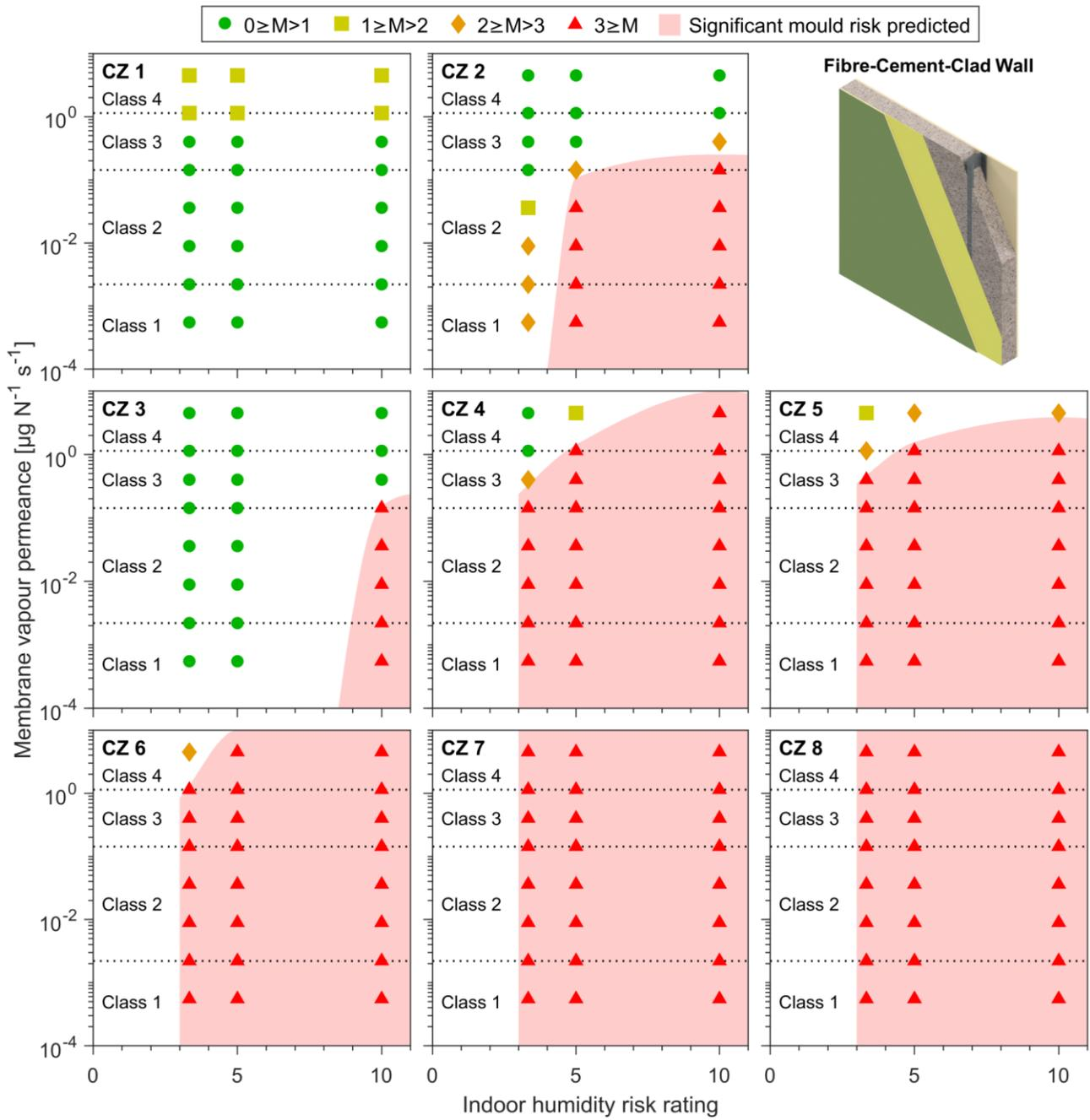
Figure 4-9: Maximum 10-year mould index ( $M$ ) simulated in fibre-cement-clad walls.
