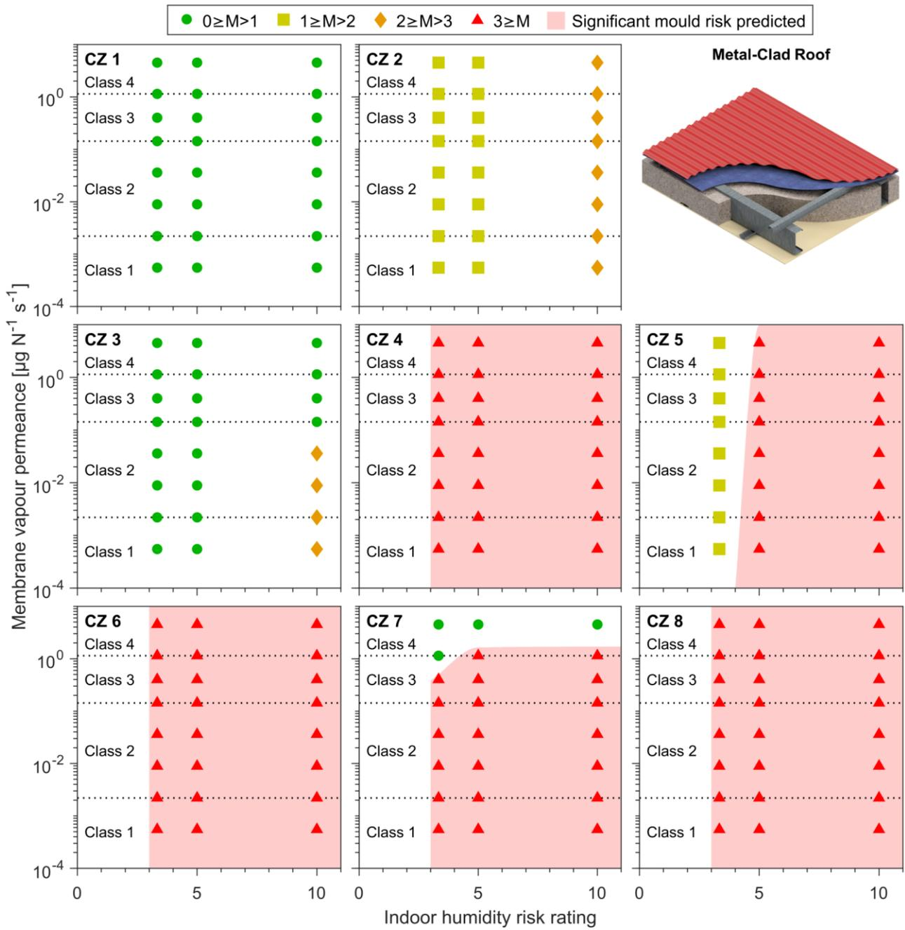
Figure 4-22: Maximum 10-year mould index ( $M$ ) simulated in metal-clad roofs.
