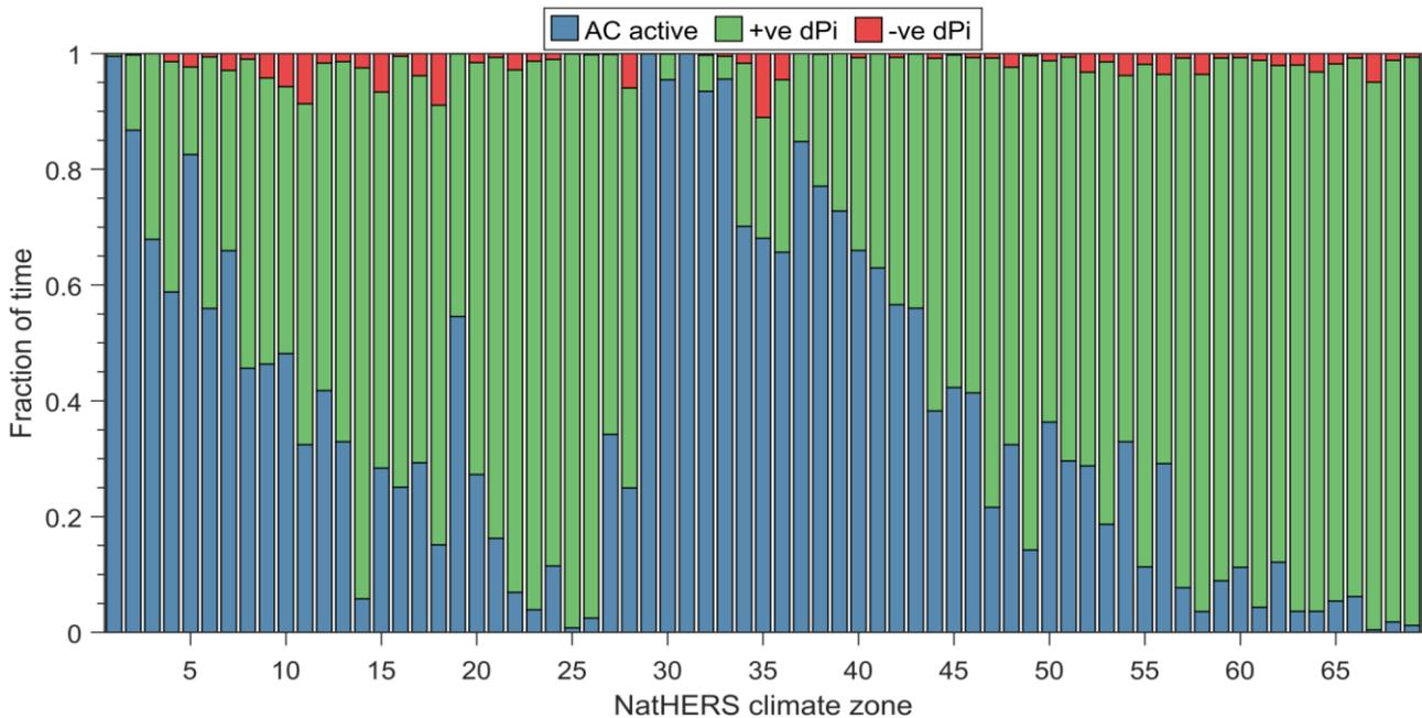
*Figure 6-5: Distribution of indoor humidity conditions generated using the standard AIRAH DA07 method (with 70 % relative humidity cap) for the 69 NatHERS climate zones. Each bar represents the distribution of hours through the course of a year in which either: air-conditioning (AC) is active, AC is not active and  $dp_i$  is positive (i.e. driving diffusion from indoors outwards), and AC is not active and  $dp_i$  is negative.*
