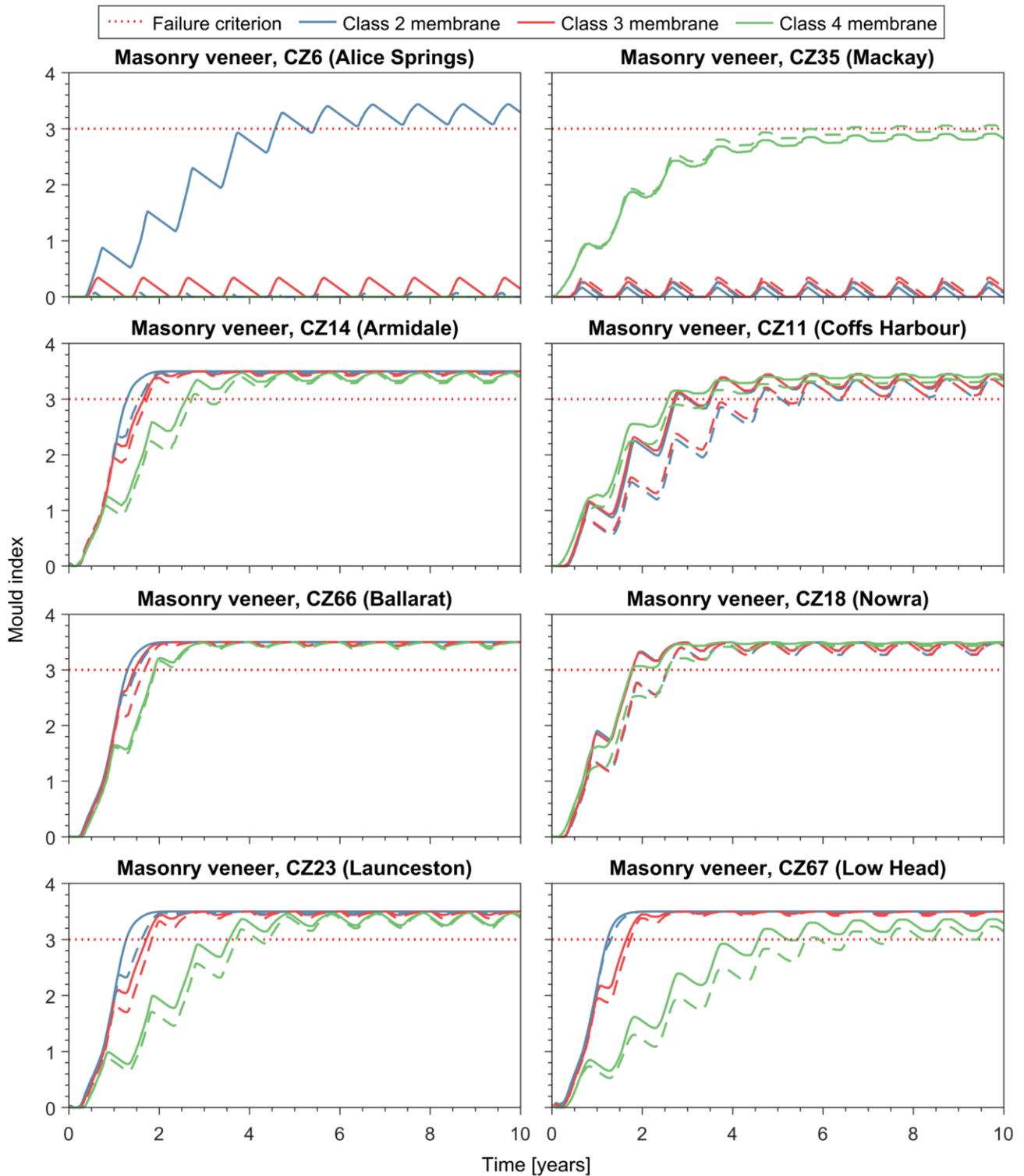
Figure 6-8: Comparison of mould index time series simulated with indoor humidity conditions generated using the standard AIRAH DA07 intermediate method with 70 % relative humidity cap (solid lines), and those generated using the hybrid method (broken lines). Results in this figure are from simulations of the masonry veneer wall with three different membranes in the 8 selected locations.
