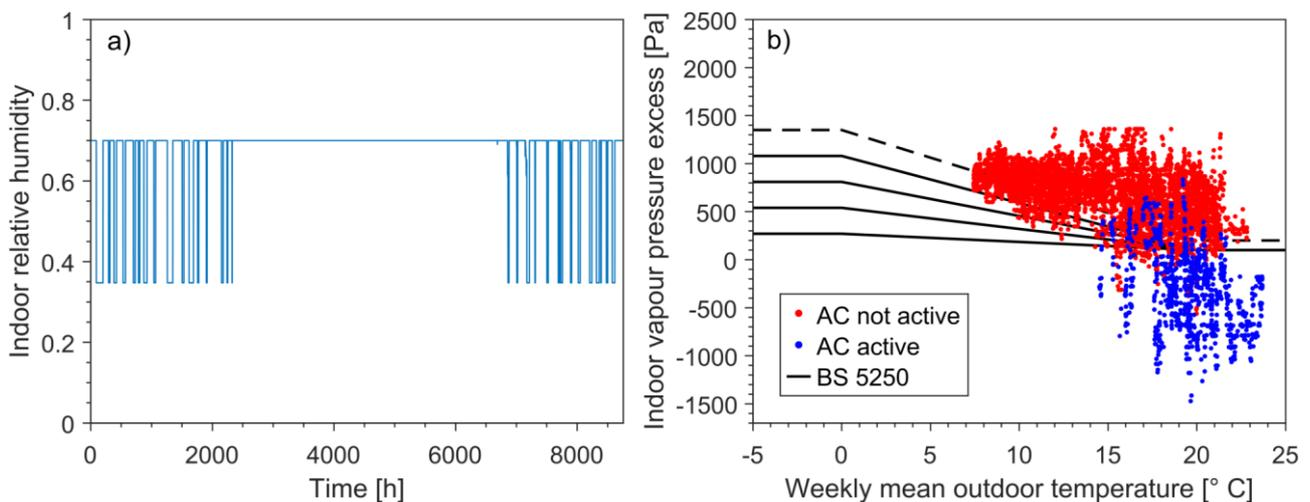
Figure 6-1: Indoor humidity boundary conditions determined for Melbourne following the AIRAH DA07 intermediate method with the standard 70 % relative humidity cap: a) relative humidity time series, b) indoor vapour pressure excess at each timestep compared to the indoor climate classes defined in BS 5250. Input assumptions include a floor area of 90 m<sup>2</sup>, ceiling height of 2.4 m, infiltration rate of 0.2 ACH, and 3 bedrooms (4 occupants).
