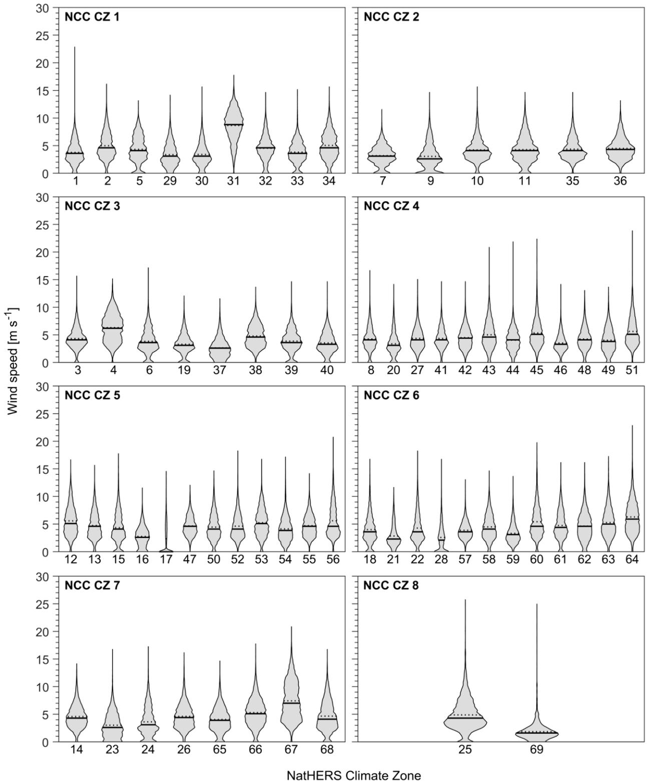
Figure 0-6: Distribution of mean hourly wind speed in the climate files used to represent each of the NatHERS Climate Zones.
