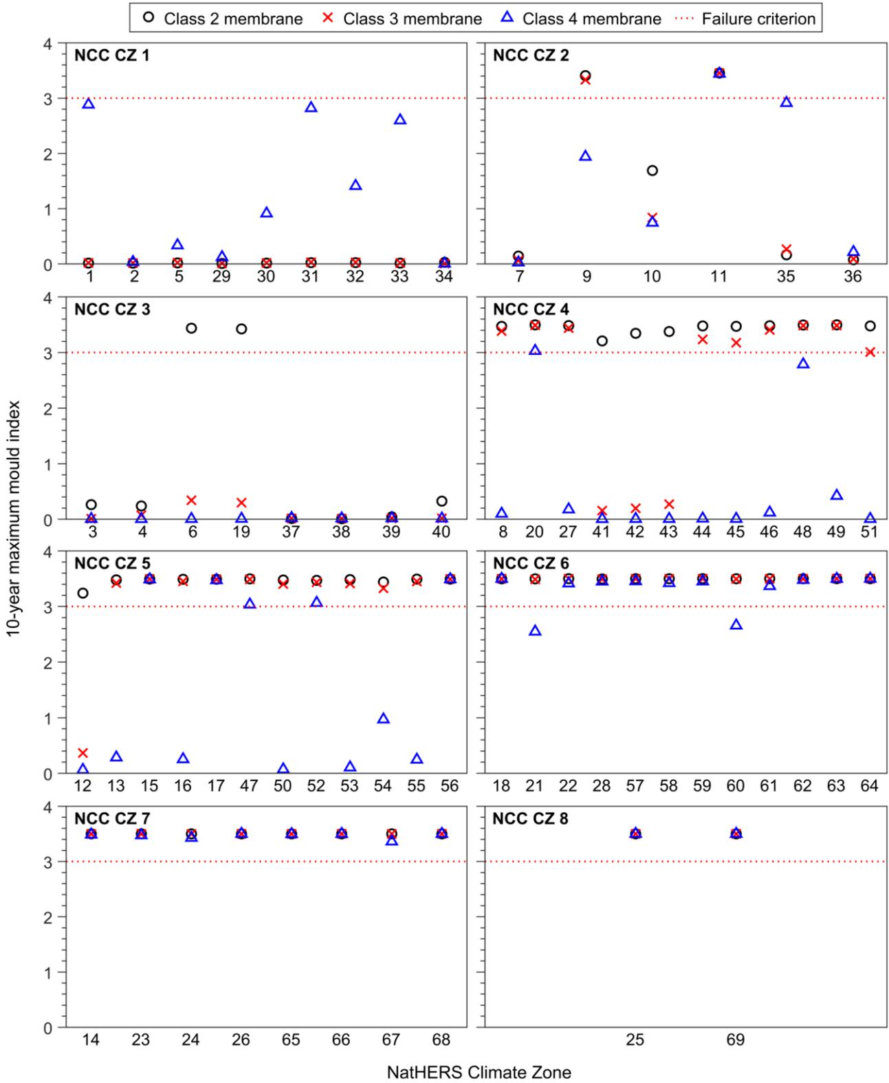
Figure 5-1: Results from WUFI simulations of the masonry veneer wall in all 69 NatHERS climate zones, with three different pliable membranes.
