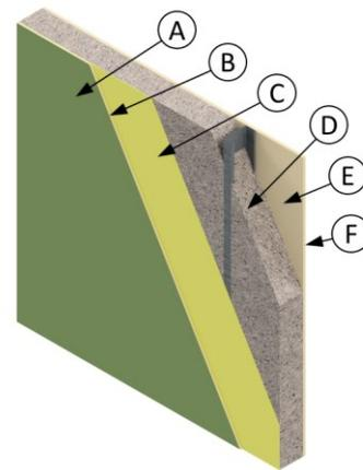
Figure 2-6: Fibre-cement-clad wall.
