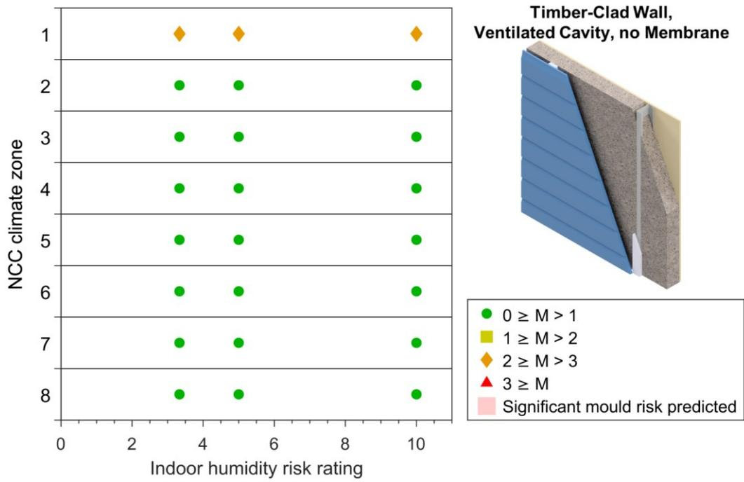
Figure 4-8: Maximum 10-year mould index ( $M$ ) simulated in timber-clad walls with ventilated cavities and no pliable membrane.
