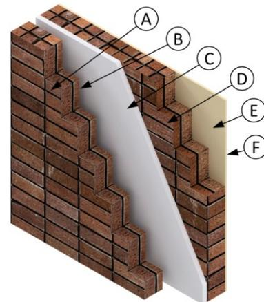
Figure 2-2: Cavity masonry wall.
