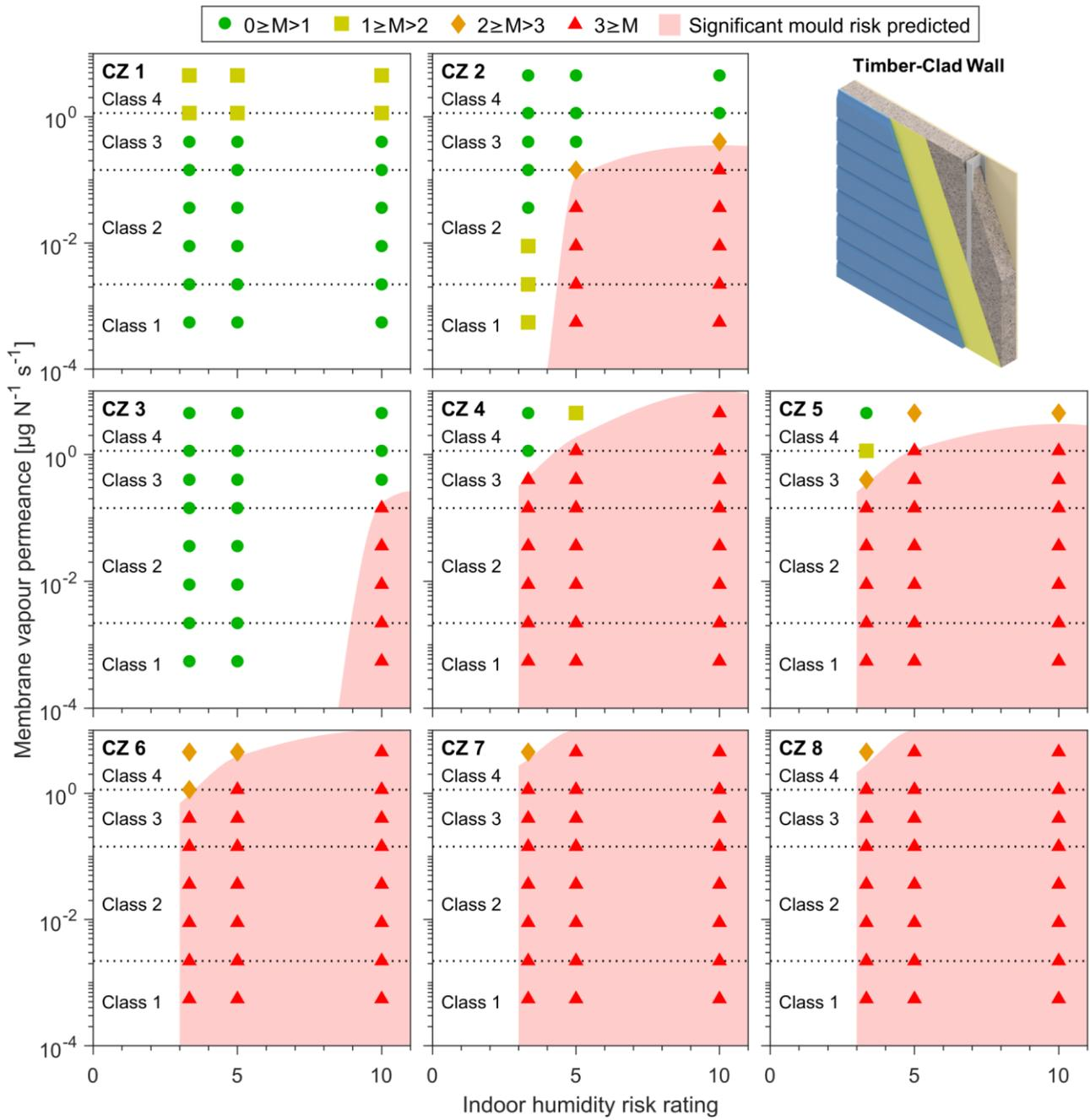
Figure 4-6: Maximum 10-year mould index ( $M$ ) simulated in timber-clad walls.
