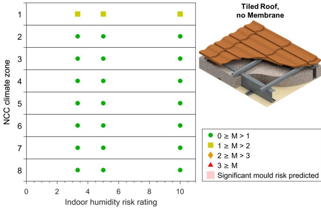
Figure 4-20: Maximum 10-year mould index ( $M$ ) simulated in tiled roofs with no membrane.
