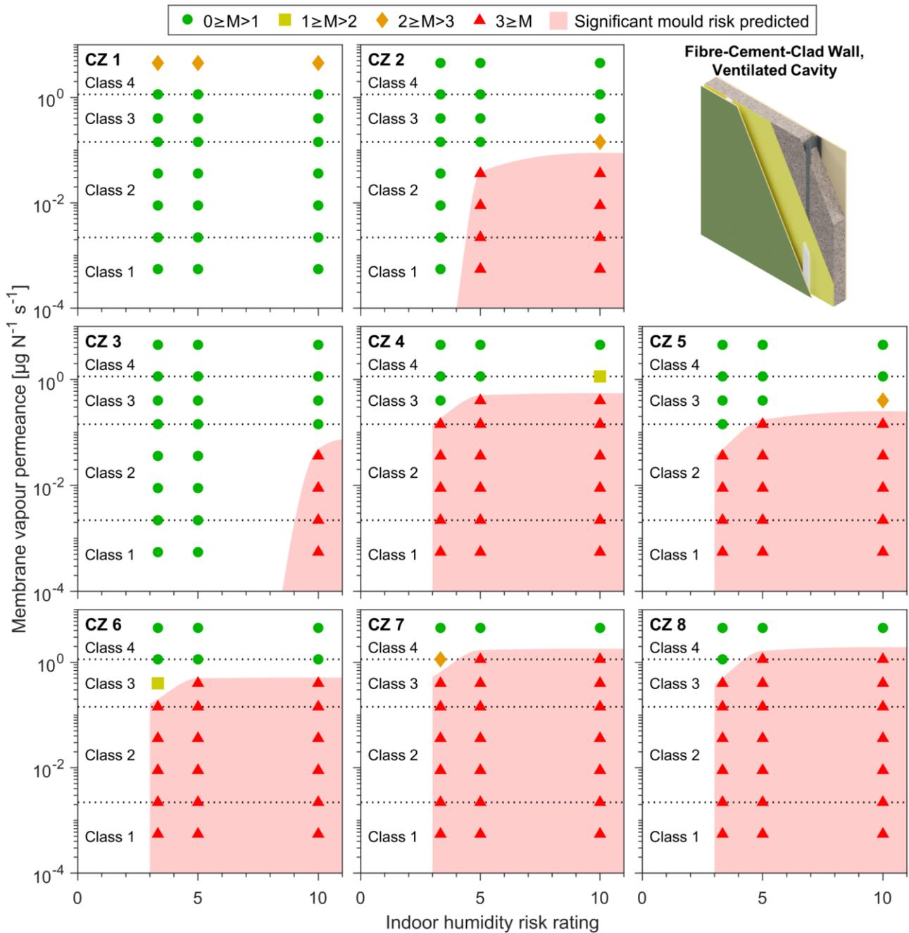
Figure 4-10: Maximum 10-year mould index ( $M$ ) simulated in fibre-cement-clad walls with ventilated cavities.
