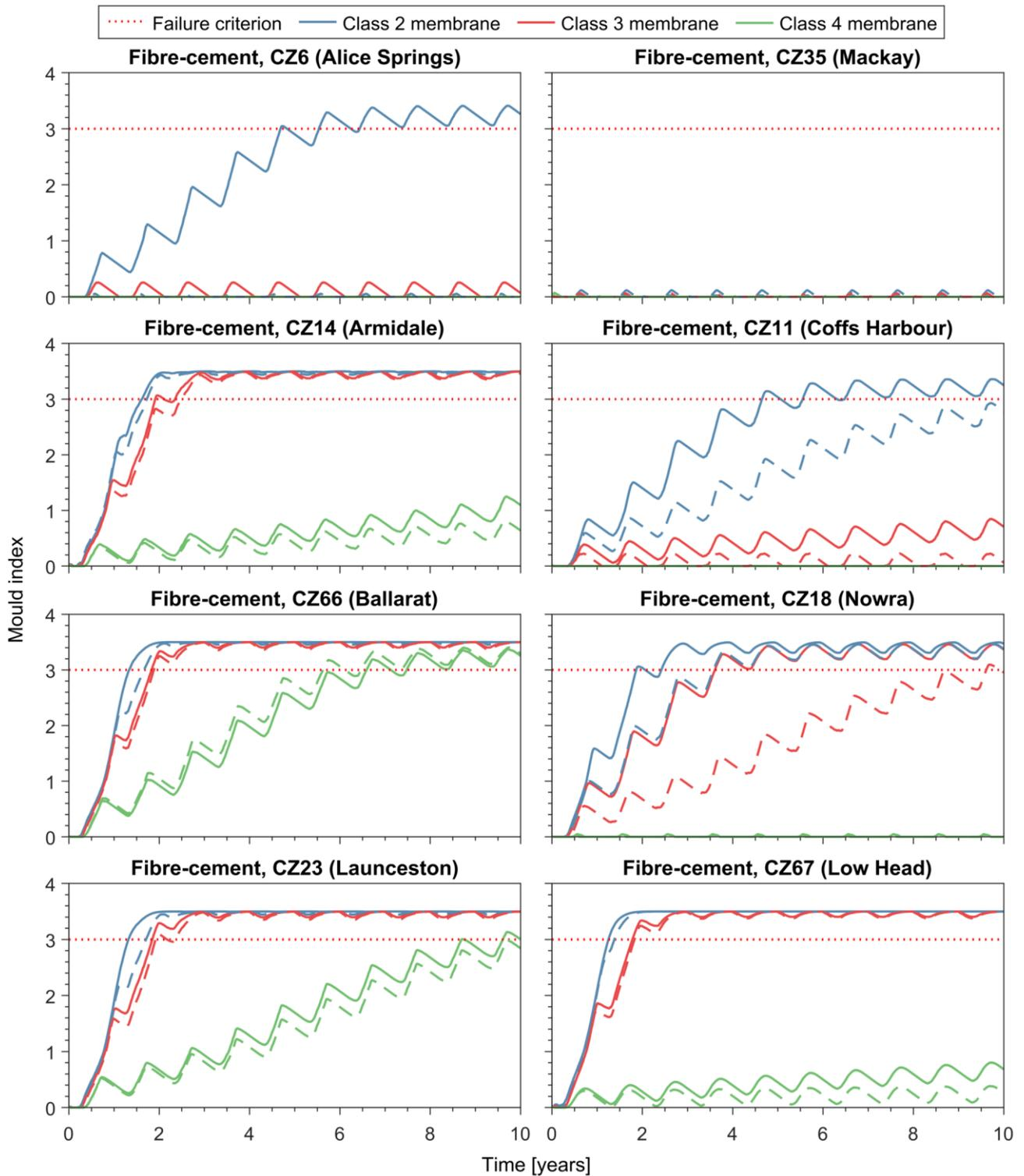
Figure 6-9: Comparison of mould index time series simulated with indoor humidity conditions generated using the standard AIRAH DA07 intermediate method with 70 % relative humidity cap (solid lines), and those generated using the hybrid method (broken lines). Results in this figure are from simulations of the fibre-cement-clad wall with three different membranes in the 8 selected locations.
