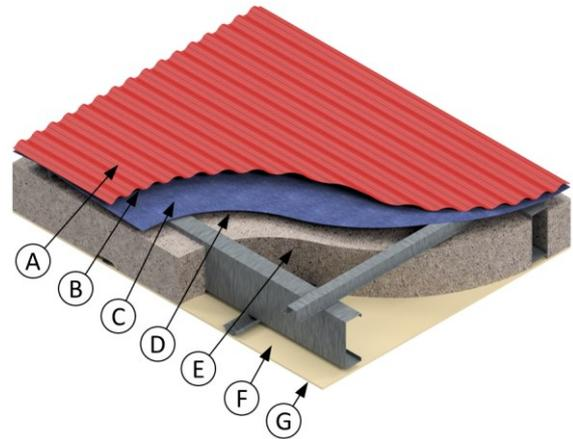
Figure 2-11: Metal-clad roof with cathedral ceiling.
