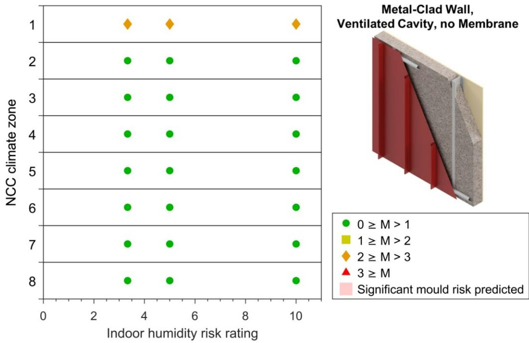
Figure 4-14: Maximum 10-year mould index (M) simulated in metal-clad walls with ventilated cavities and no pliable membrane.
