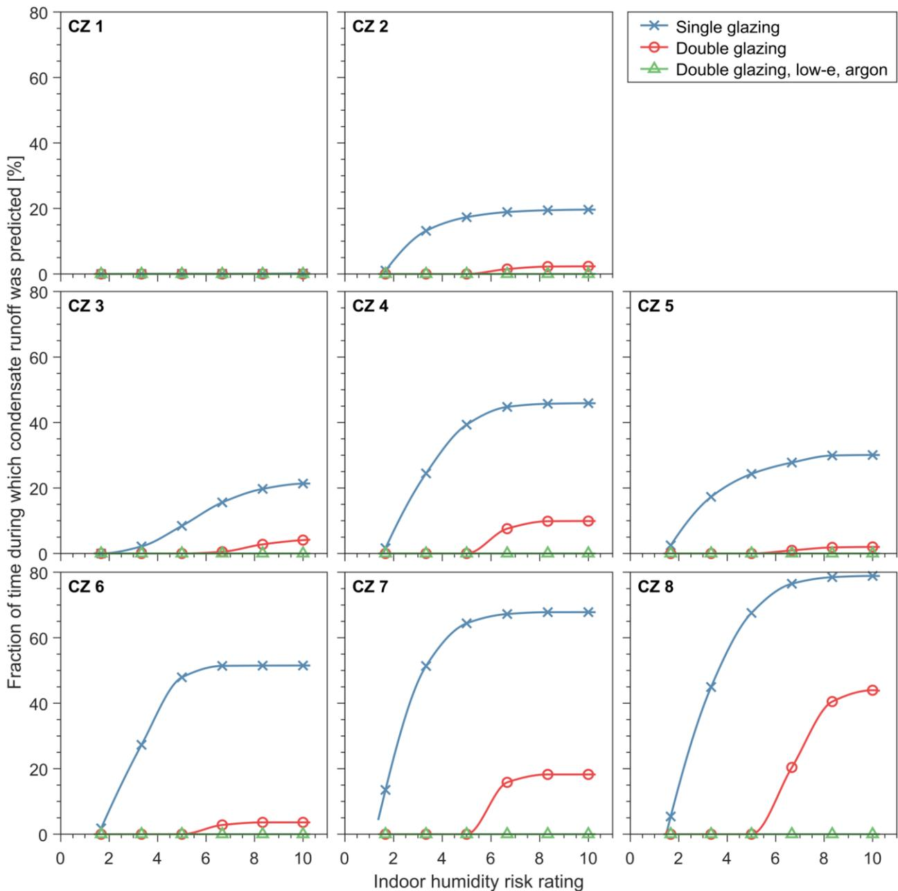
Figure 4-26: Proportion of time during which condensate runoff was predicted to occur on the indoor surface of three glazing systems.
