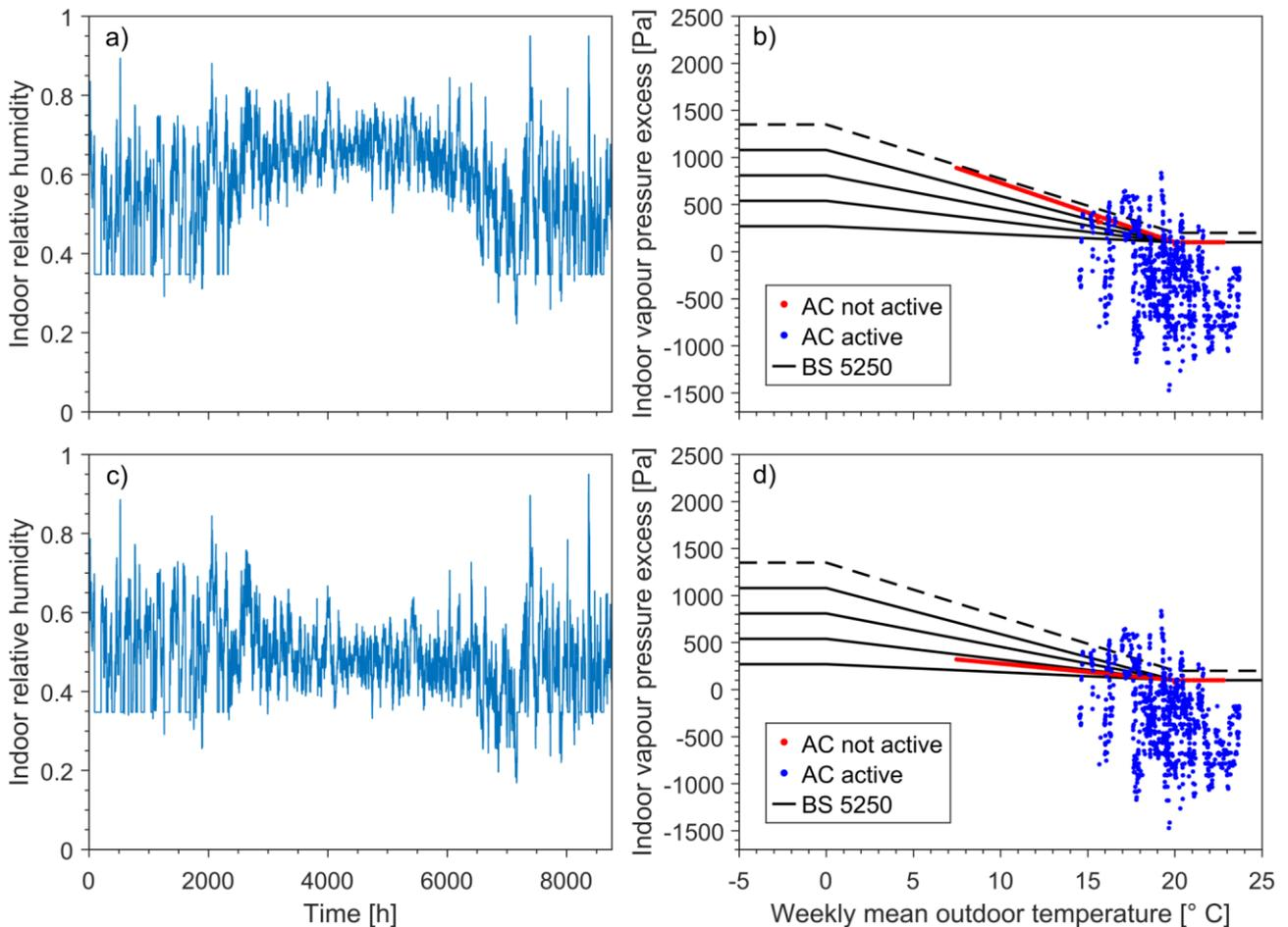
Figure 6-4: Indoor humidity boundary conditions determined for Melbourne following the hybrid method described in this report: a,c) relative humidity time series, b,d) indoor vapour pressure excess at each timestep compared to the indoor climate classes defined in BS 5250. Input assumptions in a and b are the same as in Figure 6-1 and 2; in c and d the infiltration rate has been increased from 0.2 to 0.6 ACH.
