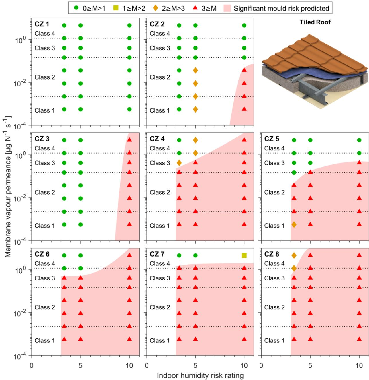
Figure 4-19: Maximum 10-year mould index ( $M$ ) simulated in tiled roofs.
