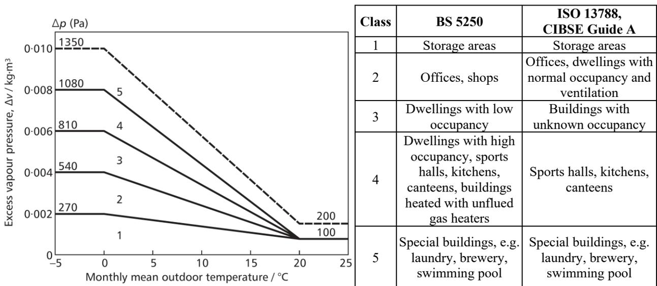
Figure 6-3: Indoor humidity classes, as defined in BS 5250, ISO 13788 and CIBSE Guide A. The graph is reproduced from CIBSE Guide A.
