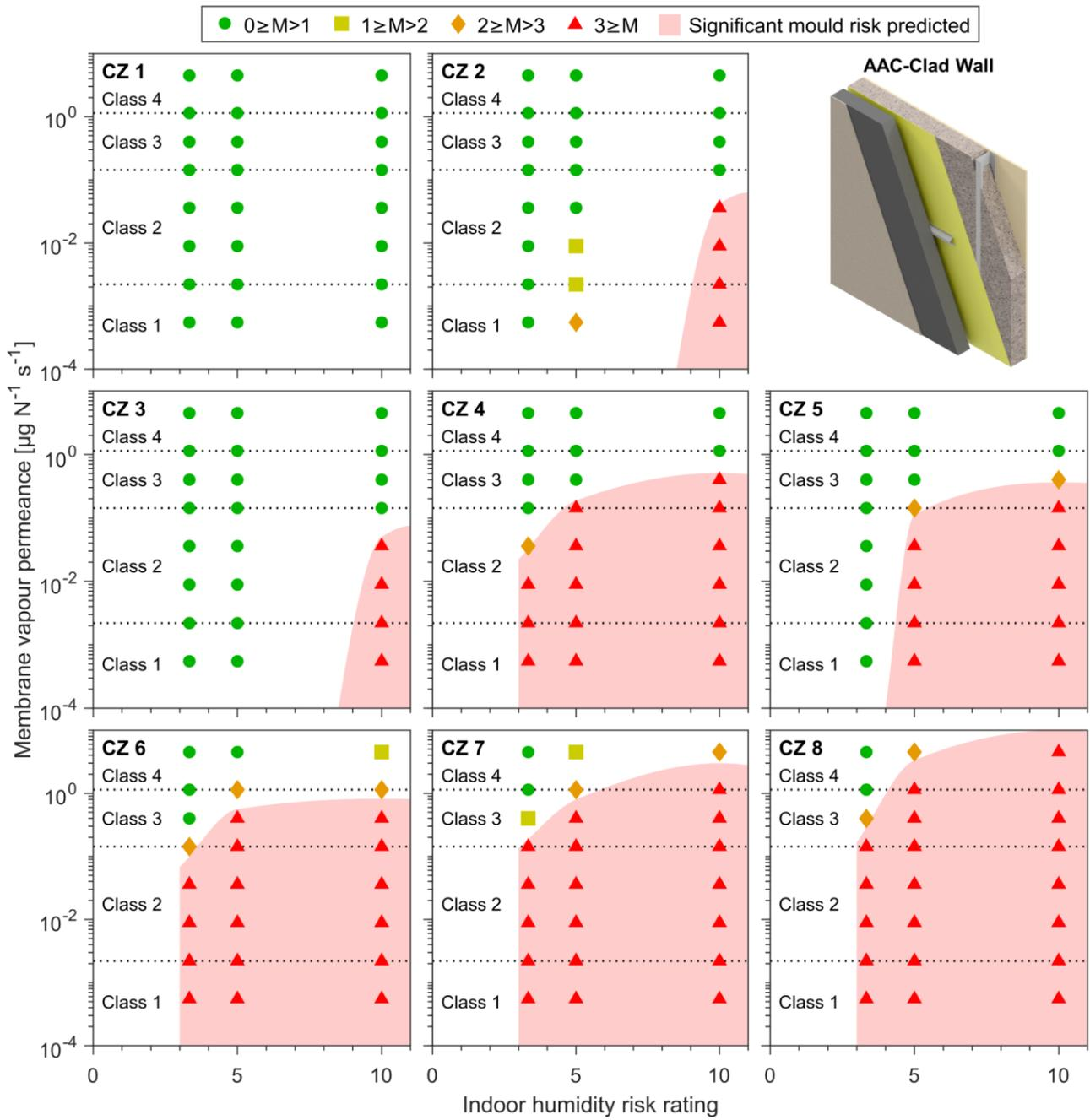
Figure 4-15: Maximum 10-year mould index ( $M$ ) simulated in walls with autoclaved aerated concrete (AAC).
