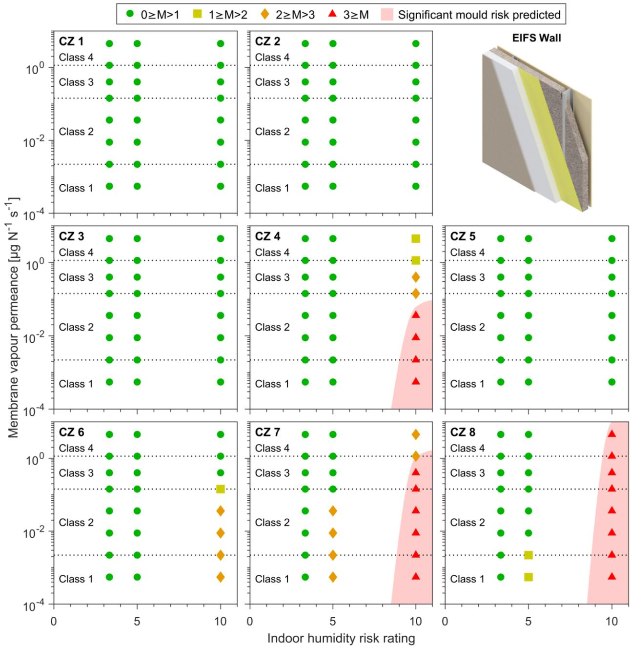
Figure 4-18: Maximum 10-year mould index ( $M$ ) simulated in walls clad with an external insulation finishing system (EIFS).
