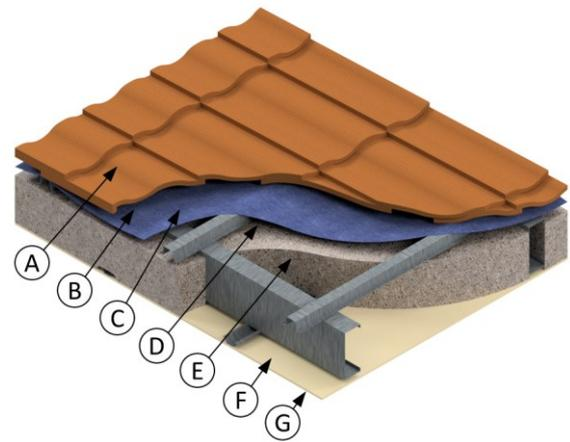
Figure 2-10: Tiled roof with cathedral ceiling.
