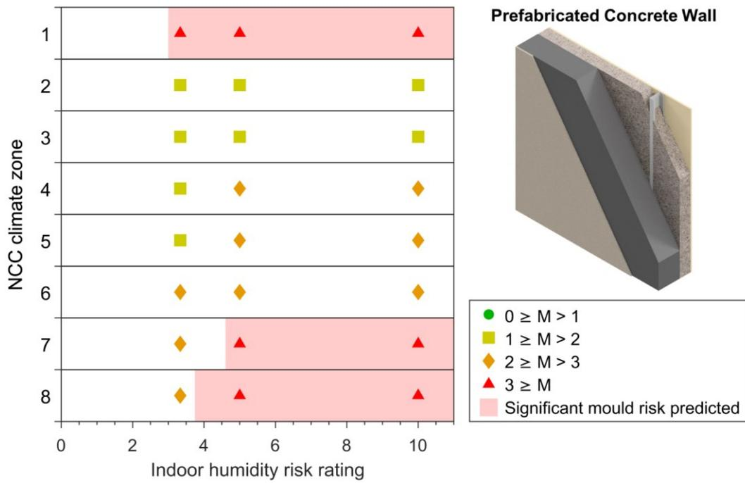
Figure 4-5: Maximum 10-year mould index (M) simulated in prefabricated concrete walls.
