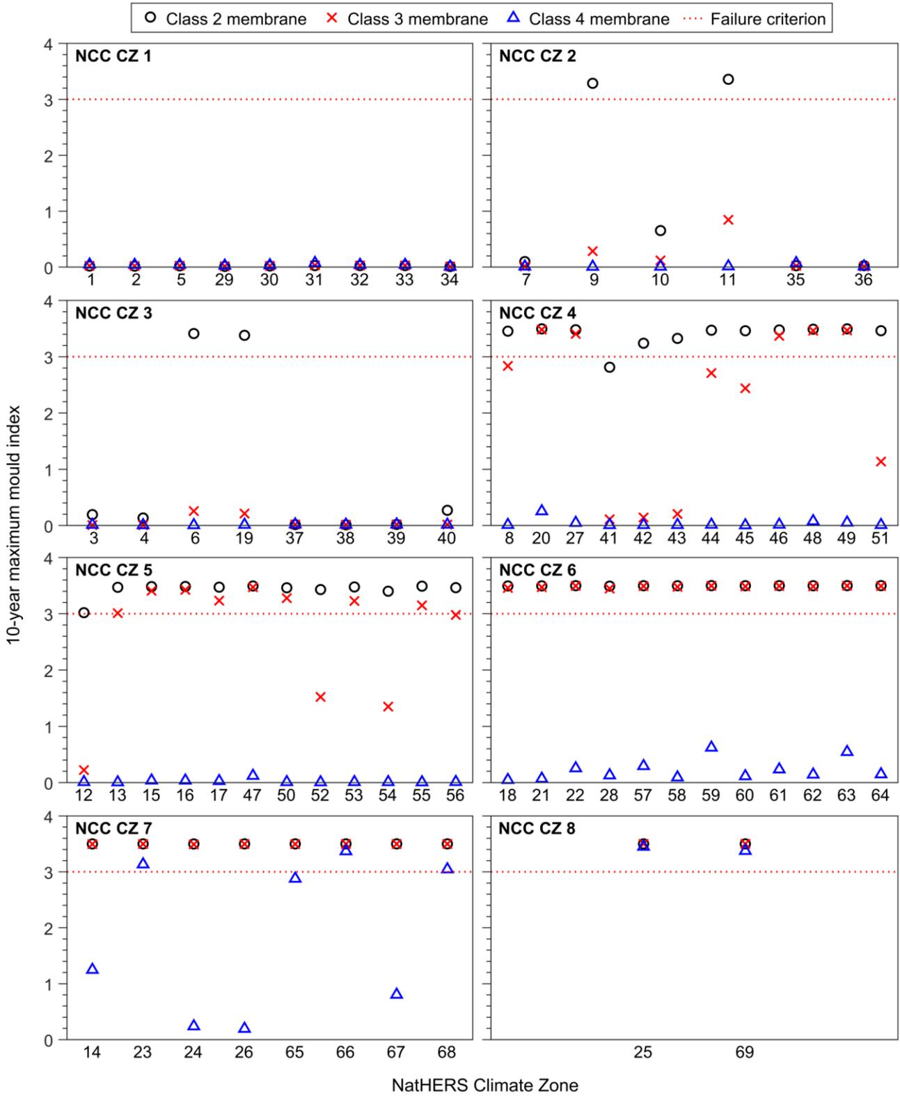
Figure 5-2: Results from WUFI simulations of the fibre-cement-clad wall in all 69 NatHERS climate zones, with three different pliable membranes.
