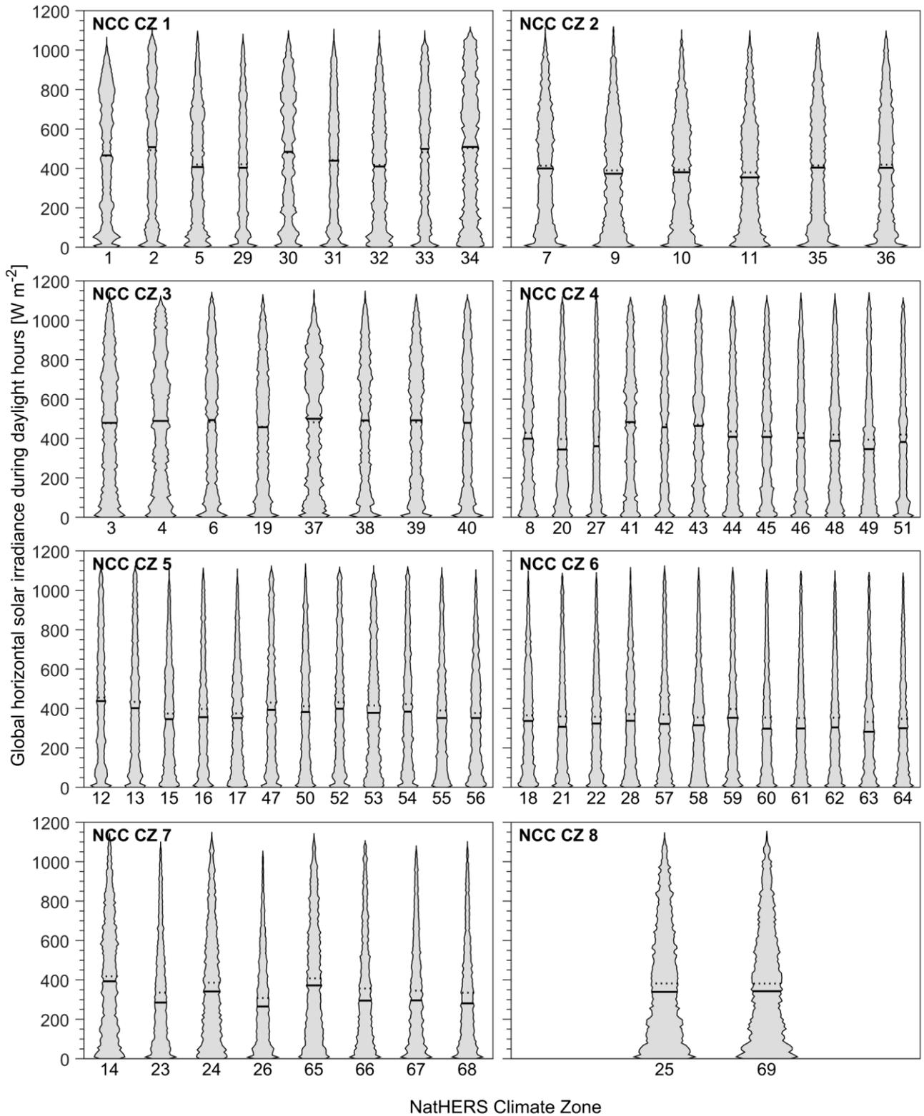
Figure 0-5: Distribution of global horizontal solar irradiance during daylight hours in the climate files used to represent each of the NatHERS Climate Zones.
