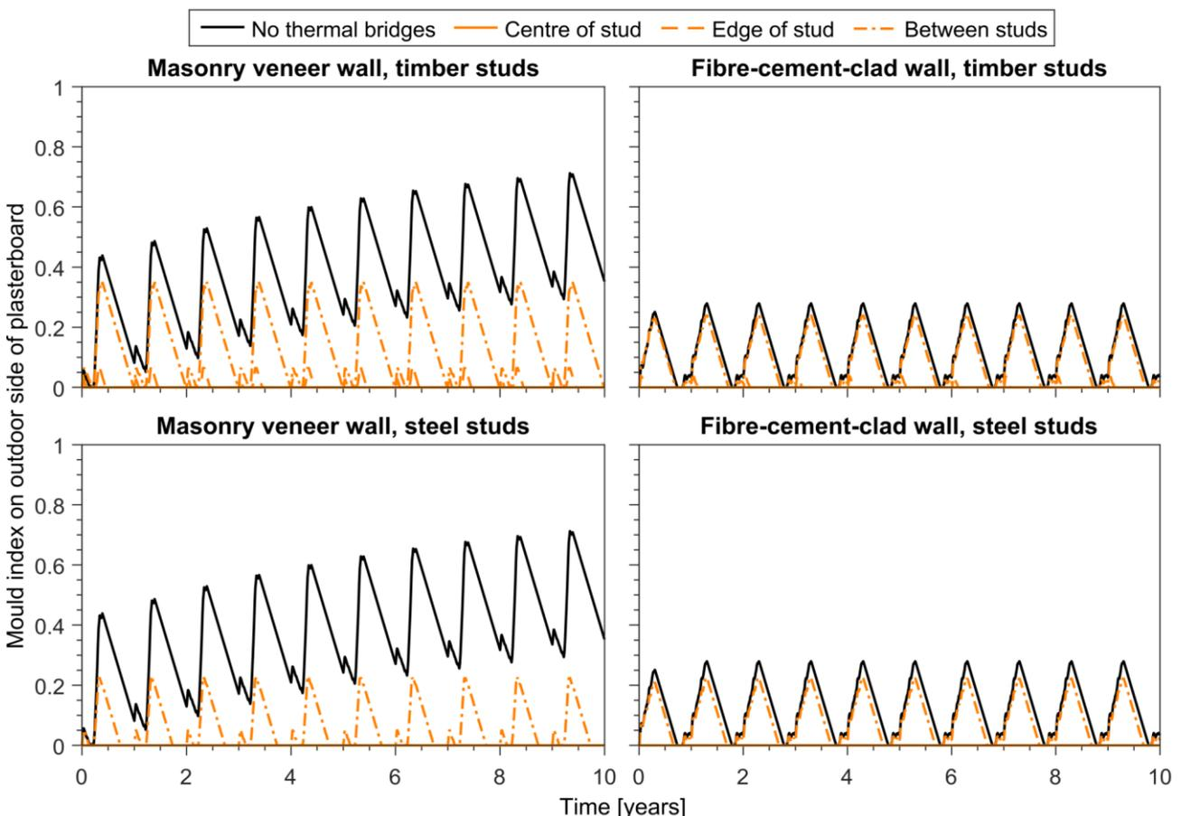
Figure 7-1: Comparison of mould index values simulated in Climate Zone 1 in two-dimensional wall geometries containing no thermal bridges, a timber stud thermal bridge, or a steel stud thermal bridge. These mould index values were simulated near the outdoor-facing surface of the plasterboard.
