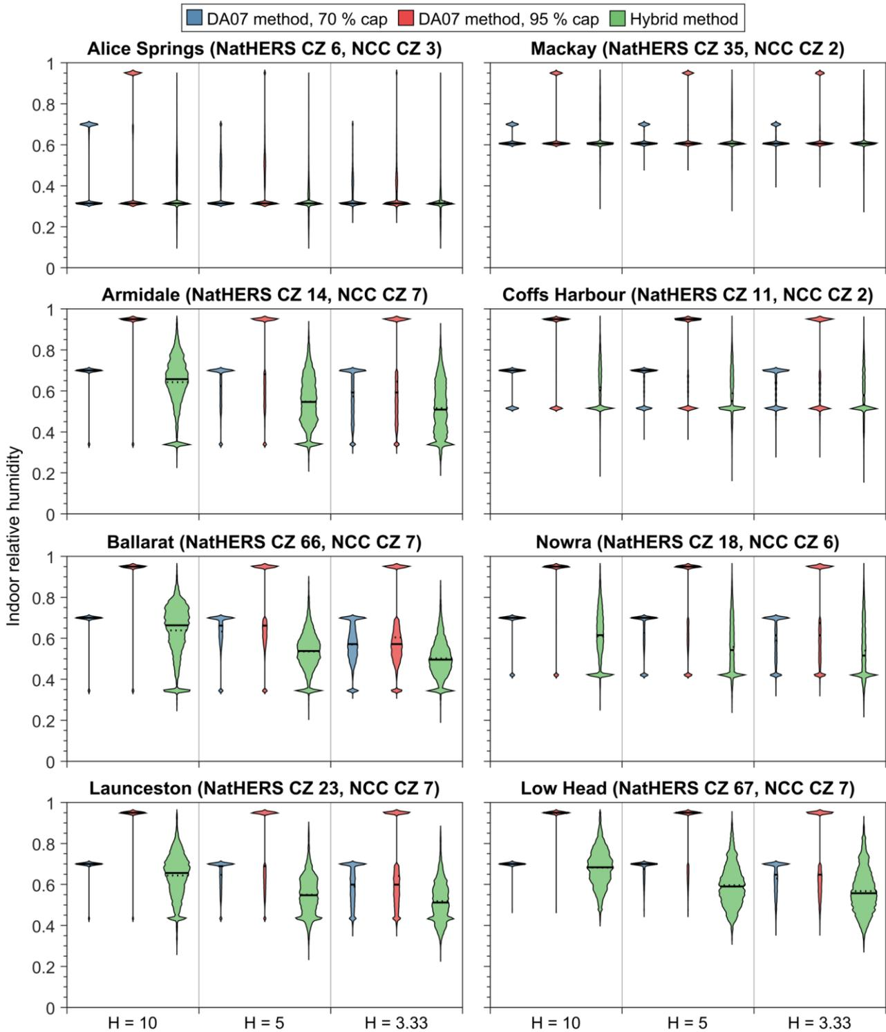
Figure 6-7: Distributions of indoor relative humidity during one year, determined for the 8 selected locations and three Indoor Humidity Risk Ratings ( $H = \{10, 5, 3.33\}$ ), using each of the investigated methods.
