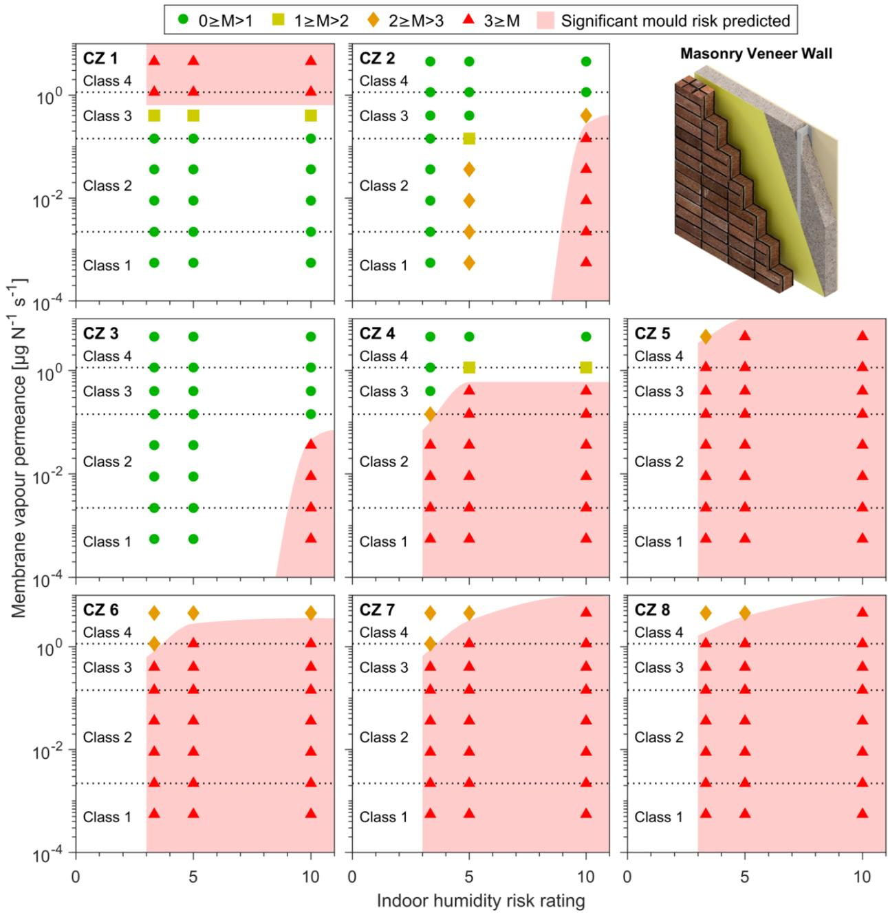
Figure 4-1: Maximum 10-year mould index ( $M$ ) simulated in masonry veneer walls.
