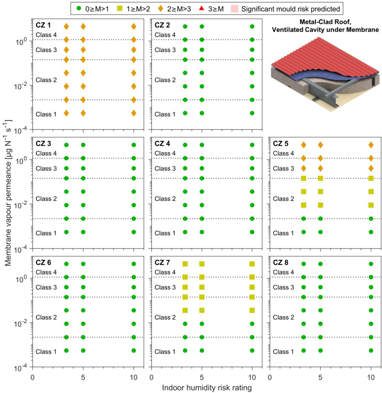
Figure 4-24: Maximum 10-year mould index (M) simulated in metal-clad roofs with ventilation under the membrane.
