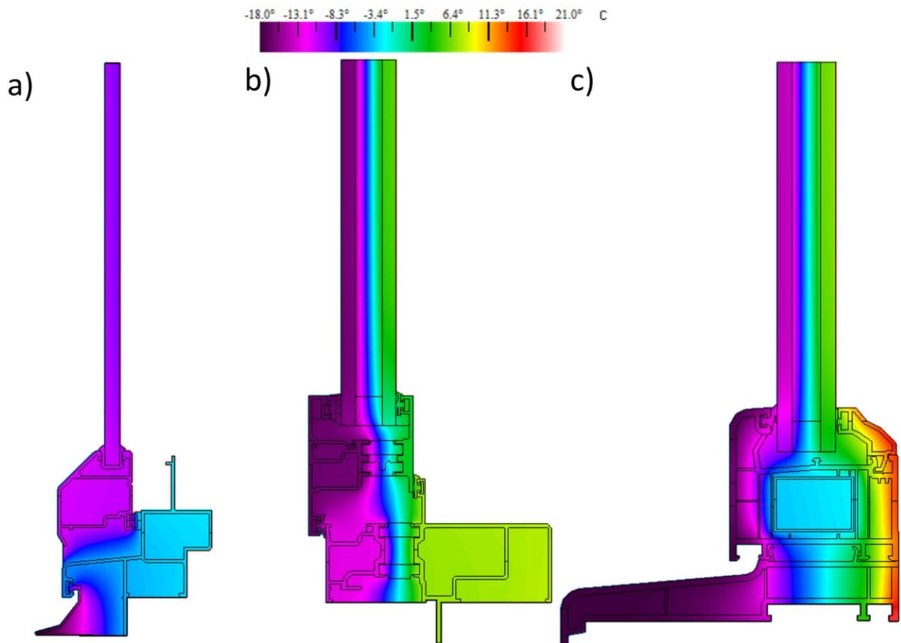
Figure 4-25: Temperature distributions simulated in the three window frames: a) aluminium sill, b) thermally broken aluminium sill, and c) uPVC sill. Images are not drawn to the same scale.
