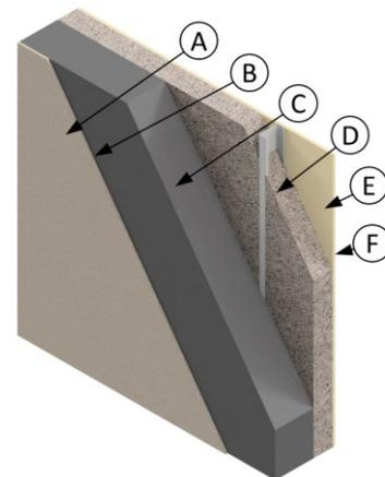
Figure 2-4: Prefabricated Concrete Wall.
