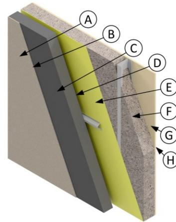
*Figure 2-8: Wall with autoclaved aerated concrete (AAC) cladding.*
