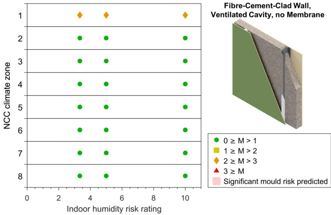
Figure 4-11: Maximum 10-year mould index ( $M$ ) simulated in fibre-cement-clad walls with ventilated cavities and no pliable membrane.
