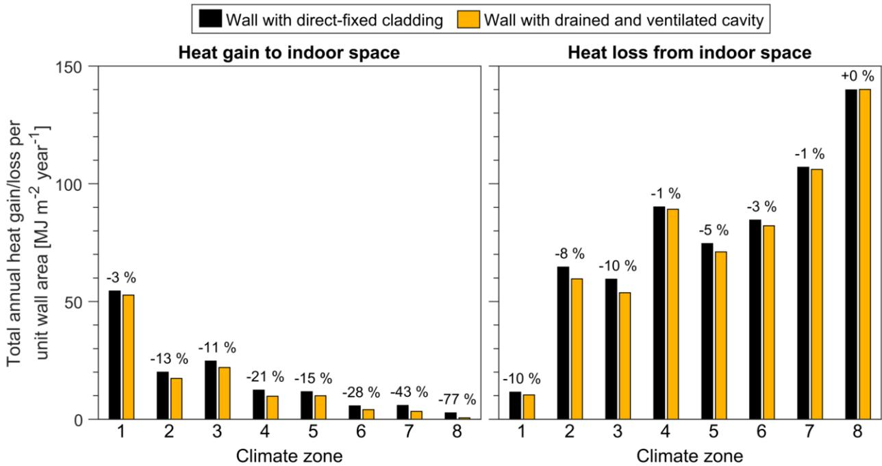
Figure 8-3: Simulated total annual heat gains and losses per unit area through walls with metal cladding and either (i) direct-fixed cladding or (ii) drained and ventilated cavities.
