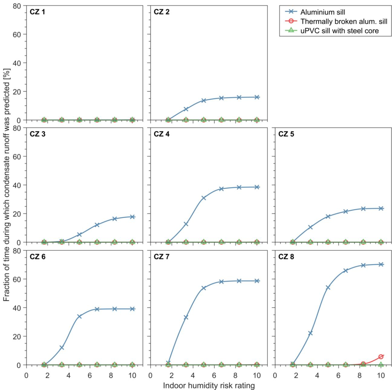
Figure 4-27: Proportion of time during which condensate runoff was predicted to occur on the indoor surface of three window frame components.
