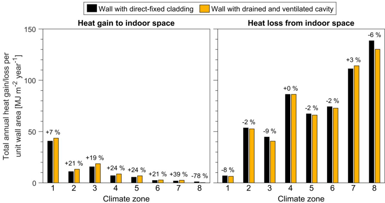
Figure 8-4: Simulated total annual heat gains and losses per unit area through walls with AAC cladding and either (i) direct-fixed cladding or (ii) drained and ventilated cavities.
