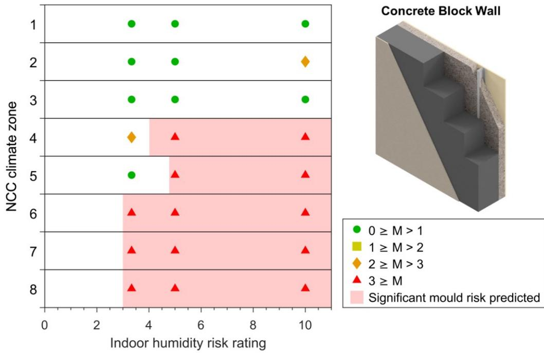
Figure 4-4: Maximum 10-year mould index (M) simulated in concrete block walls.
