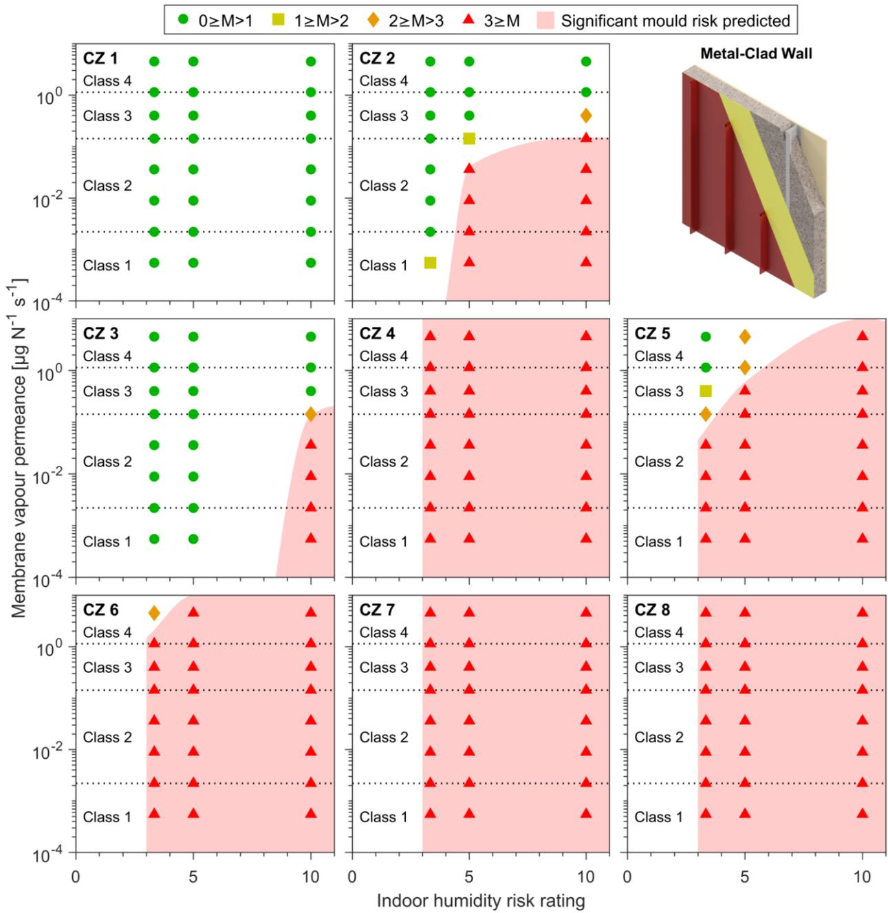
Figure 4-12: Maximum 10-year mould index ( $M$ ) simulated in metal-clad walls.
