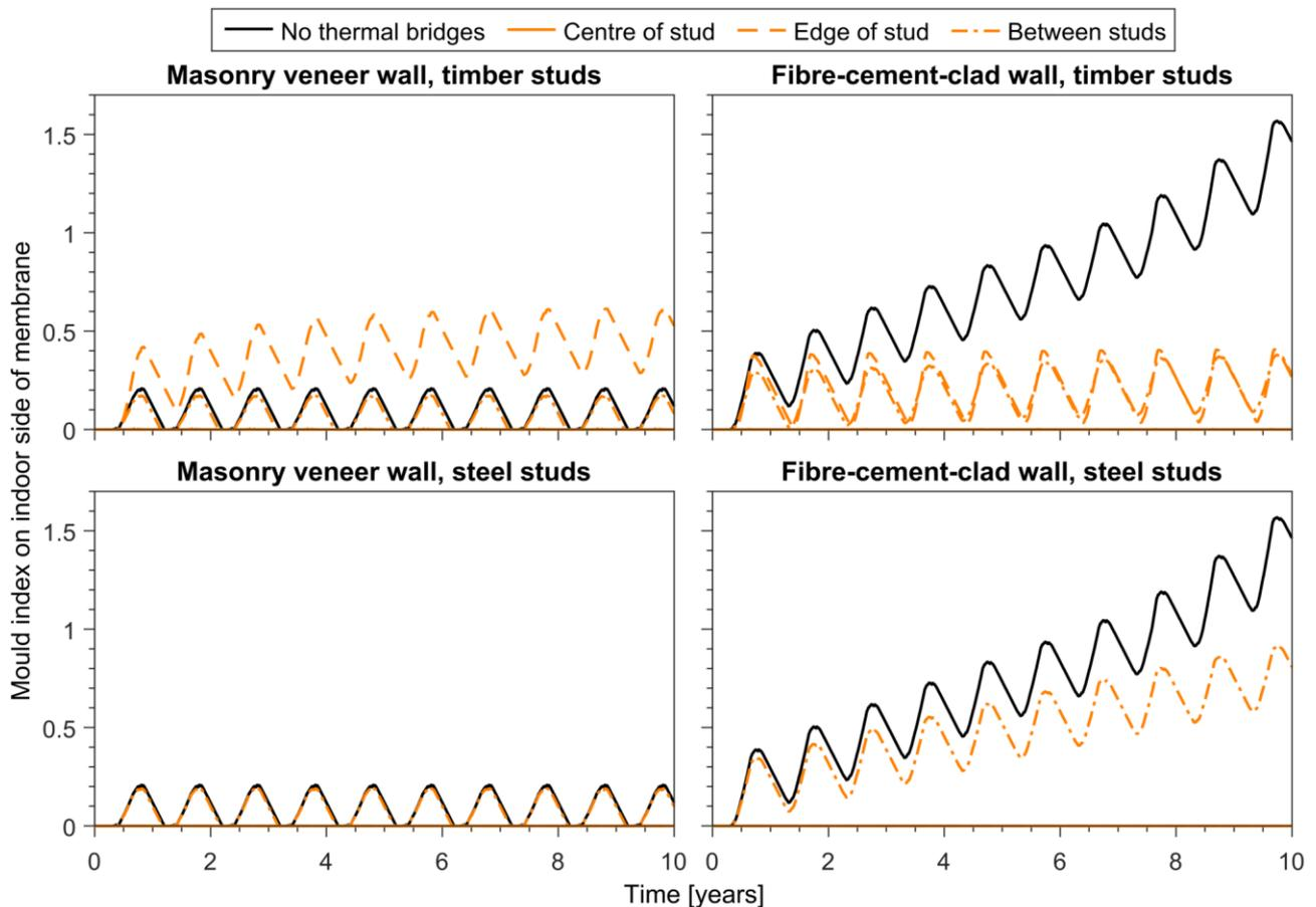
Figure 7-2: Comparison of mould index values simulated in Climate Zone 7 in two-dimensional wall geometries containing no thermal bridges, a timber stud thermal bridge, or a steel stud thermal bridge. These mould index values were simulated near the indoor-facing surface of the membrane.
