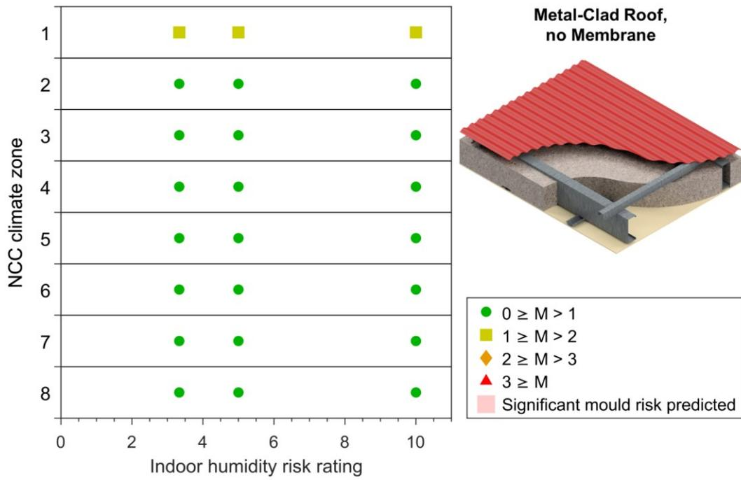
Figure 4-23: Maximum 10-year mould index (M) simulated in metal-clad roofs with no membrane.
