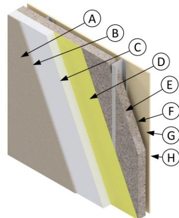
*Figure 2-9: Wall with external insulation finishing system (EIFS).*
