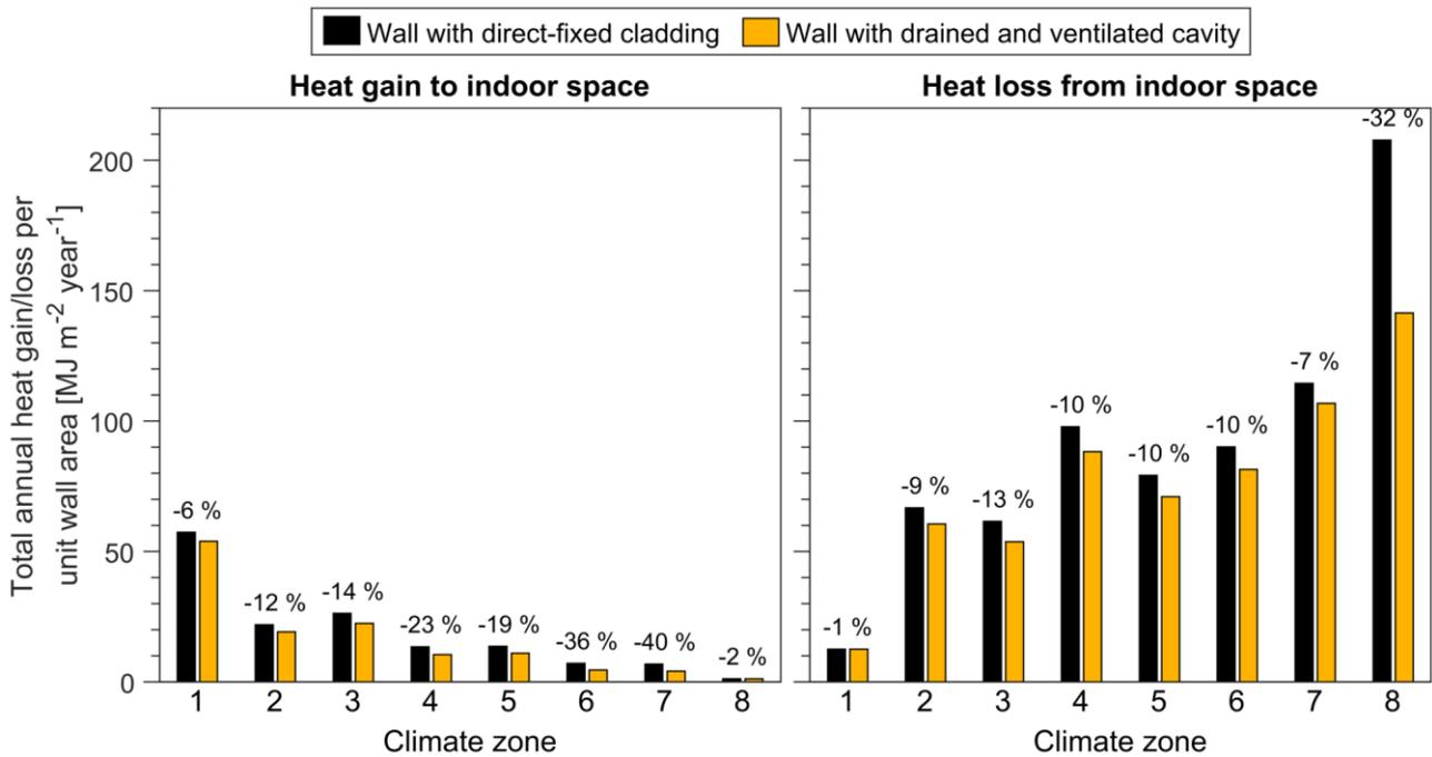
Figure 8-2: Simulated total annual heat gains and losses per unit area through walls with fibre-cement cladding and either (i) direct-fixed cladding or (ii) drained and ventilated cavities.
