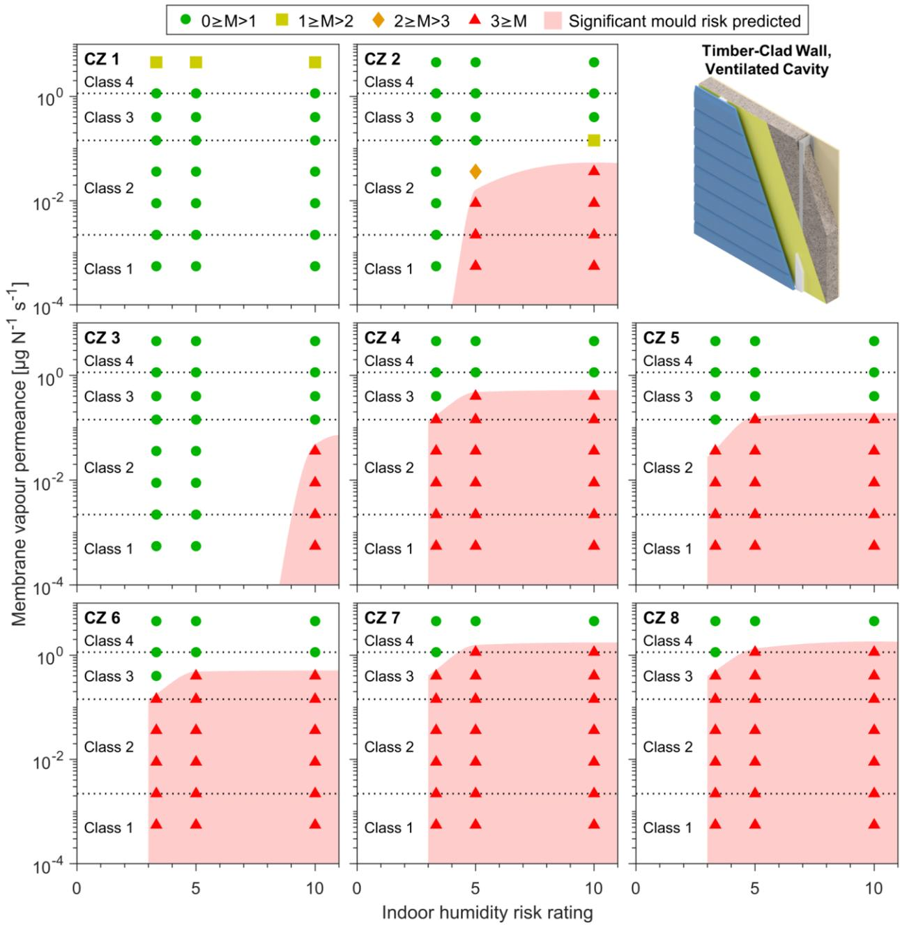
Figure 4-7: Maximum 10-year mould index ( $M$ ) simulated in timber-clad walls with ventilated cavities.
