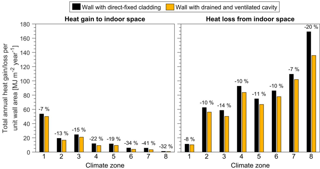
Figure 8-1: Simulated total annual heat gains and losses per unit area through walls with timber cladding and either (i) direct-fixed cladding or (ii) drained and ventilated cavities.
