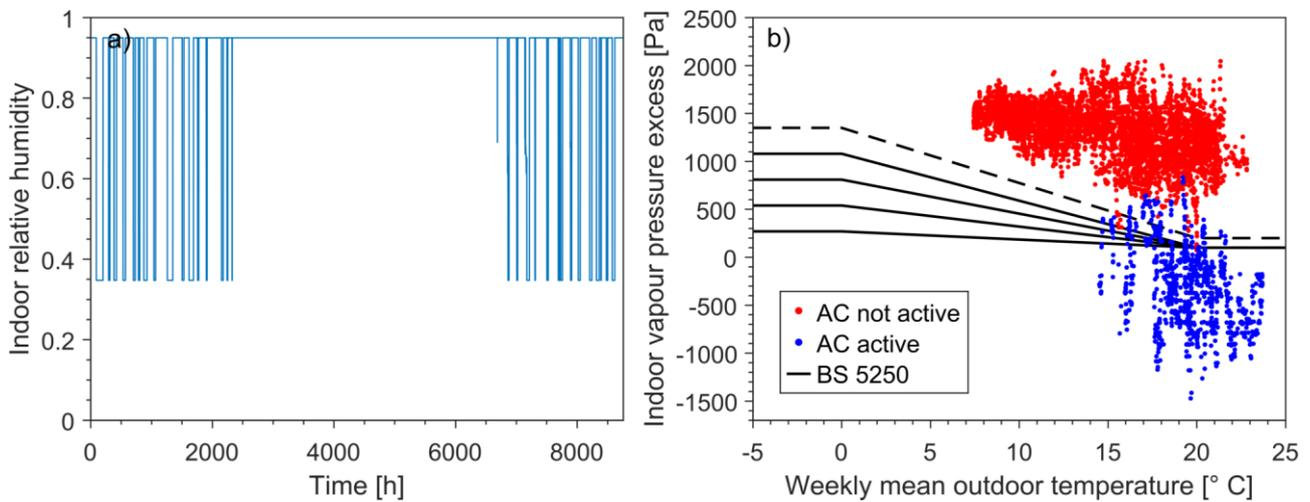
Figure 6-2: Indoor humidity boundary conditions determined for Melbourne following the AIRAH DA07 intermediate method with a 95 % relative humidity cap. Input assumptions are the same as in Figure 6-1.
