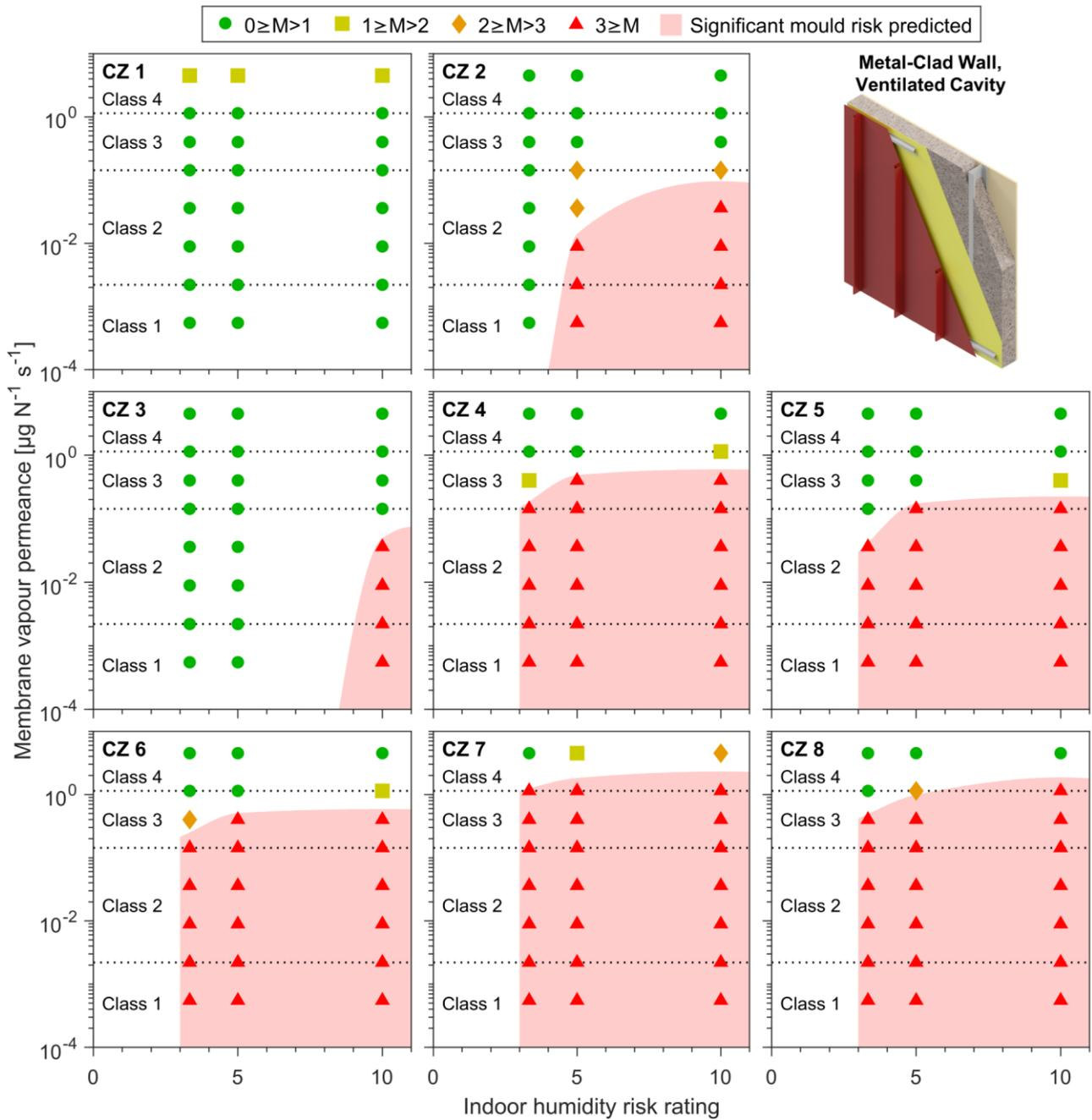
Figure 4-13: Maximum 10-year mould index ( $M$ ) simulated in metal-clad walls with ventilated cavities.
