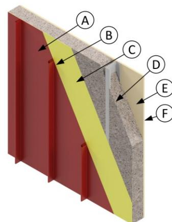
Figure 2-7: Metal-clad wall.
