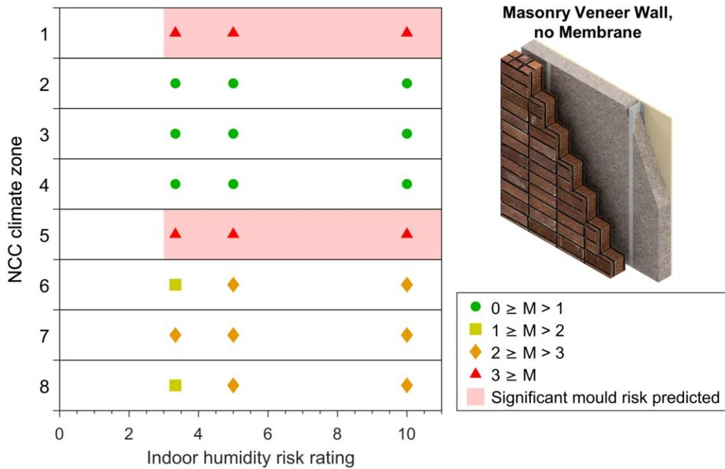
Figure 4-2: Maximum 10-year mould index ( $M$ ) simulated in masonry veneer walls with no membrane.
