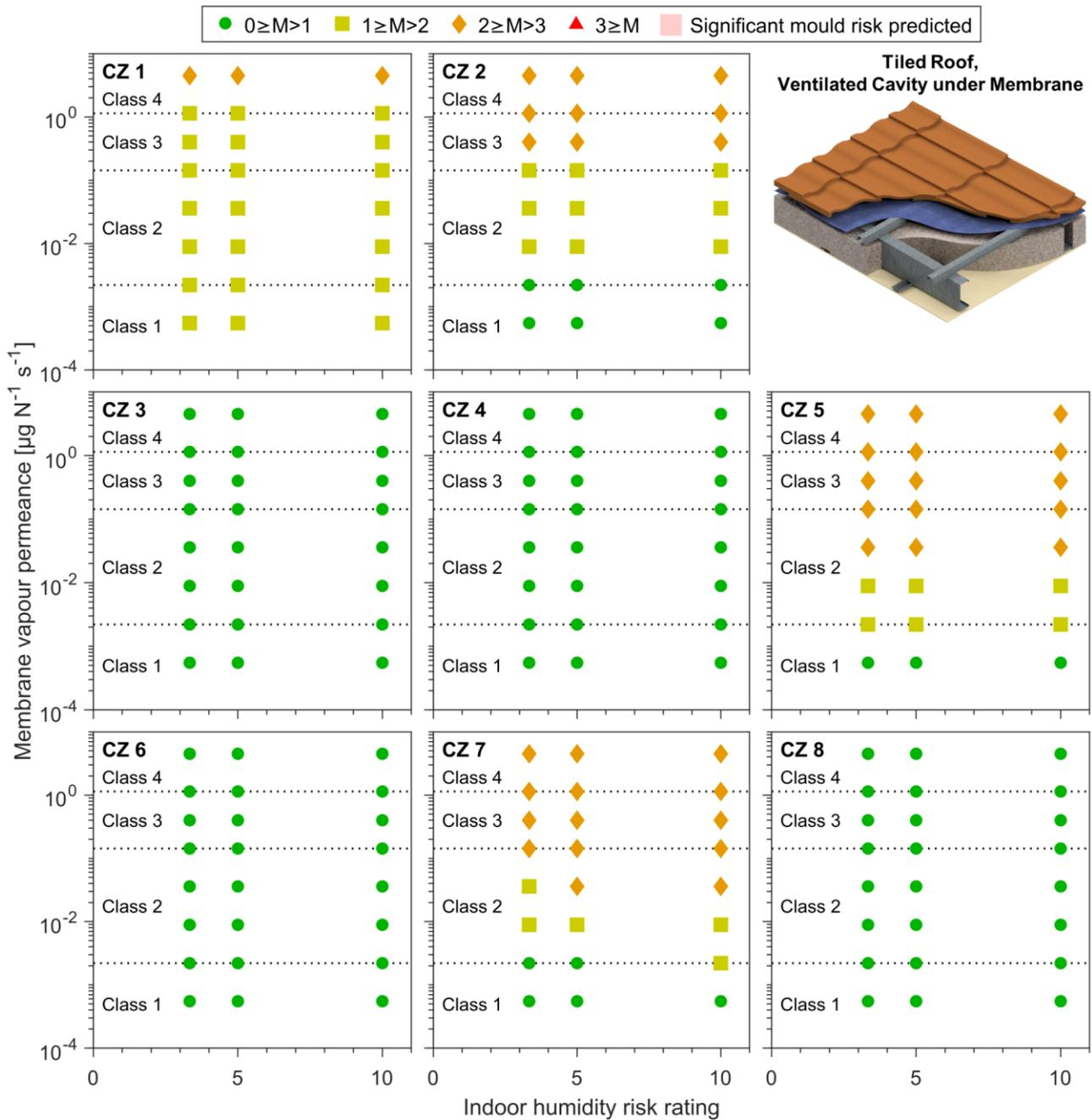
Figure 4-21: Maximum 10-year mould index (M) simulated in tiled roofs with ventilation under the membrane.
