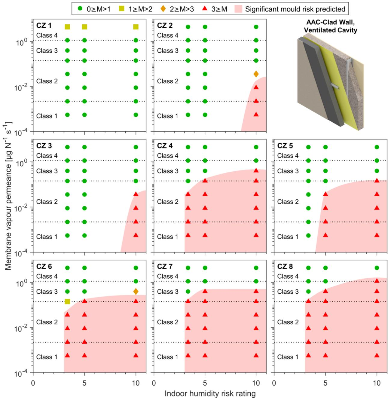
Figure 4-16: Maximum 10-year mould index ( $M$ ) simulated in walls clad with autoclaved aerated concrete (AAC), with ventilated cavities.
