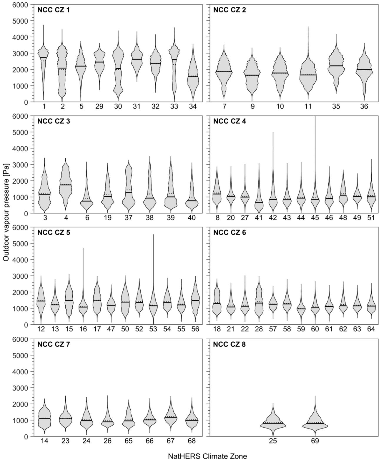
Figure 0-3: Distribution of outdoor vapour pressure in the climate files used to represent each of the NatHERS Climate Zones.
