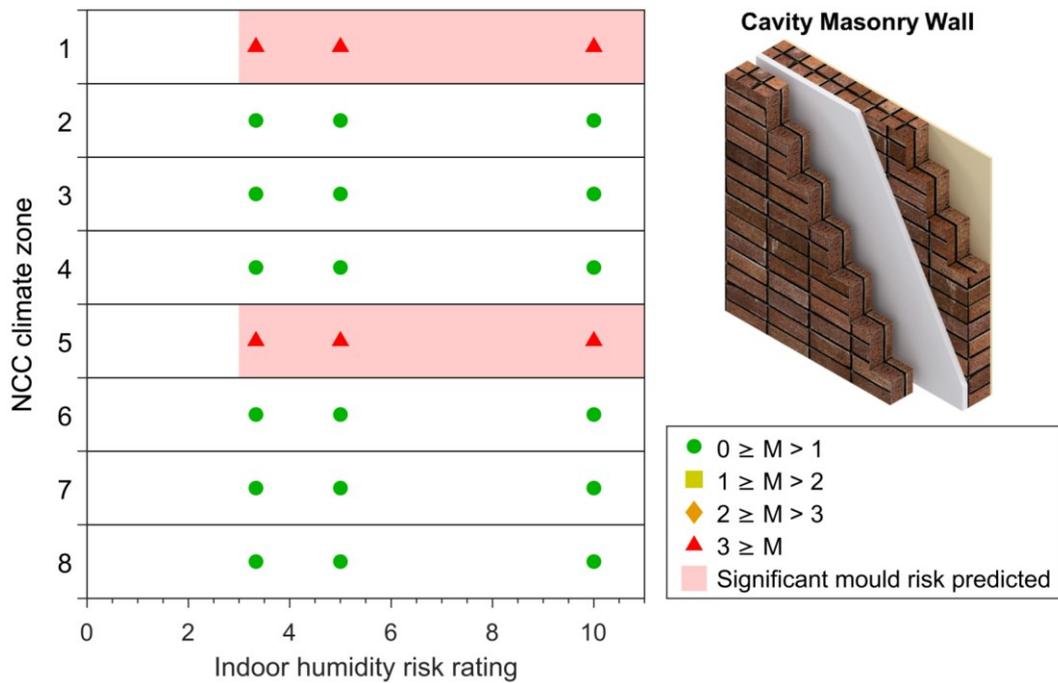
Figure 4-3: Maximum 10-year mould index ( $M$ ) simulated in cavity masonry walls.
