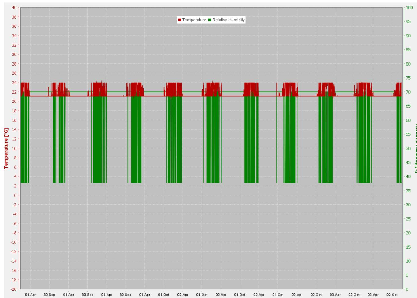
Figure 22. Internal climate condition input. The data is dependent on the external climate data where the mechanical units would be assumed to be operating when heating or cooling is required for its set points. Set point for heating is 21.1°C whilst set point for cooling is 23.9°C as per Table 4.2 in AIRAH DA07, 24/7.
