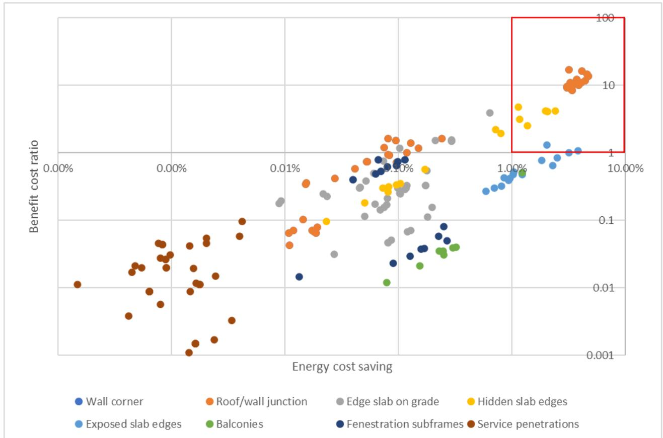
Figure 53. Collation of UoW cost/benefit analyses for various thermal bridge mitigations across a range of archetype building and climate zones. The red box indicates the measures that were both cost beneficial (BCR>1) and significant (impact>1%)
