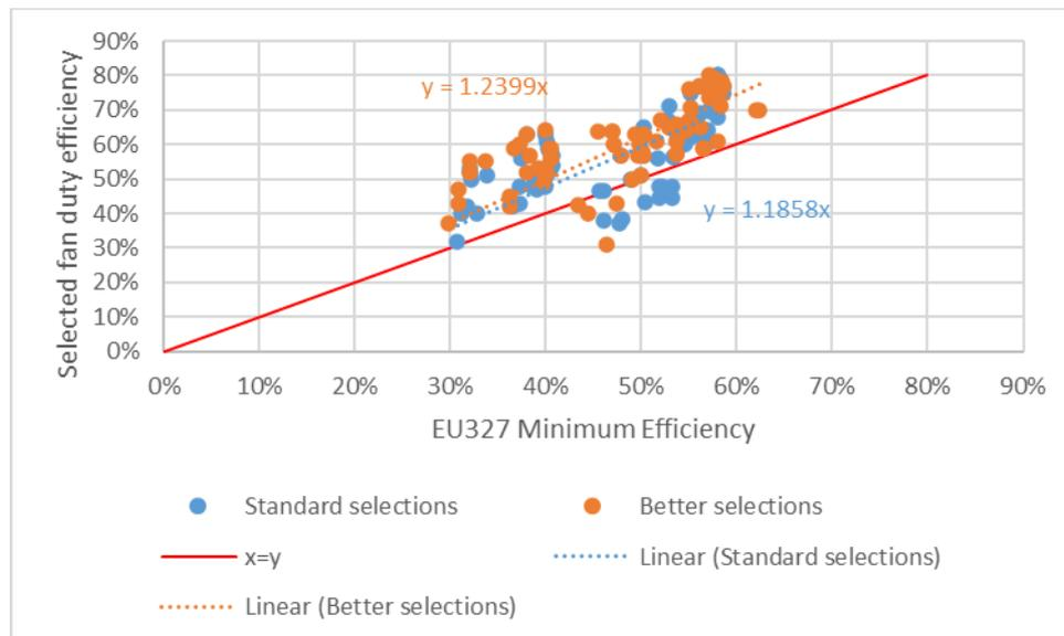
Figure 107. Comparison of selected and minimum efficiency figures for real fan selections
