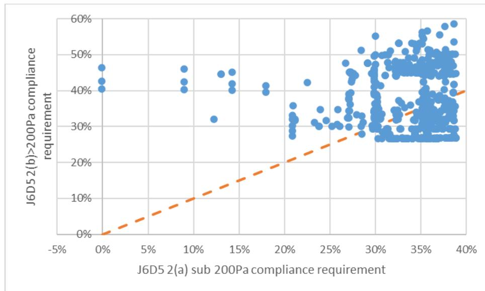
Figure 104. Comparison of compliance requirements for J6D5 2(a) (sub 200Pa) versus the equivalent J6D5 2(b) requirement.
