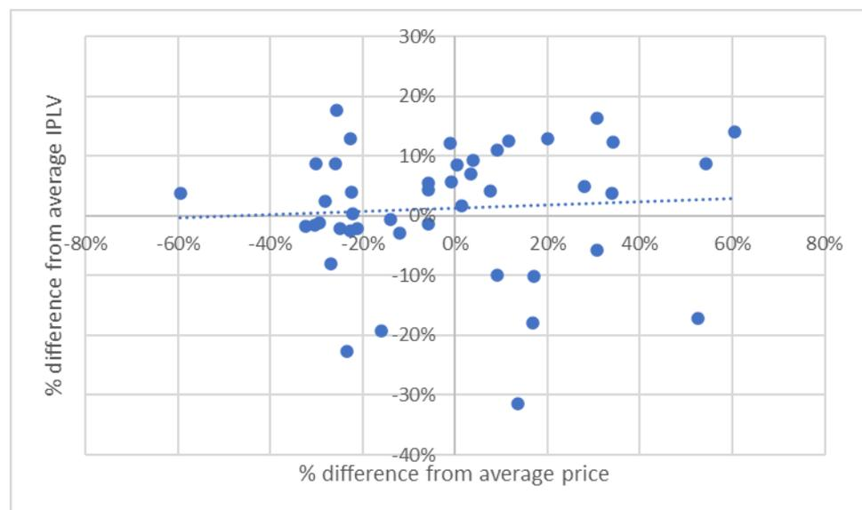
Figure 10. Percentage difference in IPLV versus percentage cost difference for air-cooled chillers; cost figures have been corrected for capacity, average IPLV was calculated to be 5.114 at all capacities.
