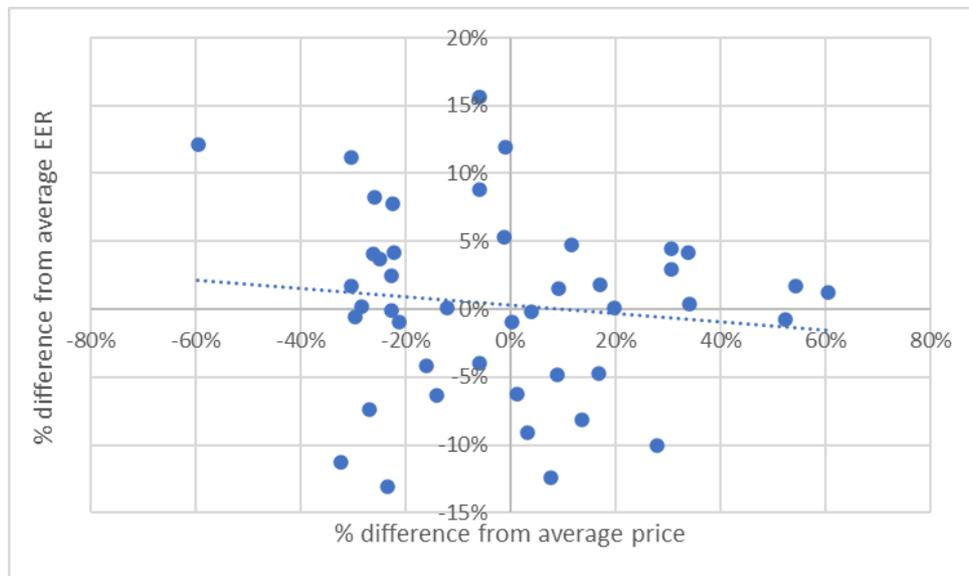
Figure 9. Percentage difference in EER versus percentage cost difference for air-cooled chillers; cost figures have been corrected for capacity, average EER was calculated to be 3.114 at all capacities.
